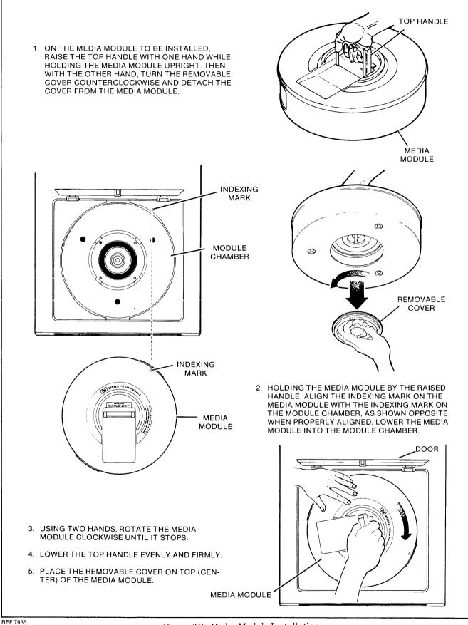
Figure 3-2. Media Module Installation
