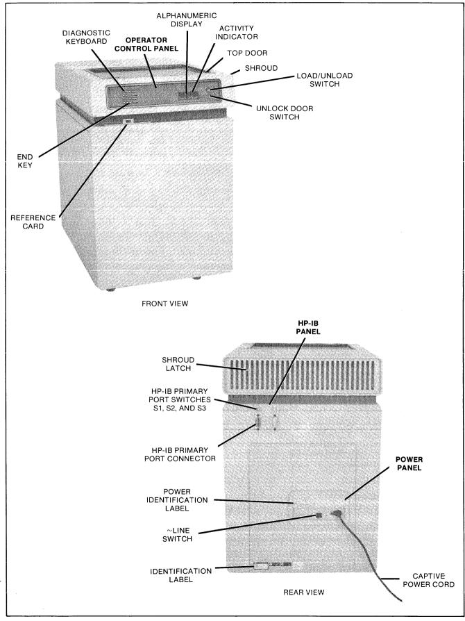
Figure 3-1. Switches, Indicators, and Connectors
