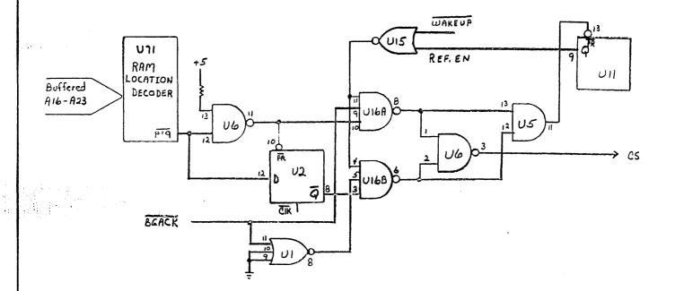
If RAM is being refreshed, the Ref.en input to U15 is high. The output of U15 is low inhibiting both gates of U16. This causes CS to remain low. When the refresh is complete, Ref.en is negated. The output of U15 then enables both gates of U16.
