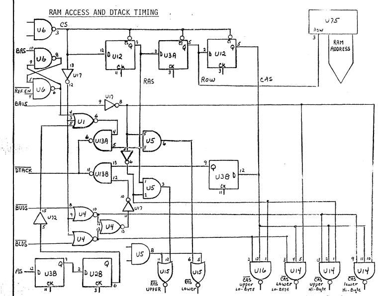
A normal CPU access of RAM is a 5 cycle access. However, if Refresh occurs during the access, time must be allowed for the refresh before the transfer of data can occur. This is accomplished by controlling the time at which DTACK occurs. During a normal access, ENDT is gated to provide DTACK. When RAM is accessed during a refresh cycle, ENDT is ignored, and since CAS won't occur until after refresh, it is gated to provide DTACK.
