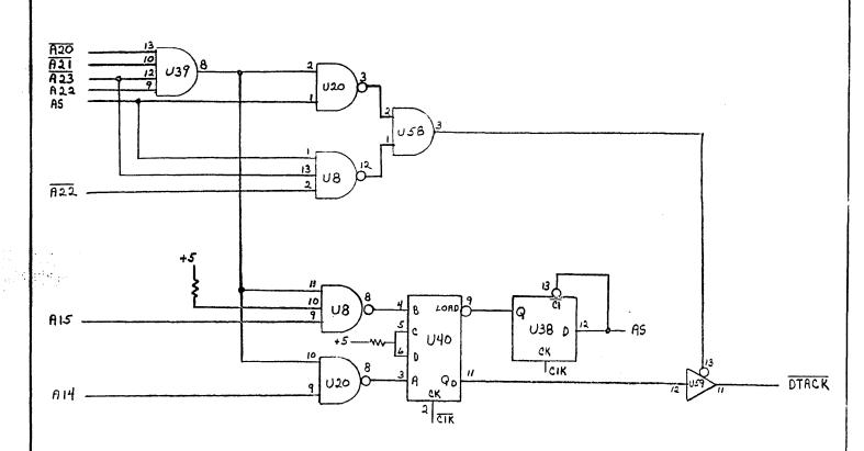
DTACK signals the CPU that a transfer is complete. Auto DTACK is generated on the CPU board and is used to supply the DTACK for the ROM address space and for internal synchronous I/O devices.
