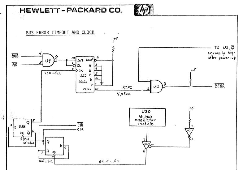
DTACK signals the processor that a data transfer is complete so that the CPU can terminate the cycle. BERR tells the CPU that DTACK has not occured during a pre-determined amount of time and it should initiate an exception processing cycle.
