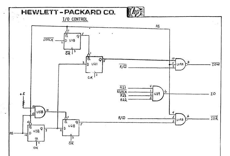
The two control signals  $\overline{IOW}$  and  $\overline{IOR}$  are used as control signals for Intel compatable peripheral chips. The signal IO is used to aid in internal chip select decoding.
