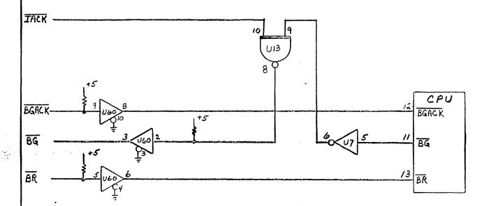
An external device capable of controlling the bus requests the bus by asserting  $\overline{BR}$  (Bus Request). When the processor sees  $\overline{BR}$ , it asserts  $\overline{BG}$  indicating that it will release bus control at the end of the current bus cycle.
