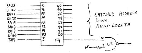
The outputs of the RAM Auto Locate circuit (U61) are tied to Q inputs of comparator U71. When the address on BA16 through BA23 matches the latched address from Auto Locate and when U71 is enabled by  $\overline{\text{BAS}}$ , the output of U71 is asserted. If Ram is not being refreshed this output is gated to become chip select.
