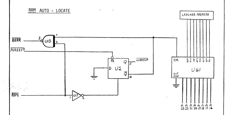
The on beard RAM locates itself at the bottom of RAM memory. This auto-locate feature eliminates the need for user set switches on an internal board.
