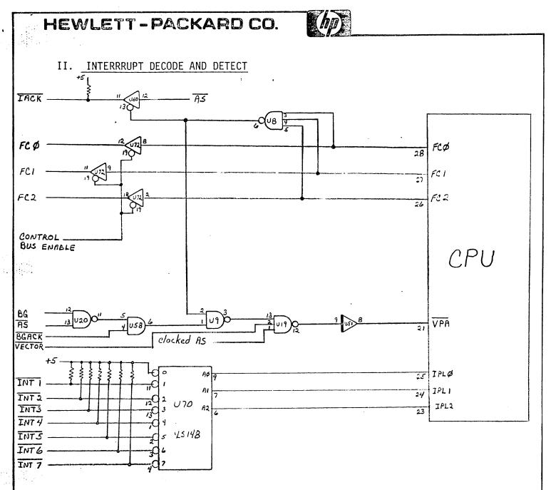
Seven levels of interrupt are decoded into a 3 line binary by U70. Interrupt level 7 is the highest priority, level 0 is no interrupt. Internal circuitry in the CPU inhibits all interrrupts with priority levels less than or equal to the current processor priority.
