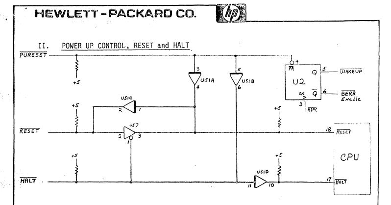
During power-up,  $\overrightarrow{PURESET}$  is asserted by the power supply board. This asserts RESET and HALT to the system bus and the processor through U5, A + B + C and presets U2.  $\overrightarrow{WAKEUP}$  from U2 is negated, inhibiting chip select (See RAM Access section).  $\overrightarrow{BERR}$  Enable is negated allowing suppression of the first  $\overrightarrow{BERR}$ . (See RAM Auto Locate section). After voltages stabilize,  $\overrightarrow{PURESET}$  is negated.
