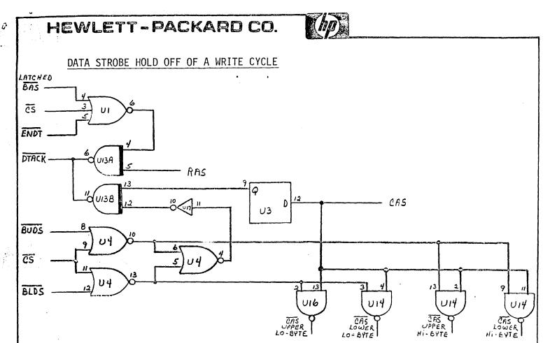
During a DMA write to RAM, the amount of time necessary to set up data to RAM is unknown. Because of this the DMA controller starts the RAM access by placing the RAM address on the bus and asserting  $\overline{\text{BAS}}$ . While data is being set up, the DMA controller holds off the data strobes until data is valid.  $\overline{\text{ENDT}}$  is inhibited because the control bus is tristated when the CPU gives up control, so U13A (EDTACK) is inhibited.
