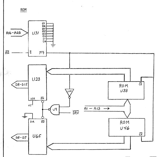
U31 decodes a low on A16 through A23 to enable  $\overline{CE}$  to ROM.  $\overline{DRV}$  is normally high so  $\overline{p=q}$  is gated through U9 to enable the data buffer U23 and U65. Data at the location addressed by the address bus is transferred through the buffers onto the processor data bus.
