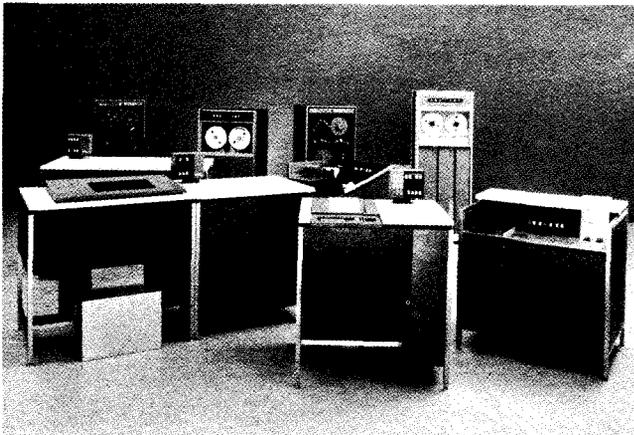
The array of peripheral devices available with Series 200 processors includes over 40 units: punched card equipment, high-speed printers, magnetic tape units, paper tape equipment, magnetic tape strip mass memory units, random access drum units, and various data communication equipment. Also included are computer-to-computer adapters, an interval timer, a time of day clock, MICR reader/sorter controls, and peripheral switching units which provide extremely flexible Series 200 configurations.
