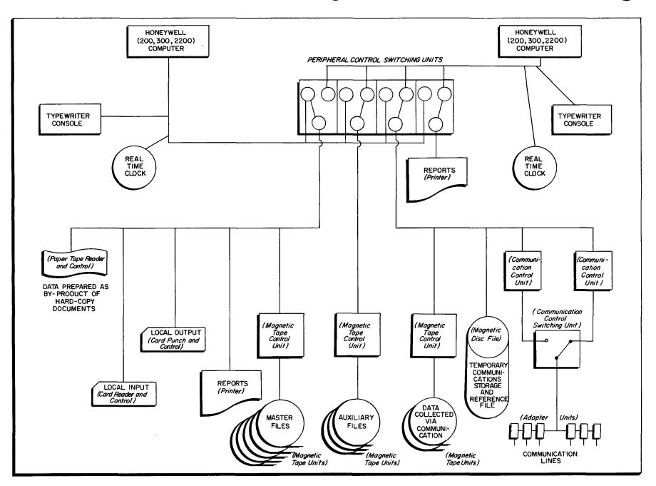
A Typical Integrated System Using Honeywell Switching Units
