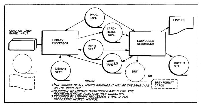
Figure 1-3. Integrated System of Library Processor and Easycoder Assembler
