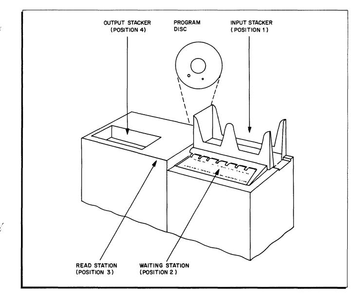
Figure 5-4. Punched Card Reader Sequence of Operation (Cover Removed)
