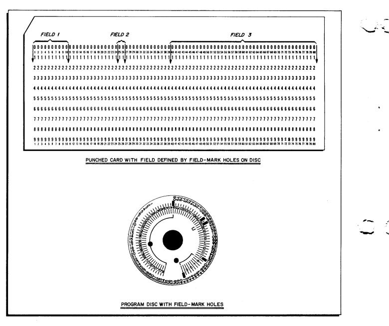
Figure 5-5. Field-Mark Orientation
