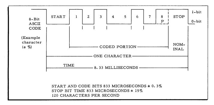
Figure 3-1. Data Station Code Character Over Common Carrier Medium Under Ideal Conditions
