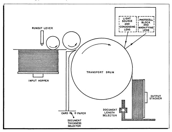
Figure 5-7. Optical Bar Code Reader Schematic Diagram
