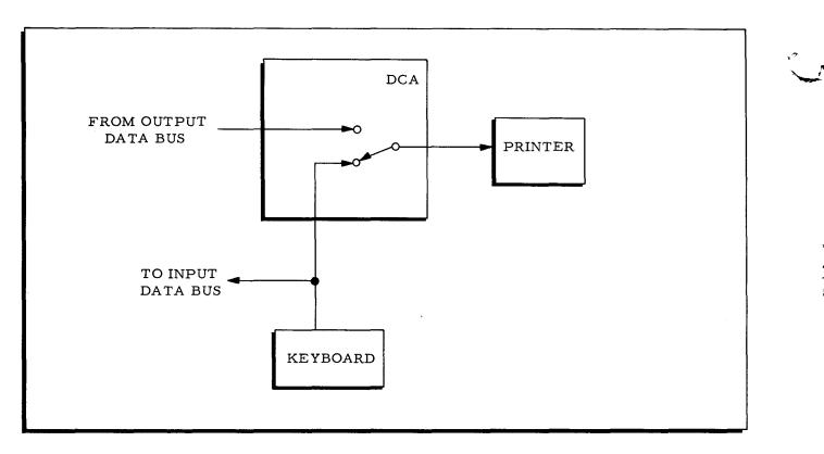
Figure 5-2. Keyboard and Printer Device Control Area Data Flow
