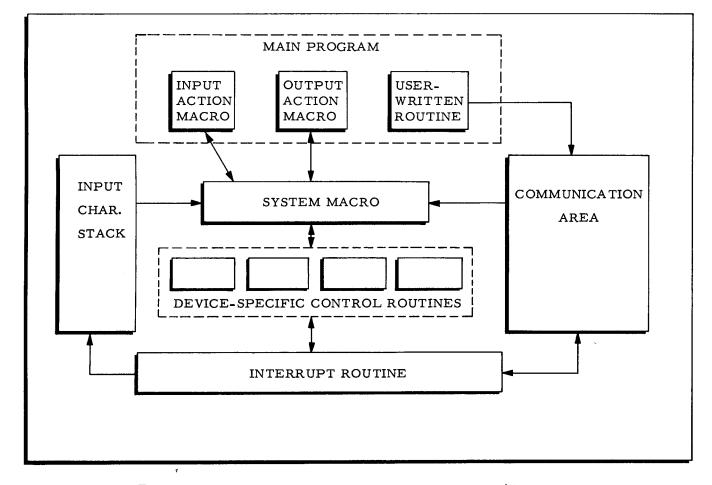
Figure 4-1. Functional Diagram of Communication I/O System
