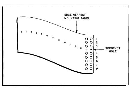
Figure 6-1. Paper Tape Code Alignment (Paper Tape Punch)
