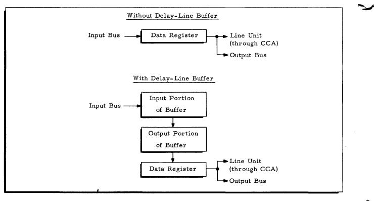
Figure 2-4. Remote-Mode Data Paths (Transmitting Data to Computer)
