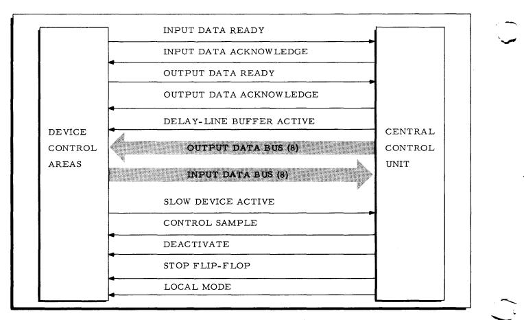
Figure 2-6. Central Control Unit Input/Output Bus
