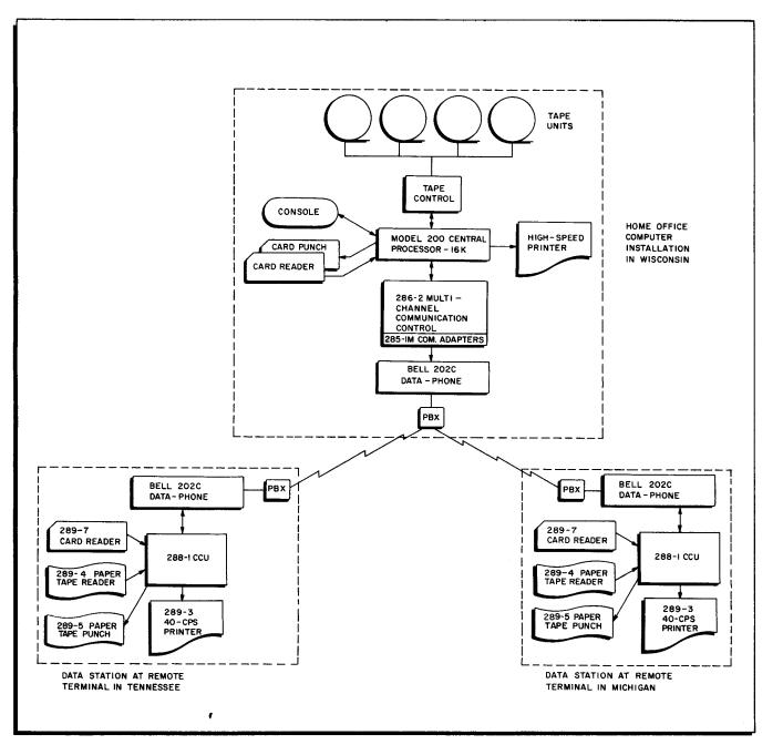
Figure 7-1. Manufacturing Company Communication System
