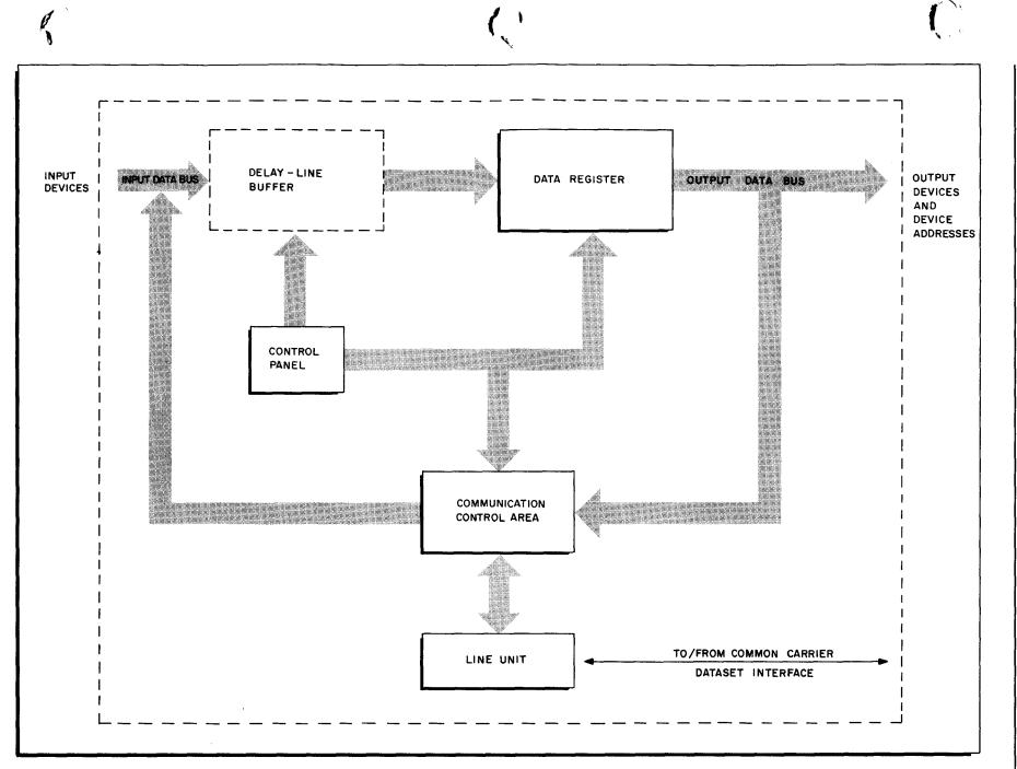
Figure 2-1. Functional Organization of Data Station Central Control Unit
