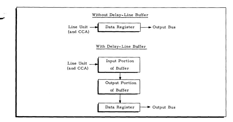
Figure 2-5. Remote-Mode Data Paths (Receiving Data from Computer)
