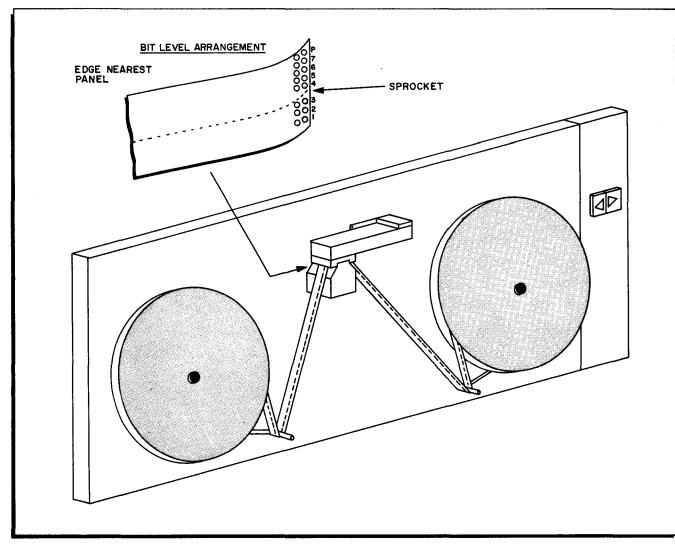
Figure 5-3. Paper Tape Reader Diagram
