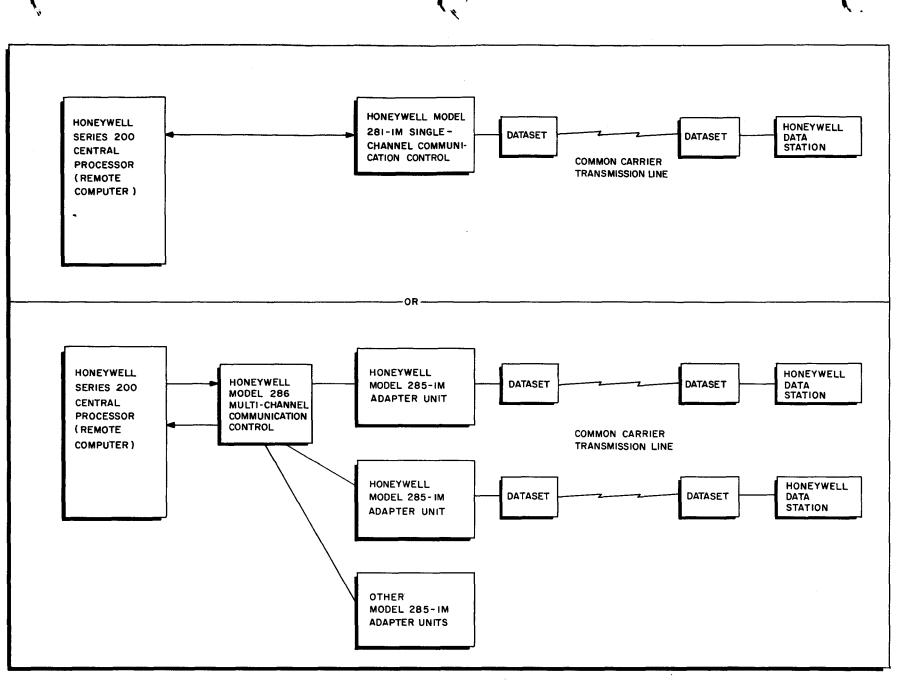
Figure 1-1. Data Flow Between the Central Processor and the Honeywell Data Station
