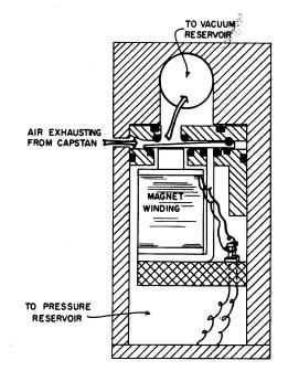
Fig. 7-Schematic of electro-pneumatic valve.
