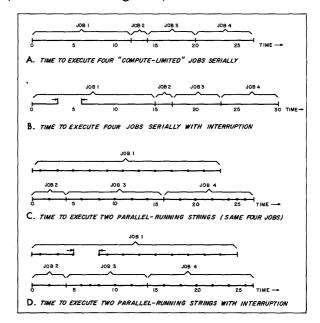
Figure 3. Parallel Processing of Two "Compute-Limited" Strings Absorbs Interruption Time
