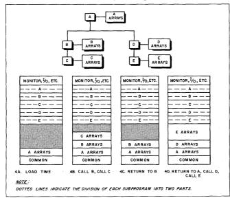
Figure 4. Dynamic Allocation of Non-Common Array Storage
