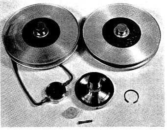
Fig. 4-Reels, reel mounts, and write-enable ring.
