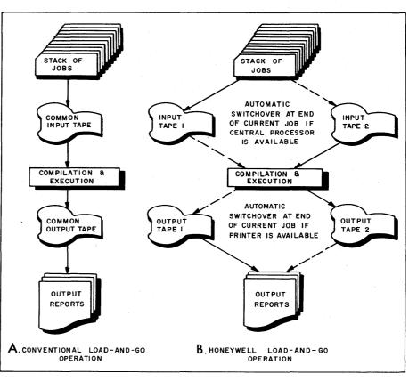
Figure 1. Comparison of Honeywell and Conventional Load-and-Go Techniques
