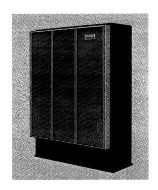
Addresses of individual tape units are specified by a simple tape-address patchboard associated with the tape control. Information transfer between each tape control and its associated magnetic tape units is independent of and simultaneous with such transfer for all other units.
