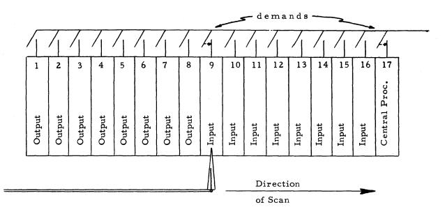
Figure II-2. Stages of Traffic Control
