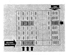
Fig. 3. Typical information array showing principle of two-dimensional detection
