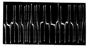
Fig. 10-Normal preamplifier output of read system.
