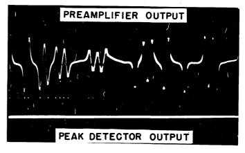
Fig. 11—Read system waveforms, including deliberate recorded dropout due to loose cotton lint.
