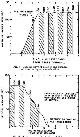
Fig. 9—Typical curve of velocity and distance vs. time during tape deceleration.
