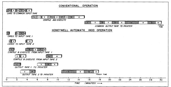
Figure 2. Timing Comparison Between Honeywell and Conventional Techniques
