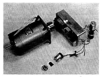
Fig. 5—Exploded view of capstans, brake and actuators.
