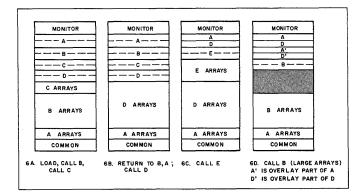
Figure 6. Dynamic Relocation, Loading from Tape, and Restoration from Tape
