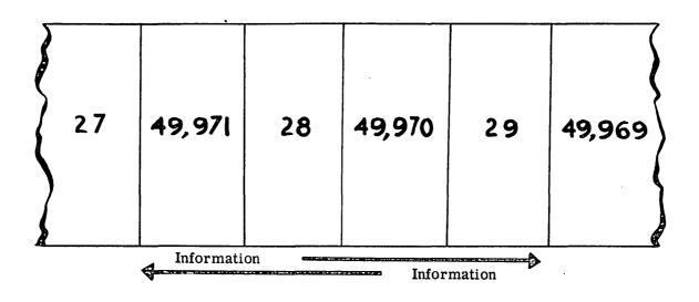
Figure 3. Interlacing of Blocks on DATAmatic 1000 Tape.
