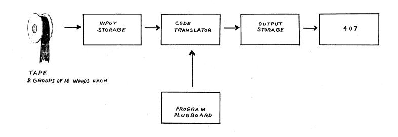
Figure 16. DATAmatic Output Converter Type 1300 Block Diagram.
