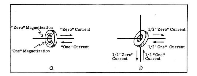
Figure 5. Typical Magnetic Core.
