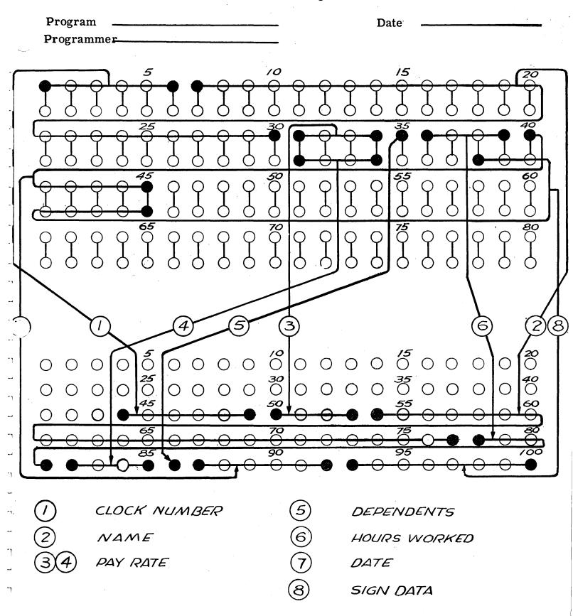
FIGURE **13** WORK SHEET Input Converter
