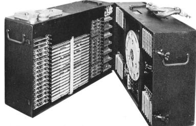
CP209 COMPUTER — first digital device performing bombing and navigation functions in an operational Navy attack bomber squadron.
