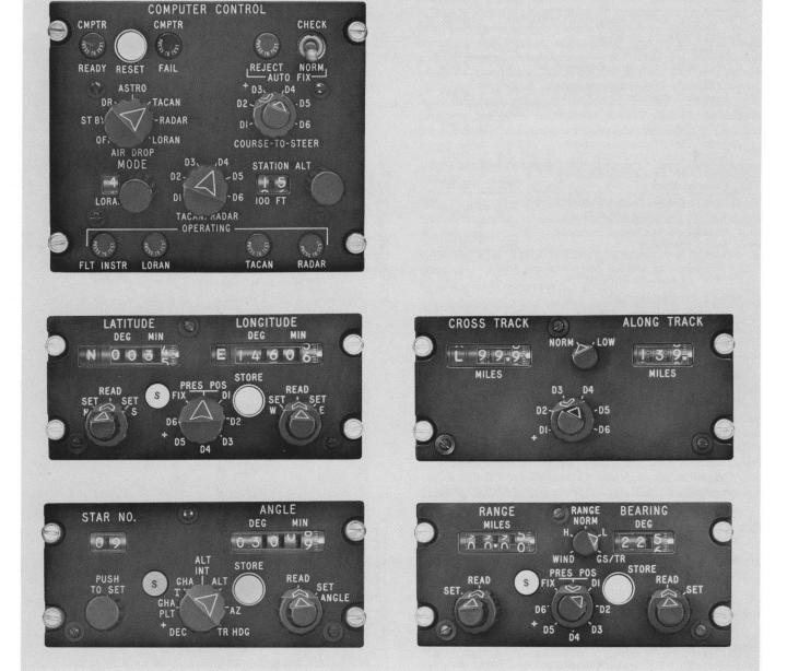
THE BASIC AN/ASN-24 (G) COMPUTER SET consists of nine units, but this number is alterable for particular system needs. Because of this flexibility, the specifications tabulated here typify a representative AN/ASN-24 (G) Computer Set, especially in regard to converter chassis weight and the total power requirements.
