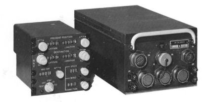
AN/ASN-41 COMPUTER SET — Now operational in the Navy's A4E, built by Douglas, marks the entry of a truly hybrid computer into the military service. It features a high accuracy miniature analog portion to perform the basic trigonometric functions and a digital integrator in the output providing high accuracy, highly reliable position data. This computer accepts Doppler inputs from the GPL AN/APN 153 radar.
