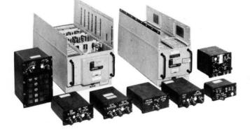
The AN/ASN-24 (G) general-purpose digital computer is the natural follow-on to its highly successful forerunner, the AN/ASN-24 (V) which, by early 1966, had logged more than 30,000 hours of flight operating time aboard the Air Force transport giant — the C-141 aircraft.
