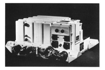
Outputs of this AN/ASN-24 modification are: • Three steering command signals to the guidance autopilot (for roll, pitch, and yaw axes) • Three gyro-torquing signals (for prelaunch platform alignment and for gyro drift compensation during flight) • Discrete output signals (for staging and for initiation and thrust cutoff sequences)
