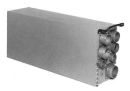
GPK-20 COMPUTER — A general - purpose digital computer for navigation and weapons delivery in military aircraft. Has modular random-access solid-state expandable core memory, arithmetic and control sections, A/D conversion, and power supply in a single unit, and incorporates selfprotection against memory loss.
