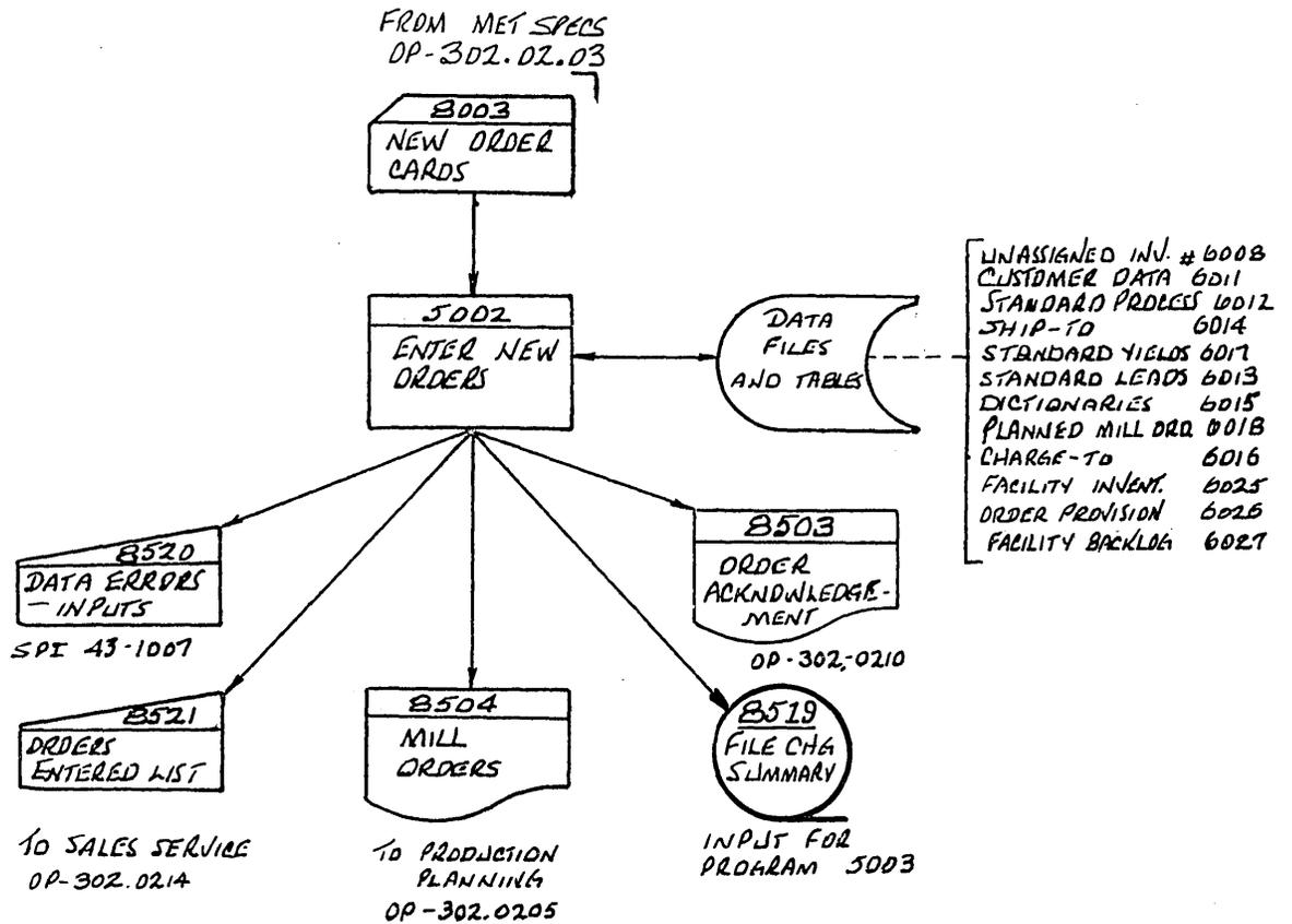
This level of chart may also be shown as a decision table in appropriate cases. Here inputs, outputs and files will be shown with the main processing box containing a reference to the table. Exhibit 3.3, Operating Procedures, is an example of a decision table.
