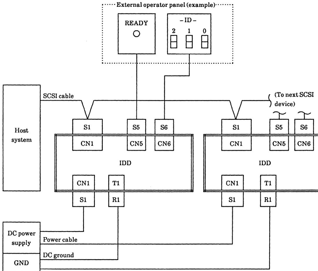
Figure 4.20 Cables connection
