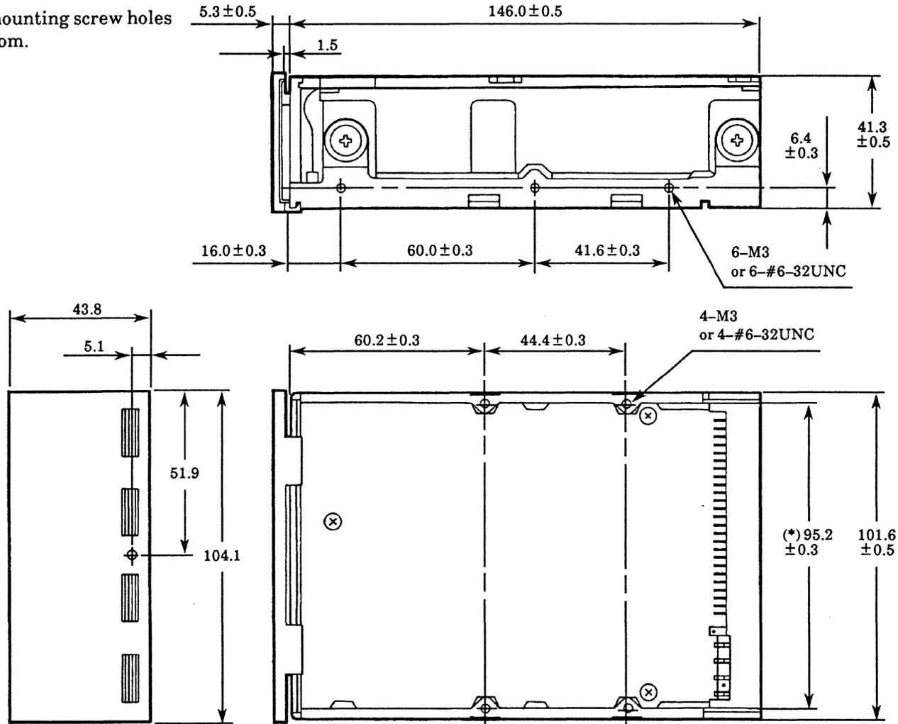
Figure 4.3 Exterior dimensions (M2624S with front panel)
