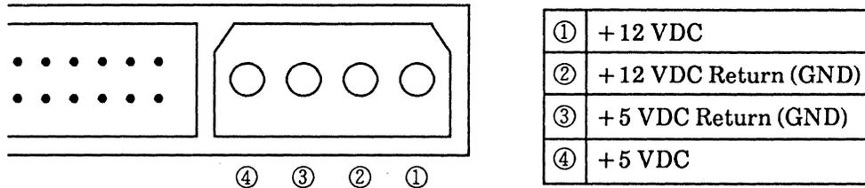
Figure 4.13 Power supply connector
