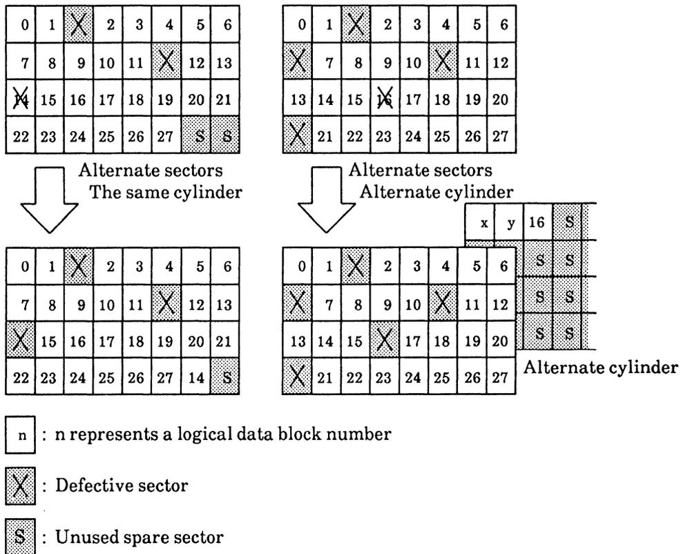
Figure 3.9 Alternate block allocation by REASSIGN BLOCKS command
