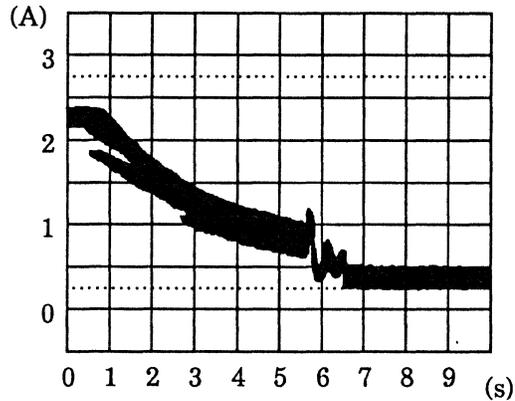
Figure 4.7 Current waveform (+12 VDC)
