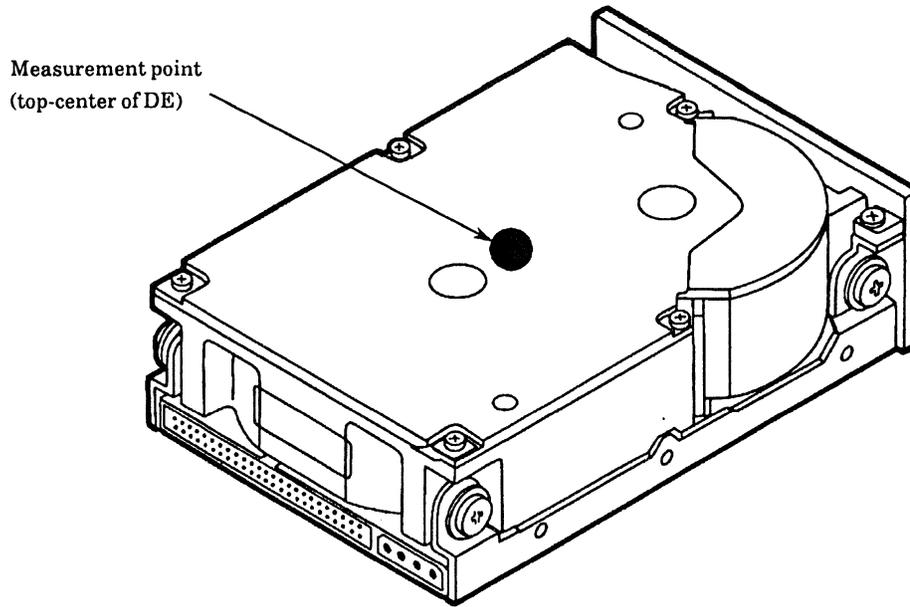
**Figure 4.1 DE surface temperature measurement point**
