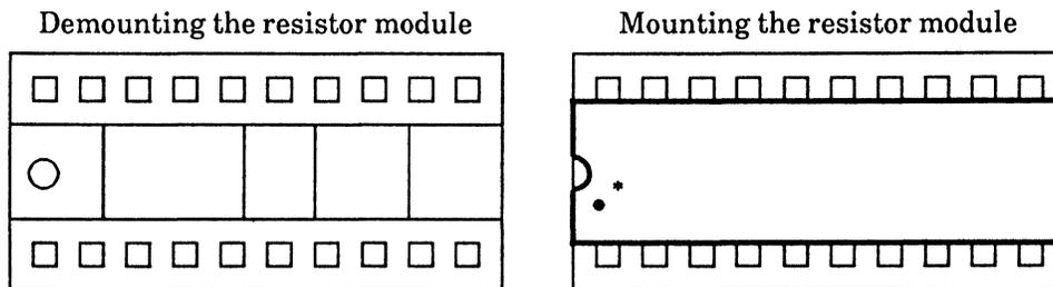
\*1 ● shows pin No. 1 of the resistor module.
