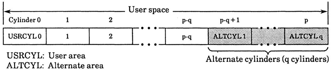
**Figure 3.3 Alternate cylinder**
