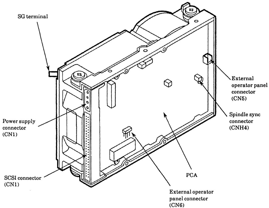
Figure 4.12 Positions of connectors (M2624S)
