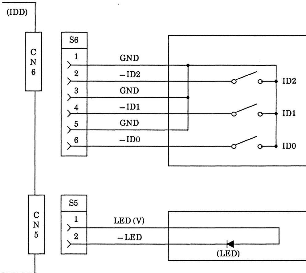
Figure 4.23 Example of external operator panel circuit
