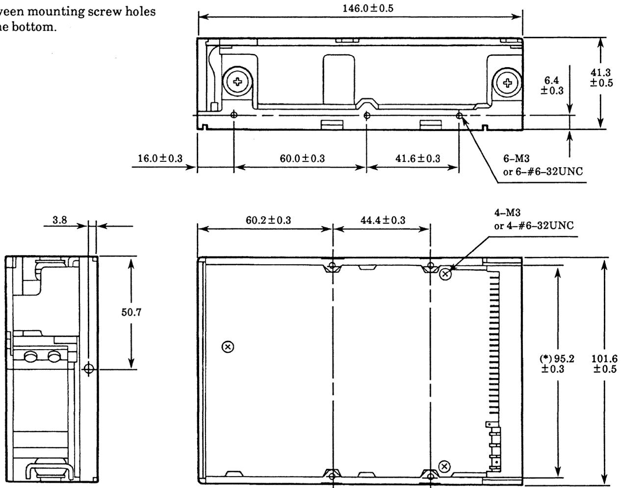
Figure 4.2 Exterior dimensions (M2624S without front panel)
