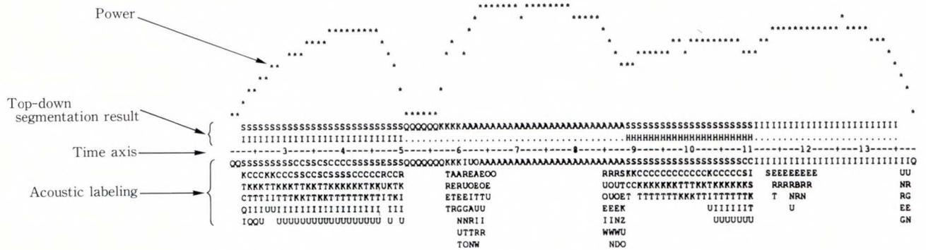
Fig. 5—Example of acoustic labeling and segmentation result.
