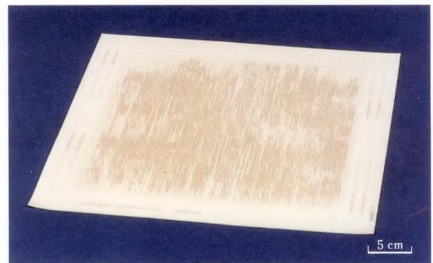
Fig. 10—Green sheet with copper pattern.
