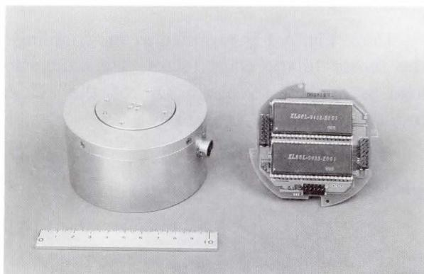
Fig. 6—Six-axis force/torque sensor and circuit board.
