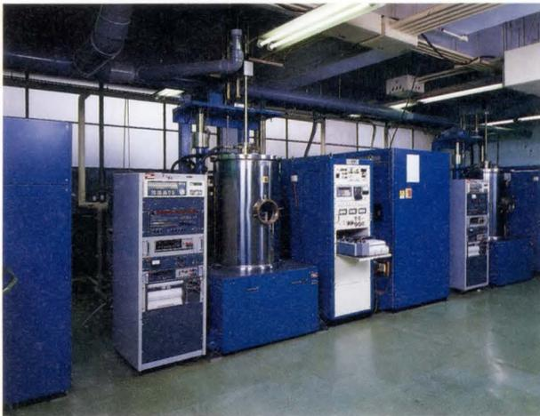
Fig. 12—Crystal growth stations at Fujitsu.
