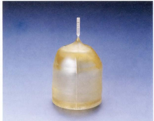
Fig. 13—As grown four-inch LN crystal under production at Fujitsu.
