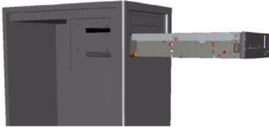
Figure 2-9 Installing the internal tape drive
