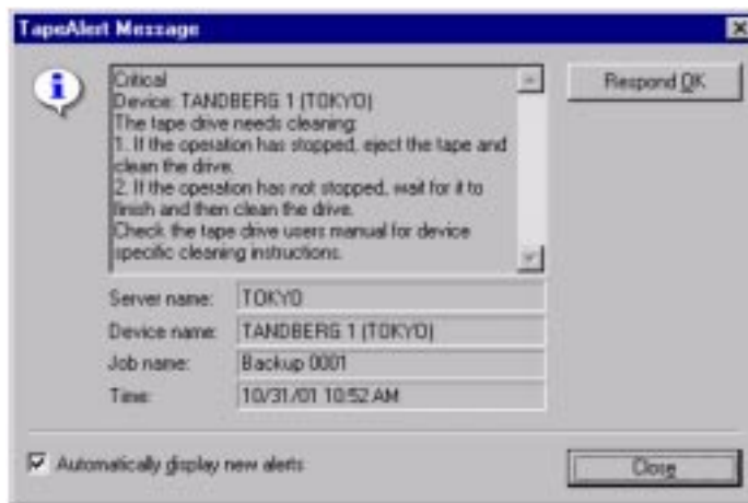
Figure 5-1 Backup Exec reporting that the tape drive needs cleaning
