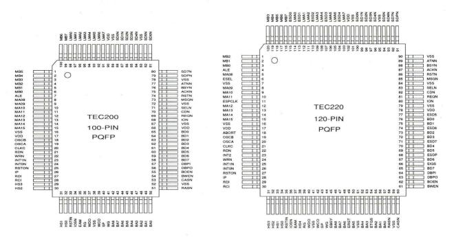
Figure 4. TEC 200 100-Pin PQFP Pin Diagram Figure 5. TEC 220 120-Pin PQFP Pin Diagram
