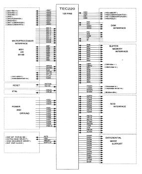
Figure 3. TEC 220 Functional Signal Grouping
