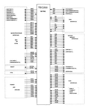
Figure 2. TEC 200 Functional Signal Grouping
