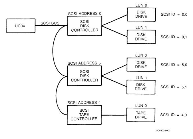
Figure 3-1. SCSI Bus Device Numbering Example
