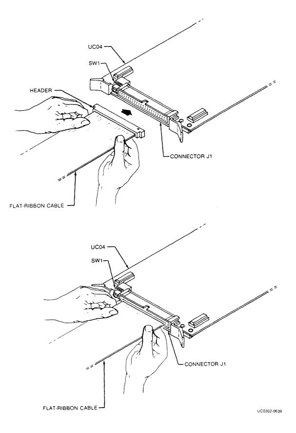
Figure 4-5. Plugging the Transadapter Flat Cable into Jl.
