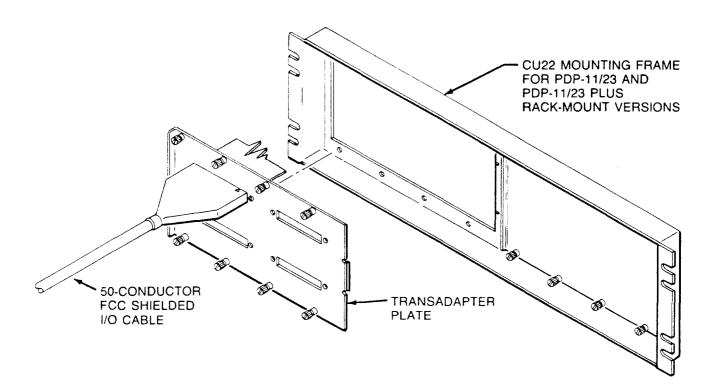
Figure 4-7. Installing the Universal Rack Mount Cabling Kit
