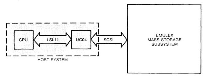
Figure 1-2. UC04 Subsystem Configuration
