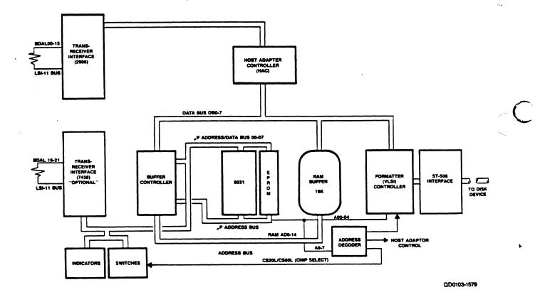
Figure 7-1. QD01/D Block Diagram
