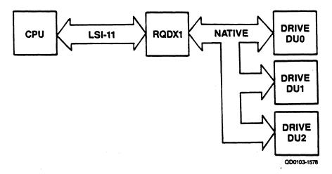
Figure 3-1. DEC MSCP Subsystem Logical and Physical Configuration
