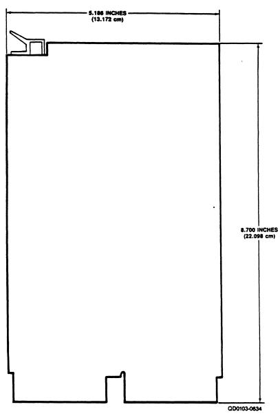
Figure 2-1. QD01/D Disk Controller Dimensions
