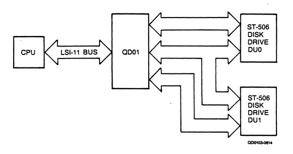
Figure 3-2. QD01/D Subsystem Logical and Physical Configuration
