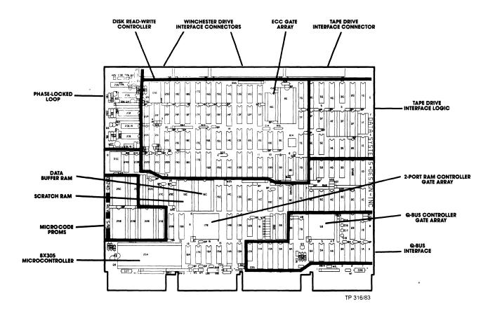
Figure 3-1. DSD 8240 Controller Board
