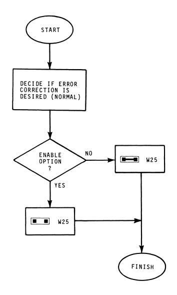
Figure 4-11. Error Correction Option TP 523/83
