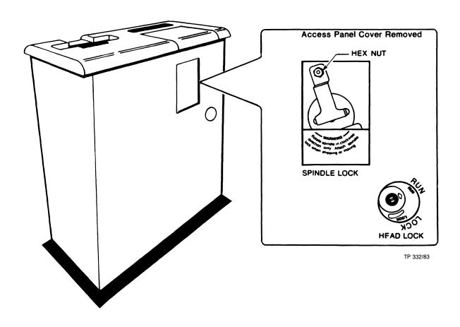
Figure 4-3. Winchester Spindle and Head Lock
