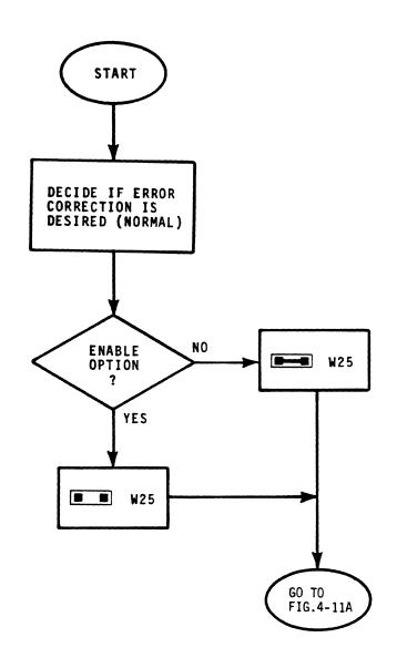
Figure 4-11. Error Correction Option TP 523 83
