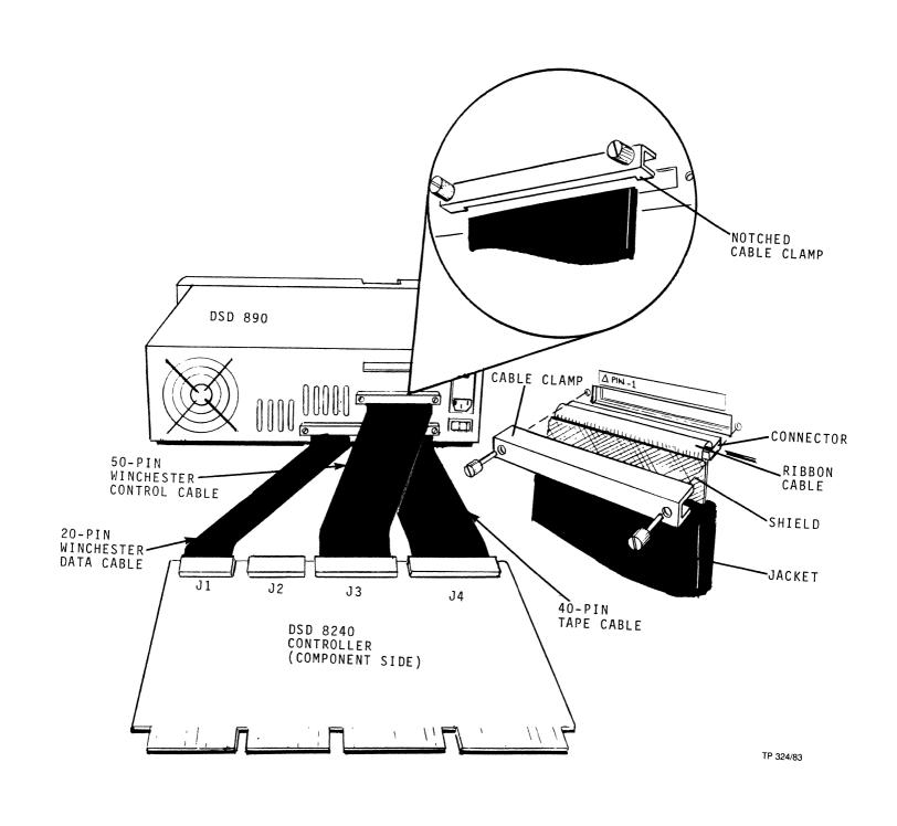
Figure 4-5. Cabinet and Board Cabling
