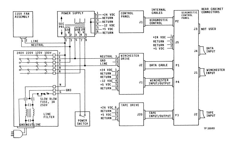
Figure 7-7. Power Distribution Diagram
