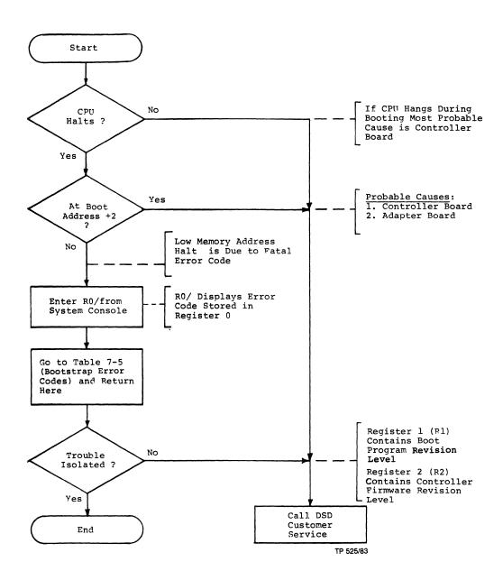
Figure 7-6. Bootstrapping Failure.
