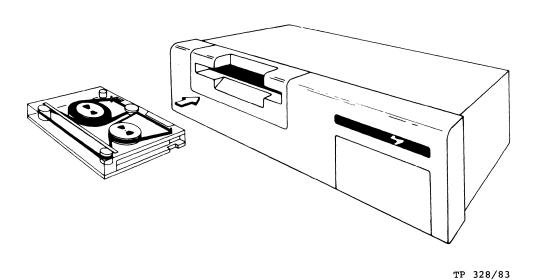
Figure 5-2. Inserting the Cartridge
