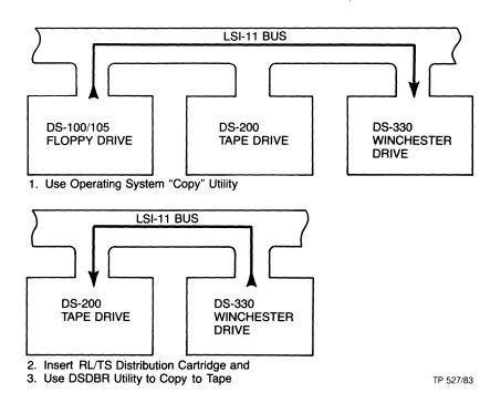
Figure 4-13. Transferring Software Using Floppy
