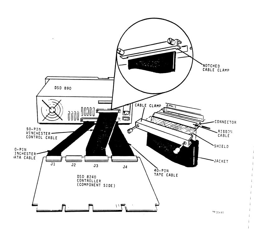
Figure 4-5. Cabinet and Board Cabling
