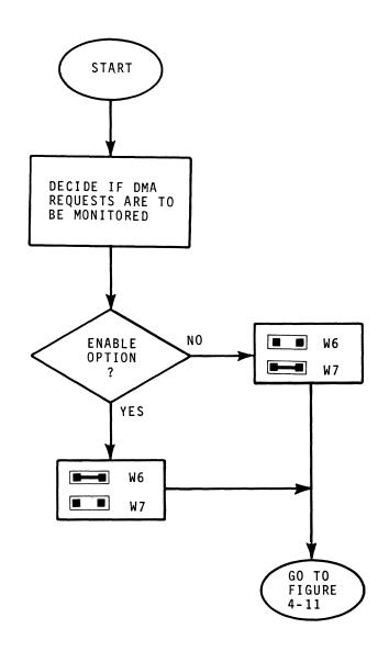
Figure 4-10. DMA Request Monitor Option TP 522/83
