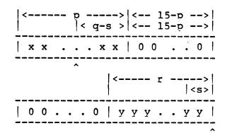
The significant digits of x are then continuously divided by the significant digits of y until 15 decimal digits are generated. Referring to the above diagram, note that the number of fractional digits produced by the division is determined by the placement of the adjusted decimal point in x. The field following the decimal point contains (q-s) plus (15-p) positions, yielding the following precision and scale for the result of the division
