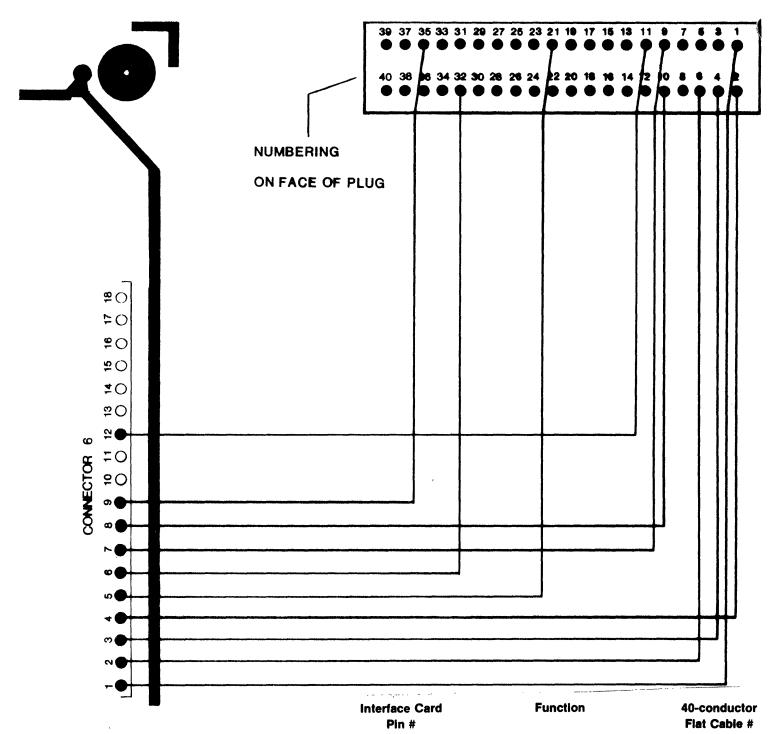
Connections for the printer to the interface card connector 6 are detailed below, pin to pin with the function provided.
