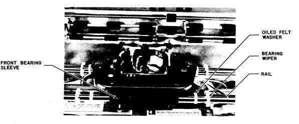
Figure 5-19 CARRIAGE AND RAIL REASSEMBLY
