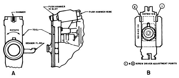
Figure 5-28 PRINT WHEEL TO HAMMER ALIGNMENT
