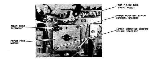
Figure 5-9 PAPER FEED MOTOR REMOVAL
