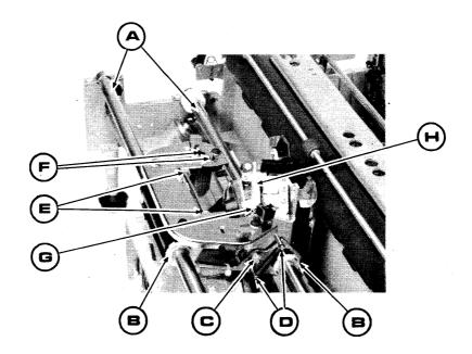
Figure 5-1 CARRIAGE SYSTEM LUBRICATION POINTS
