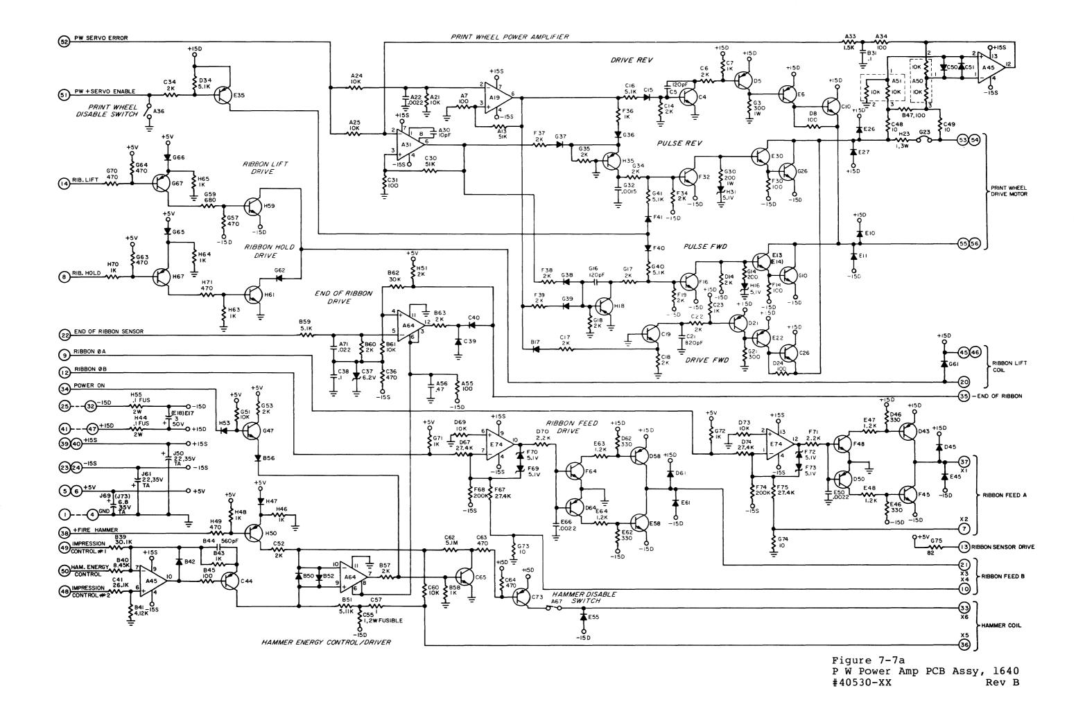
Figure 7-7a Print Wheel Power Amplifier PCB Assy, 1640 Series #40530-10 Rev B
