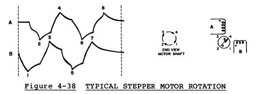
Figure 4-38 illustrates the development of stepper motor rotation from two inputs  $90^{\circ}$  out of phase with each other. Actually, the paper feed stepper motor's rotor has a magnetic node each 7.5°. This would be difficult to illustrate. It should be noted, therefore, that for clarity the illustration depicts a stepper rotor with magnetic nodes every  $90^{\circ}$  only.
