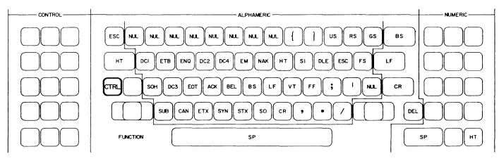
Figure 2-16 CTRL MODE KEY ASSIGNMENT
