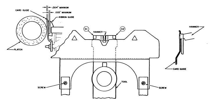
Figure 5-22 CARD GUIDE ADJUSTMENTS
