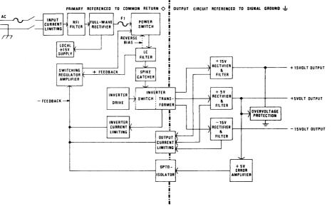
Figure 4-43 INTERNAL POWER SUPPLY BLOCK DIAGRAM, B
