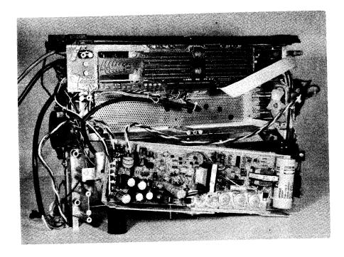
Figure 5-44 POWER SUPPLY REMOVAL/INSTALLATION
