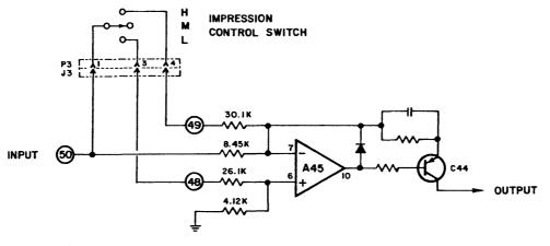
Figure 4-39 HAMMER ENERGY CONTROL CIRCUIT
