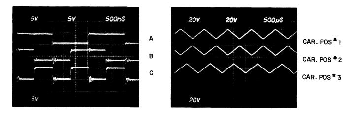
Figure 4-24 SERVO FEEDBACK DEMODULATOR/INTEGRATOR/AMPLIFIER WAVEFORMS
