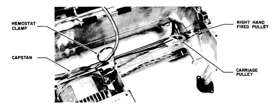
Figure 5-36 RIGHT-HAND CARRIAGE DRIVE CABLE INSTALLATION
