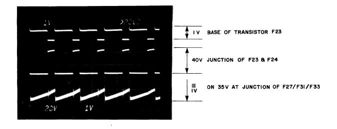
Figure 4-18 -30 VOLT POWER INVERTER WAVEFORMS
