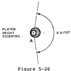
Figure 5-26 PLATEN HEIGHT ECCENTRICS ADJUSTMENT LIMITS
