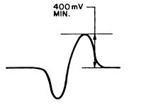
Figure 5-30 PRINT WHEEL HOME SENSOR WAVEFORM
