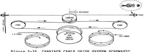
Figure 5-35 CARRIAGE CABLE DRIVE SYSTEM SCHEMATIC
