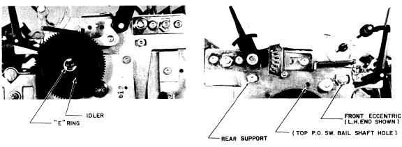
Figure 5-7 CARRIER SYSTEM REMOVAL - B
