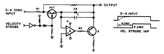
Figure 4-28 TYPICAL SAMPLE AND HOLD CIRCUIT
