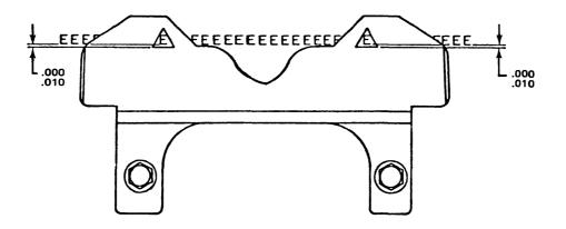
Figure 5-24 CARD GUIDE ALIGNMENT
