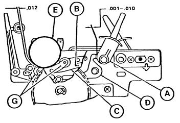
Figure 5-12 PAPER FEED ADJUSTMENTS
