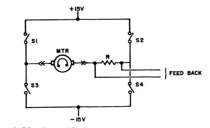
Figure 4-32 CARRIAGE POWER AMPLIFIER SIMPLIFIED DIAGRAM
