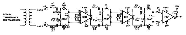
Figure 4-21 SERVO FEEDBACK AMPLIFIER
