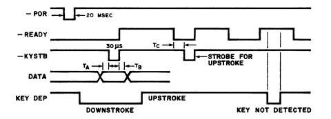
$T_A = 5 \mu s$  MINIMUM: DATA BITS STABLE BEFORE STROBE IS ACTIVE.  $T_B = 5 \mu s$  MINIMUM: DATA BITS STABLE AFTER STROBE GOES HIGH.  $T_C = 10 \mu s$  MINIMUM: READY ACTIVE LOW UNTIL NEW STROBE IS SENT. NOTE: DATA IS TAKEN DURING 'T<sub>B</sub>'.
