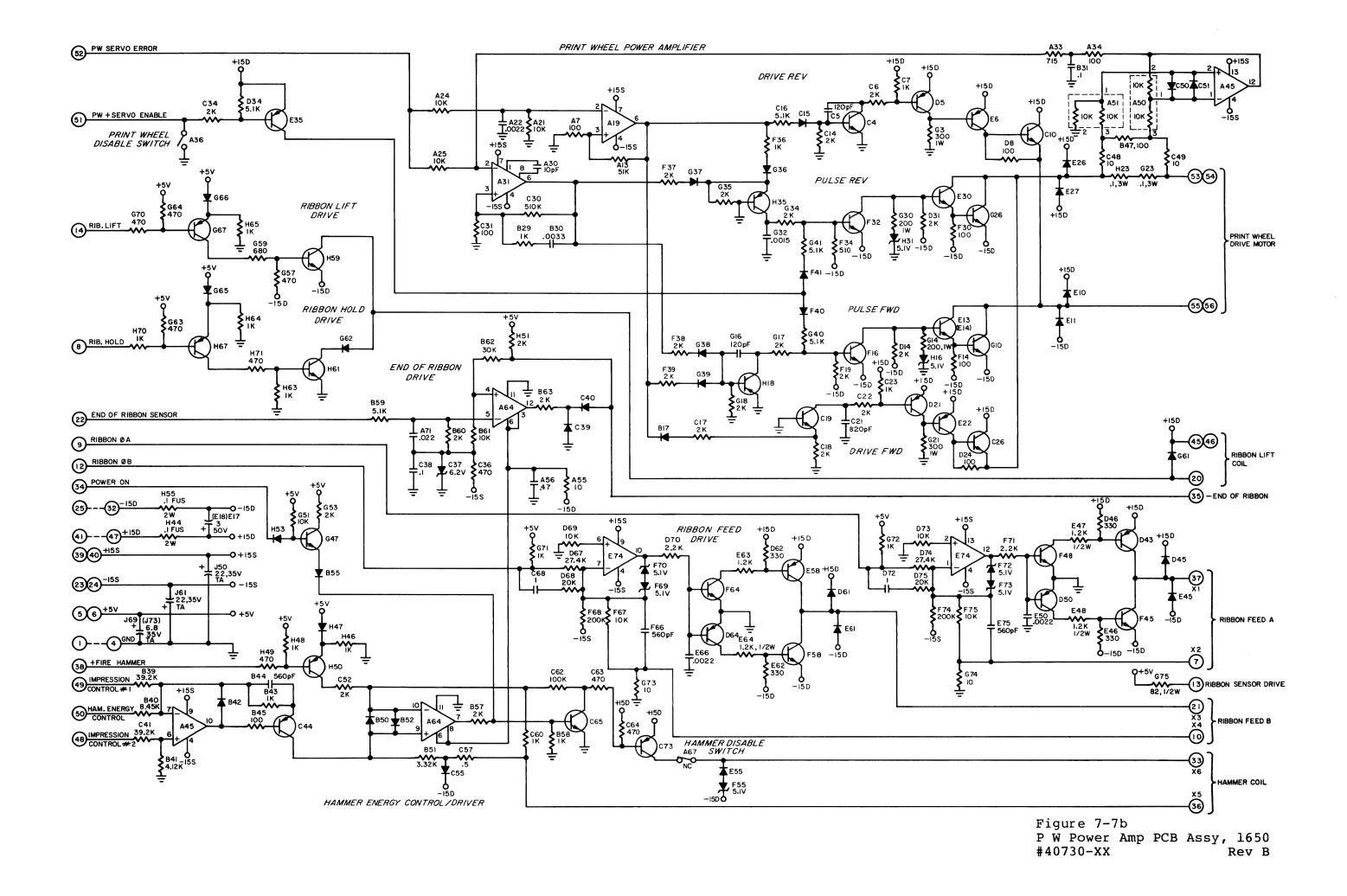
Figure 7-7b Print Wheel Power Amplifier PCB Assy, 1650 Series #40730-10 Rev B
