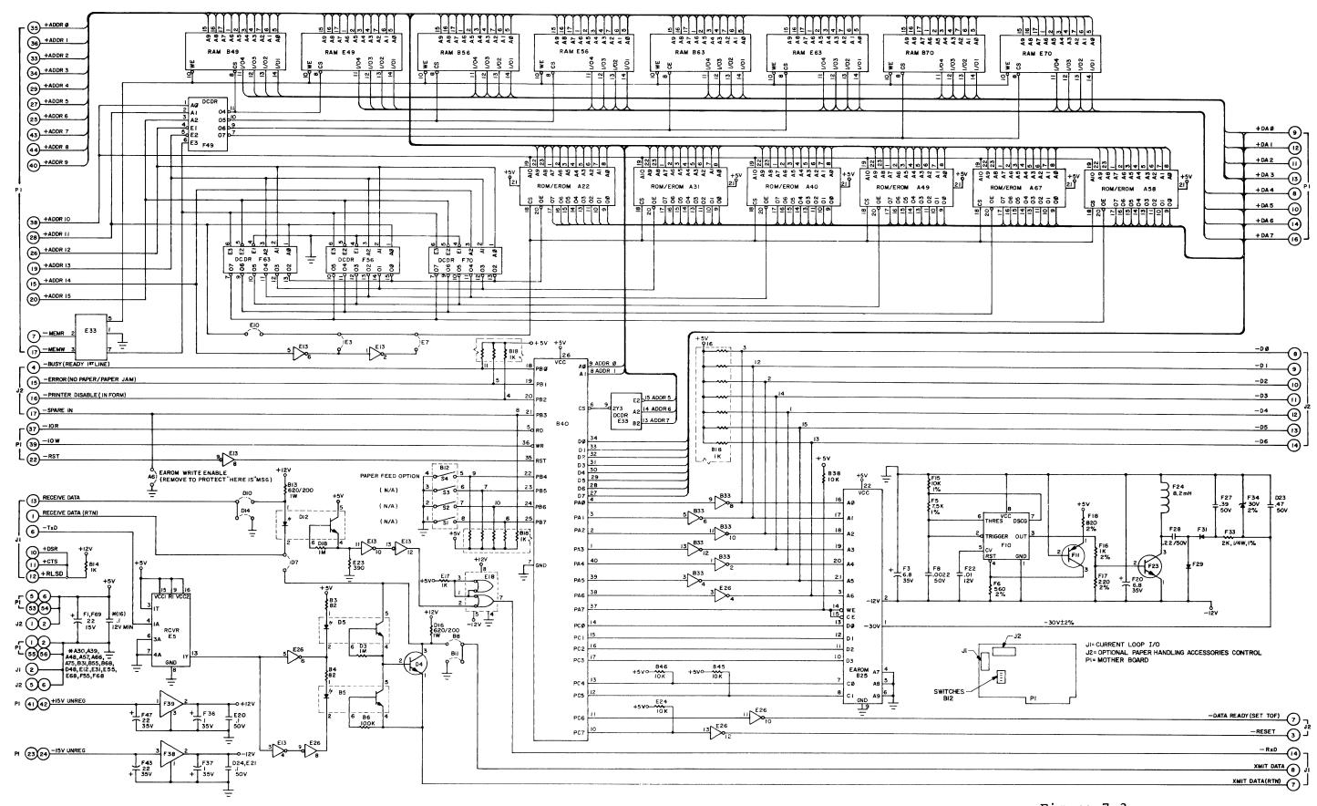
Figure 7-3 XMEM2 Expanded Memory PCB Assy #400664-XX Rev C Figure 7-3 XMEM2 Expanded Memory PCB Assy #400664-XX Rev C
