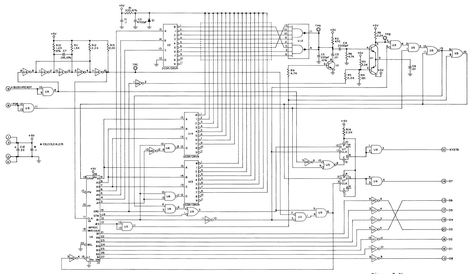
Figure 7-9b Keyboard PCB Assy, C #301658-01 Rev B Figure 7-9b Keyboard PCB Assy, C #301658-01 Rev B
