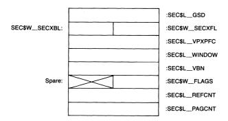
**Figure B-36**Layout of a Section Table Entry
