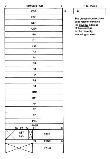
**Figure B-25**Layout of the Hardware Process Control Block
