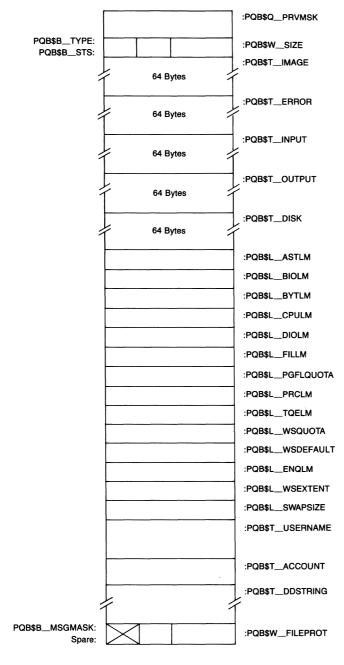
**Figure B-29**Layout of a Process Quota Block
