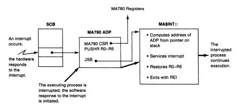
**Figure 5-6**Control Flow in Servicing an MA780 Interrupt
