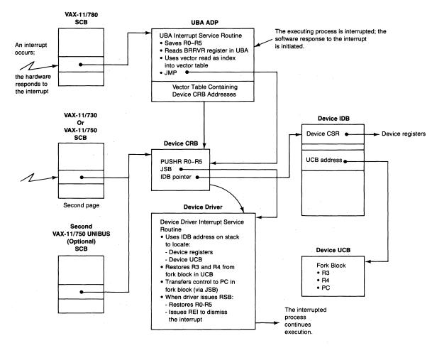
**Figure 5-3**Control Flow in Servicing a UNIBUS Interrupt
