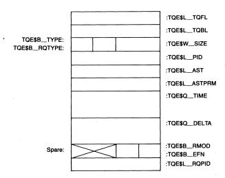
**Figure B-39**Layout of a Timer Queue Element
