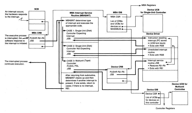
**Figure 5-4**Control Flow in Servicing a MASSBUS Interrupt
