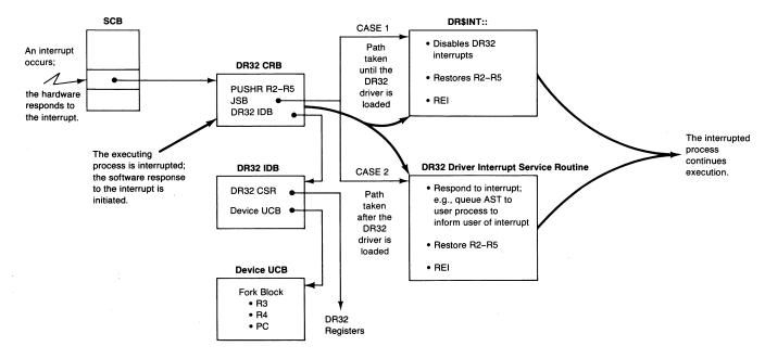
**Figure 5-5**Control Flow in Servicing a DR32 Interrupt
