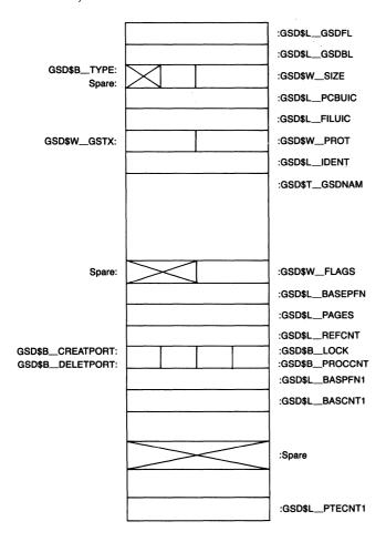
**Figure B-7**Layout of a Global Section Descriptor
