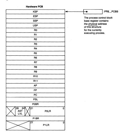
Figure 10-6 Hardware Process Control Block
