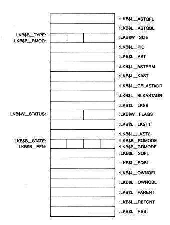
Figure B-19 Layout of a Lock Block
