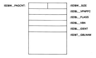
**Figure B-14**Layout of an Image Section Descriptor
