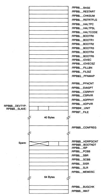
**Figure B-34**Layout of the Restart Parameter Block
