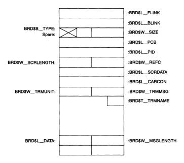
**Figure B-2**Layout of a Broadcast Descriptor Block
