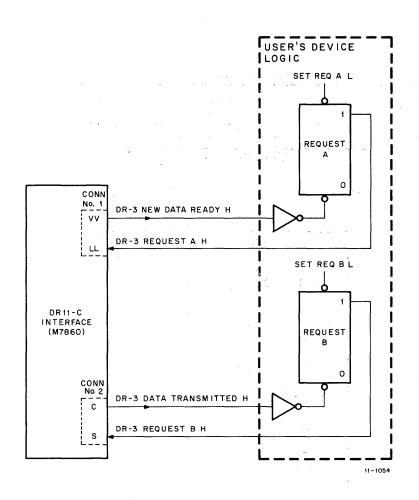
Figure 6-3 Request Line Control Logic
