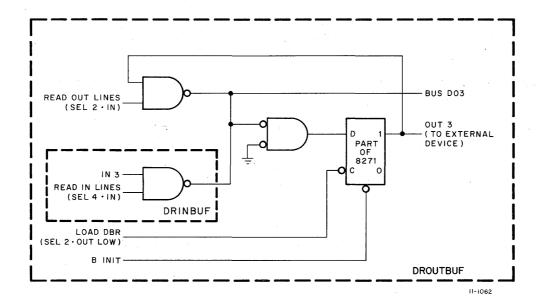
Figure 4-7 Input and Output Buffers, Simplified Diagram (one bit position)
