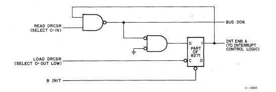
Figure 4-5 Status Register Input/Output Gating (one bit position)
