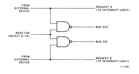
Figure 4-6 DRCSR Read-Only Bits (REQUEST A and B)
