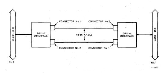
Figure 6-4 Interprocessor Buffer, Simplified Diagram
