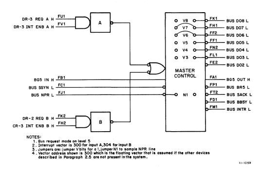
Figure 4-4 Interrupt Control Logic, Simplified Block Diagram
