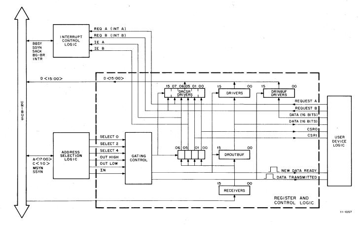
Figure 4-1 DR11-C Interface, Block Diagram
