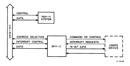
Figure 1-1 System Block Diagram
