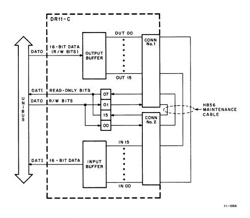
Figure 5-1 DR11-C Bits Jumpered by Maintenance Cable
