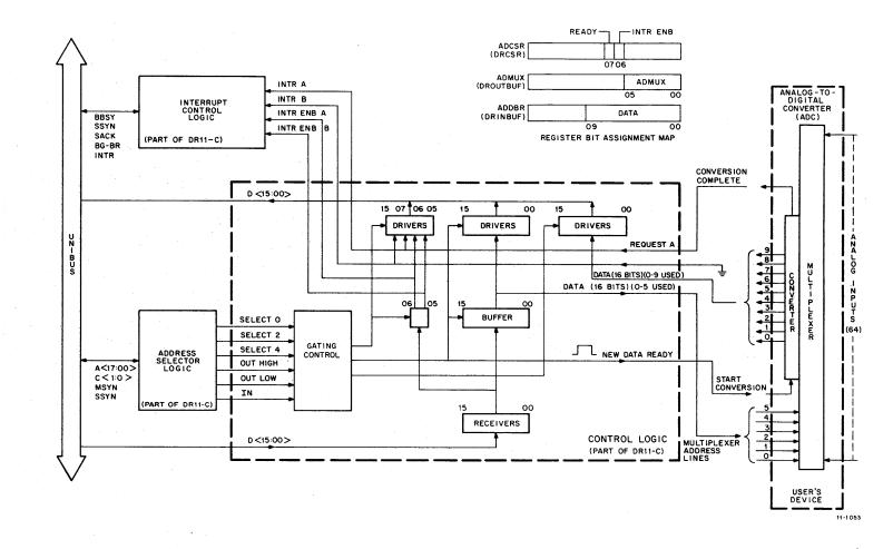
Figure 6-2 Interrupt Serviced Interface
