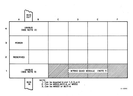
Figure 1-2 Typical M7860 Quad Module Mounting In a DD11-A
