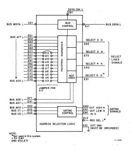
Figure 4-2 Address Selection Logic, Simplified Diagram
