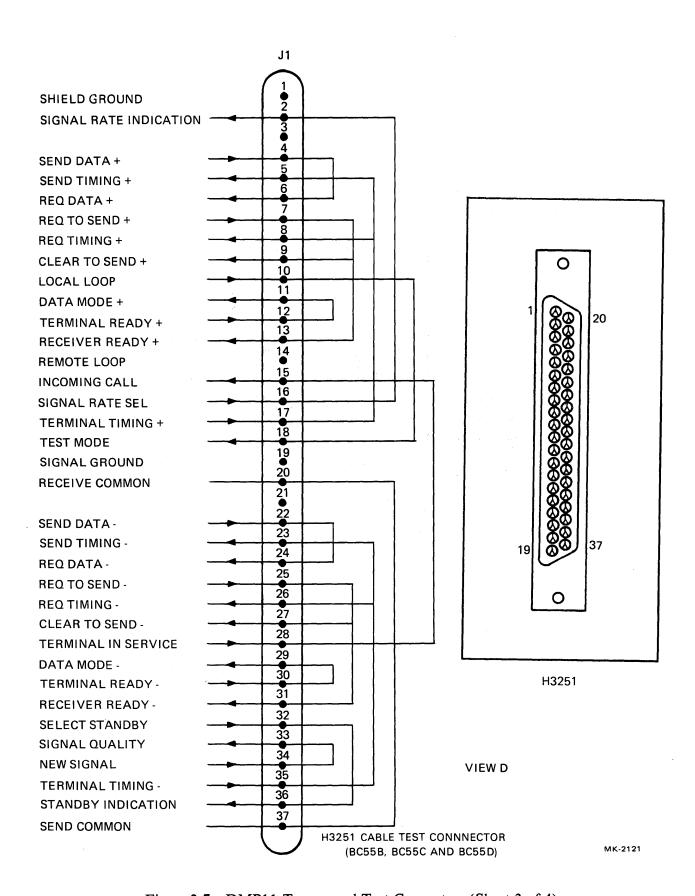
Figure 2-7 DMP11 Turnaround Test Connectors (Sheet 3 of 4)
