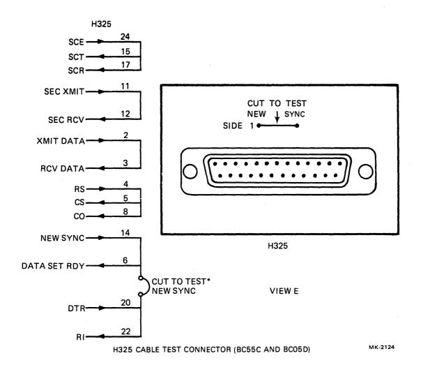
Figure 2-7 DMP11 Turnaround Test Connectors (Sheet 4 of 4)
