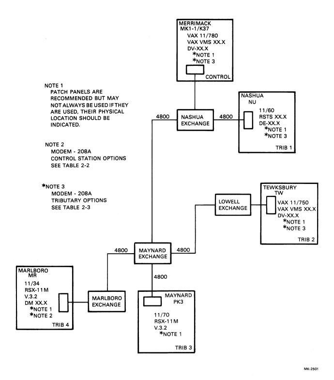
Figure 2-2 Example of a Topology Diagram for a Remote Multipoint Network
