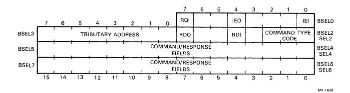
Figure 3-2 Command and Response Fixed and Variable Formats
