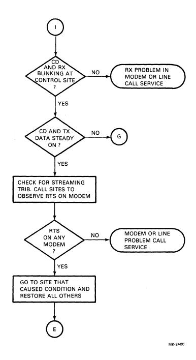
Figure 6-1 Typical Isolation Troubleshooting Flowchart (Sheet 3 of 5)
