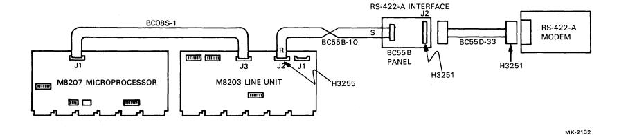
Figure 2-8 DMP11 Remote System Cabling Diagram (Sheet 1 of 2)
