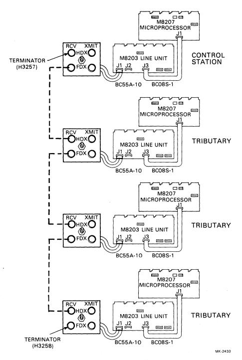
Figure 2-11 Multipoint Cable Routing Example Full-Duplex Control Station End Node
