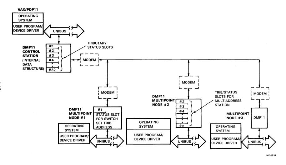
Figure 1-4 Block Diagram of a Multipoint Network with Multiple Tributary Addresses
