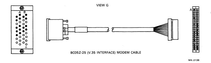
Figure 2-6 DMP11 Cable Drawings (Sheet 3 of 3)
