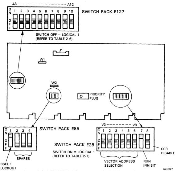
Figure 2-3 M8207-YA Microprocessor Switch/Jumper Locations
