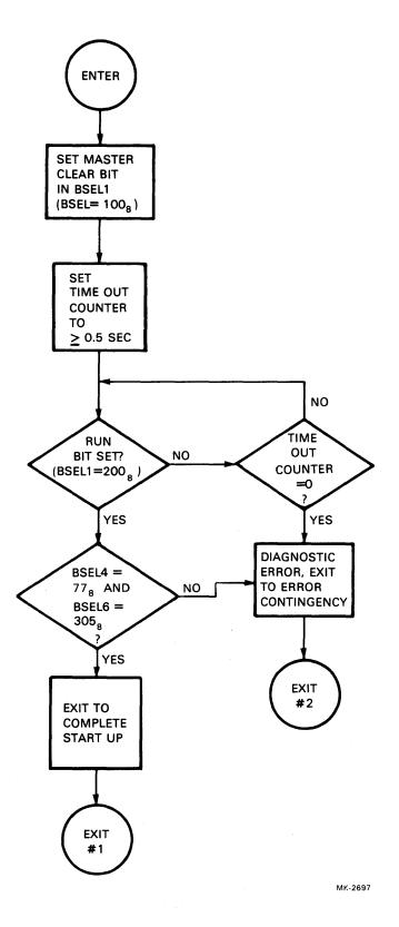
Figure 3-4 Flowchart for a Routine to Initialize the DMP11
