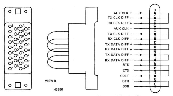
Figure 2-7 DMP11 Turnaround Test Connectors (Sheet 1 of 4)
