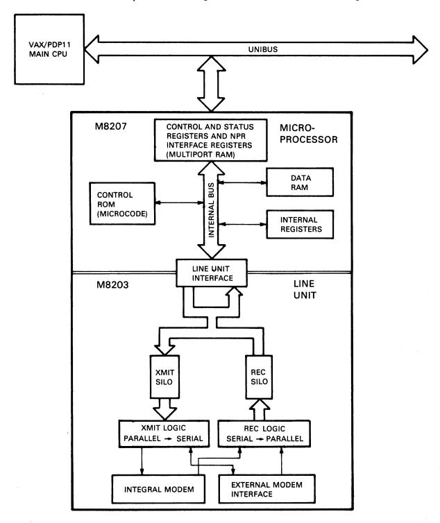
Figure 1-1 Simplified Block Diagram
