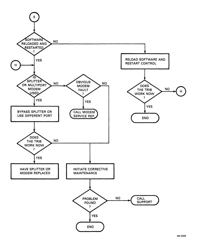
Figure 6-1 Typical Isolation Troubleshooting Flowchart (Sheet 5 of 5)
