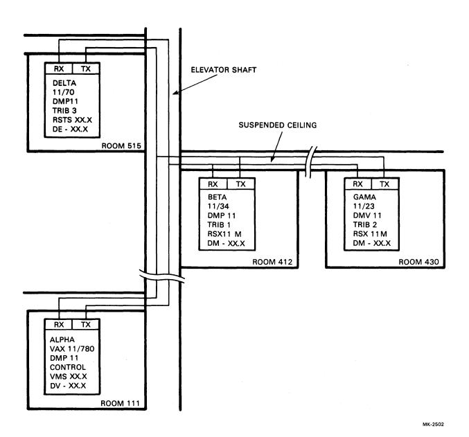
Figure 2-1 Example of a Topology Diagram for a Local Multipoint Network
