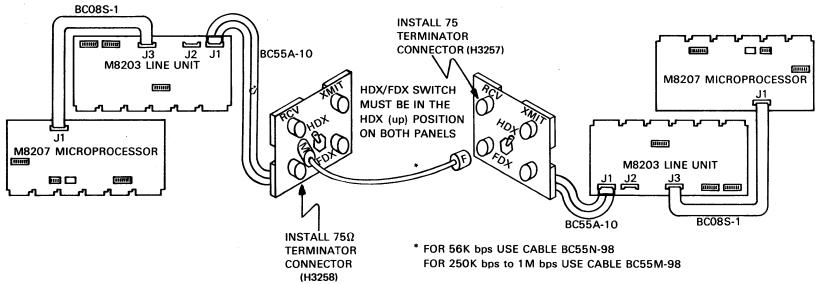
Figure 2-10 Multipoint Cable Routing Example Half-Duplex
