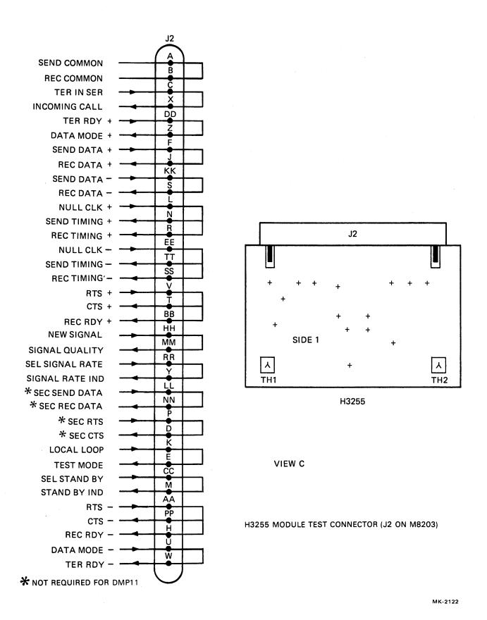
Figure 2-7 DMP11 Turnaround Test Connectors (Sheet 2 of 4)
