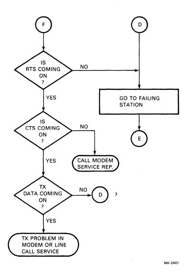
Figure 6-1 Typical Isolation Troubleshooting Flowchart (Sheet 4 of 5)
