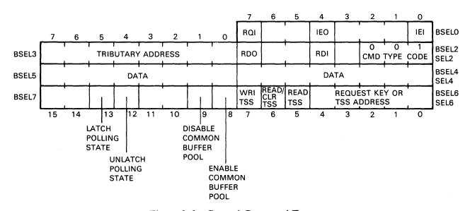
Figure 3-6 Control Command Format
