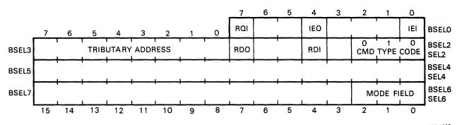
Figure 3-5 Mode Definition Command Format
