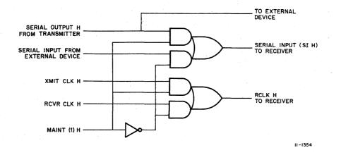
Figure 5-9 Maintenance Logic – Simplified Diagram
