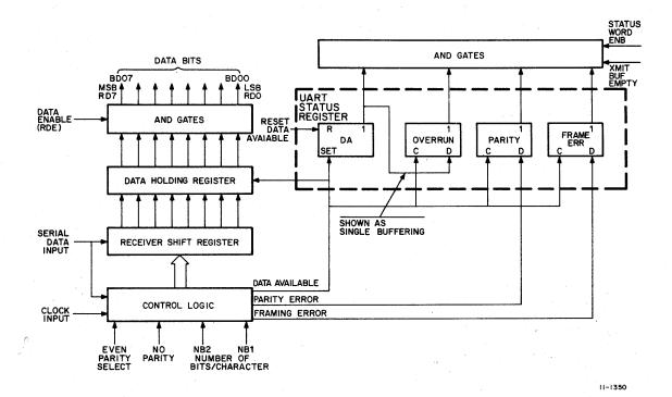
Figure 5-5 UART Receiver – Block Diagram
