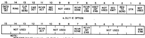
RDR ENB (bit 0) used only with DL11-A and DL11-C b.DL11-A THROUGH DL11-D OPTIONS
