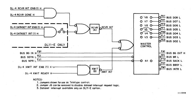
Figure 5-3 Interrupt Control Logic – Simplified Diagram
