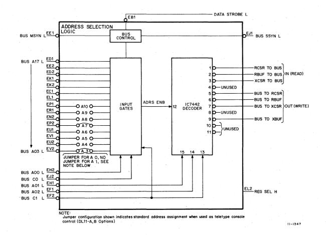
Figure 5-1 Address Selection Logic – Simplified Diagram
