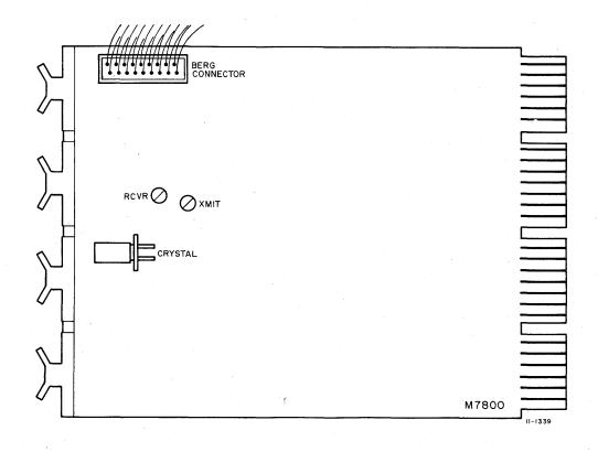
Figure 2-4 Crystal and Switch Location
