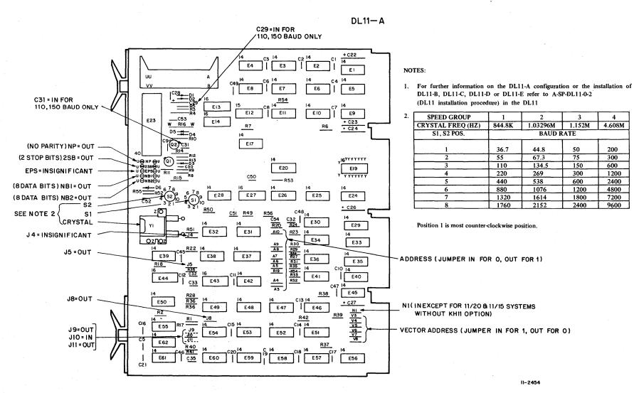
Figure 3-2 Jumper Locations on the M7800 Module
