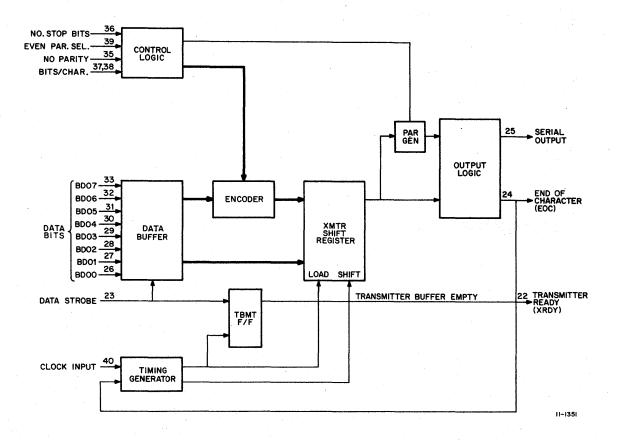
Figure 5-6 UART Transmitter - Block Diagram
