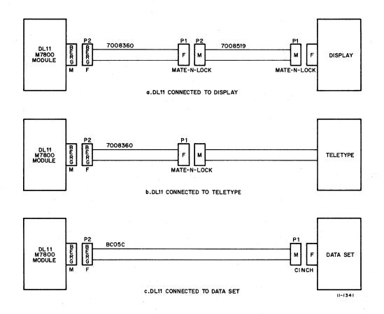
Figure 3-3 DL11 Cable Connections
