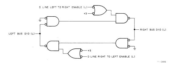
Figure 3-2 D Line Logic Circuit
