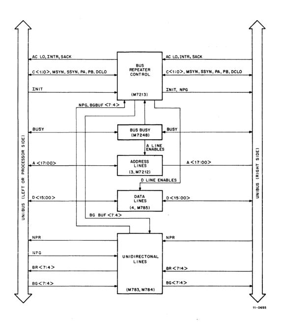
Figure 1-1 DB11 Bus Repeater Block Diagram
