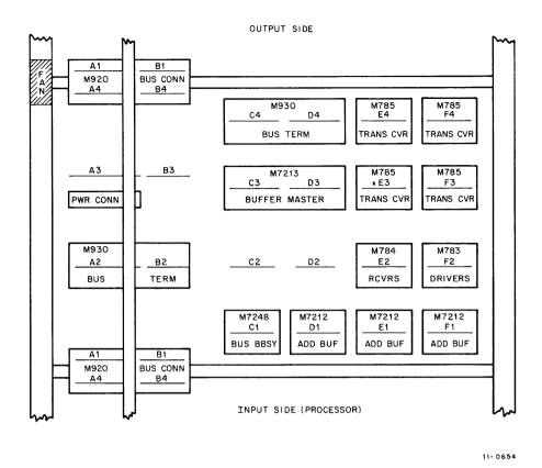
Figure 2-1 DB11 System Unit Layout
