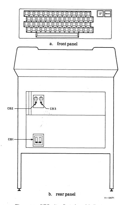
Figure 3-1 DECwriter Controls and Indicators
