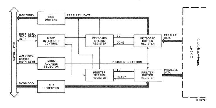
Figure 2-1 LC11 Controller—Simplified Block Diagram
