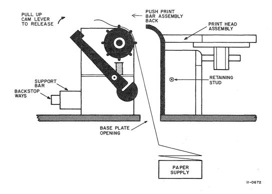
Figure 3-2 Loading Paper into LA30 DECwriter
