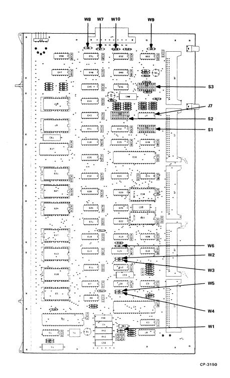
Figure 3-7 LS120 Logic Board
