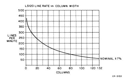
Figure 4-2 LS120 Line Rate Versus Column Width
