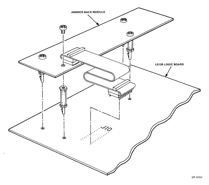
Figure 7-6 Installation of the Answerback Board
