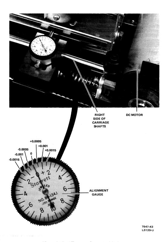
Figure 7-14 Alignment Gauge Positioning
