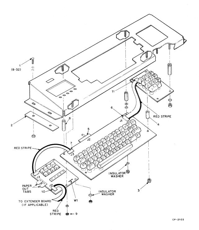
Figure 7-5 Keyboard and Bezel Assembly - Cabling and Hardware
