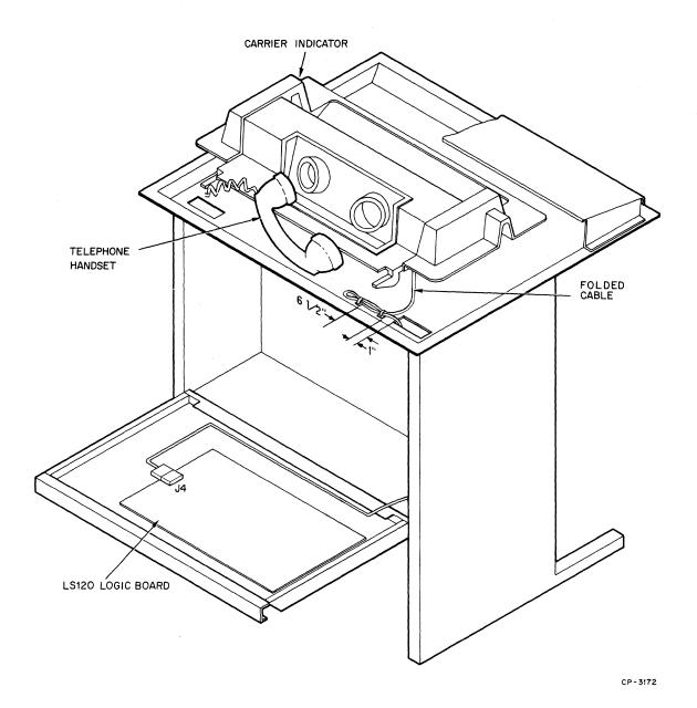
Figure 7-10 Installation of Acoustical Coupler Option Kit (LAXX-LM)
