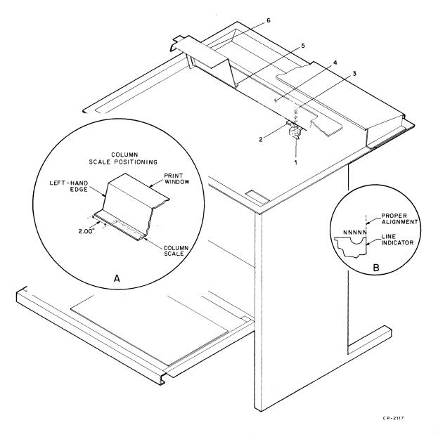
Figure 7-4 Installation of Scale and Pointer
