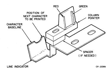
Figure 7-3 Line Indicator and Column Pointer
