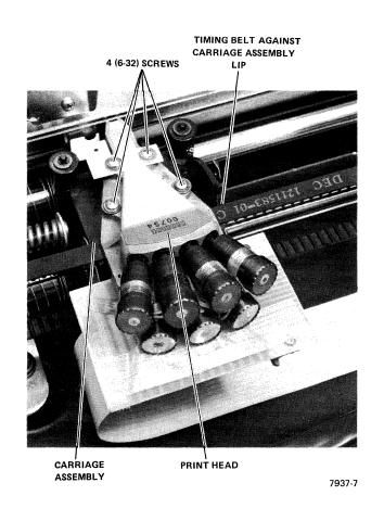
Figure 7-12 Remove Print Head and Ribbon Cable
