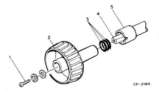
Figure 7-9 Installation of O Ring on Tractor Drive Shaft
