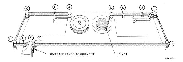
Figure 2-9 Ribbon Installation
