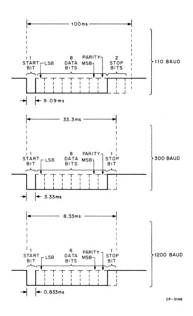
Figure 3-5 Serial Interface Timing Diagram
