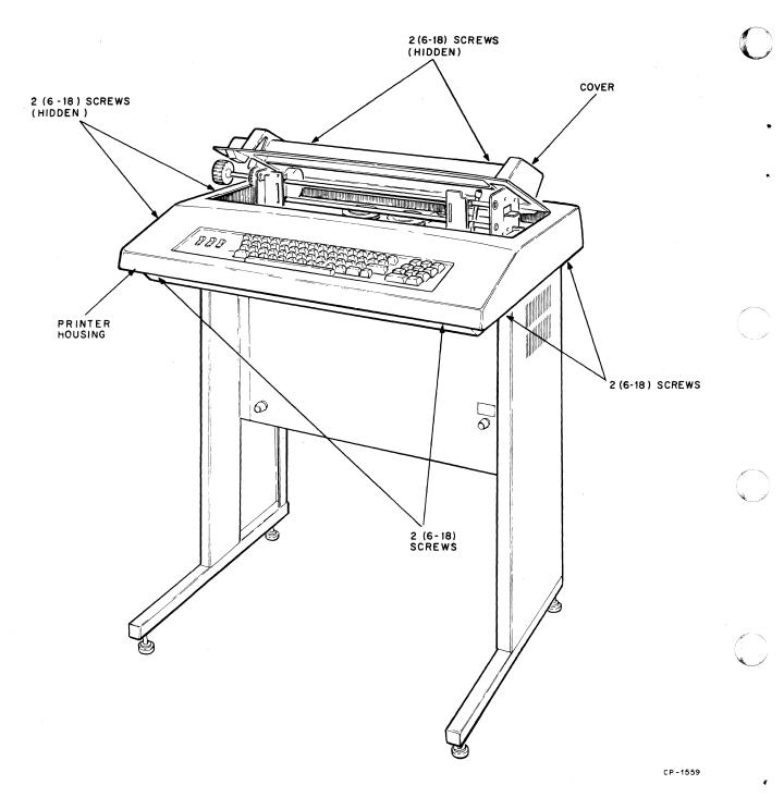
Figure 7-11 Remove Printer Housing
