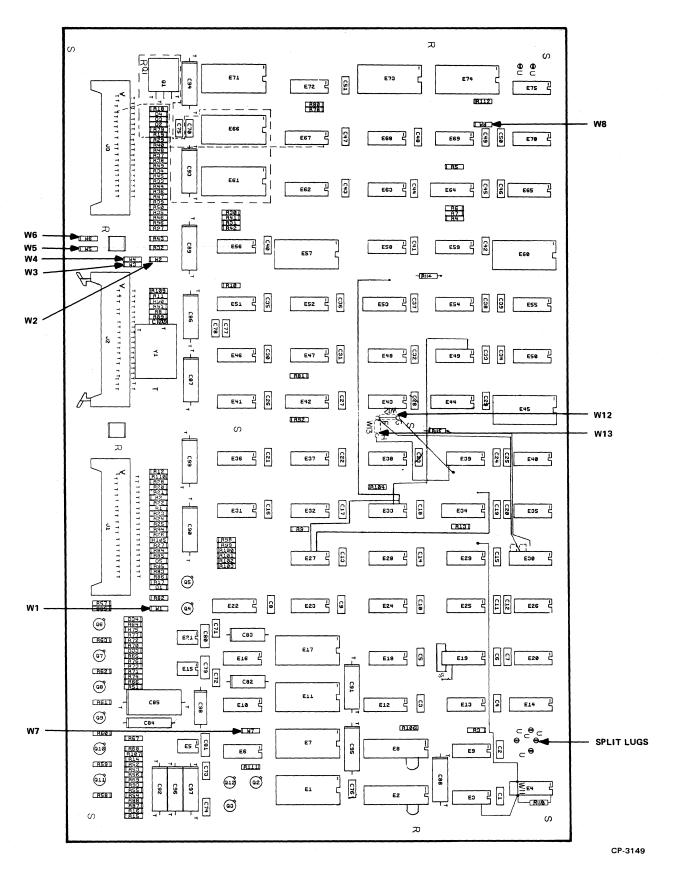
Figure 3-6 Printer Board Jumper Locations
