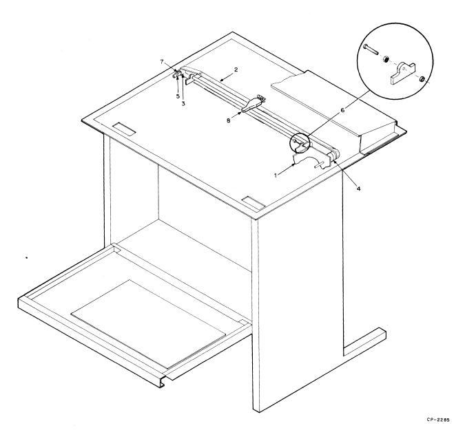
Figure 7-13 Installation of Compressed Font Option Kit
