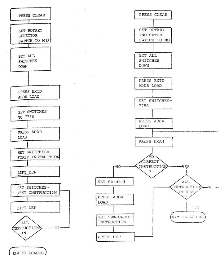
Figure 2-3 Checking the RIM Loader
