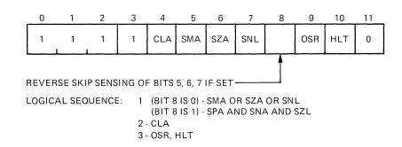
Figure 3 Group 2 Operate Microinstruction Bit Assignments
