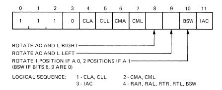
Figure 2 Group 1 Operate Microinstruction Bit Assignments
