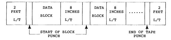
Leader trailer is any string of 0 or 200 punches; usually it is just 200 punches; leader trailer is terminated by a 201 punch, which indicates the start of a data block. The first punch after the last data block is 377, which is end of tape. Each data block has the following format:
