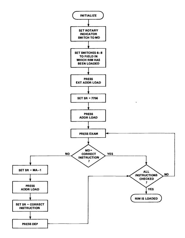
Figure B-2 Checking the RIM Loader
