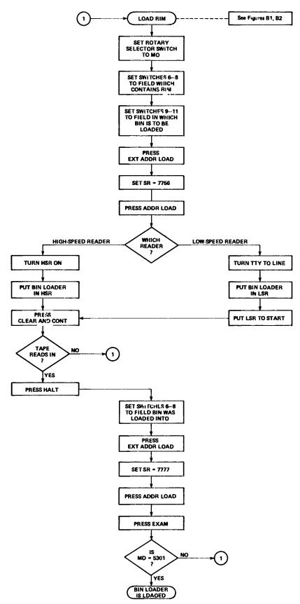
Figure B-3 Loading the BIN Loader
