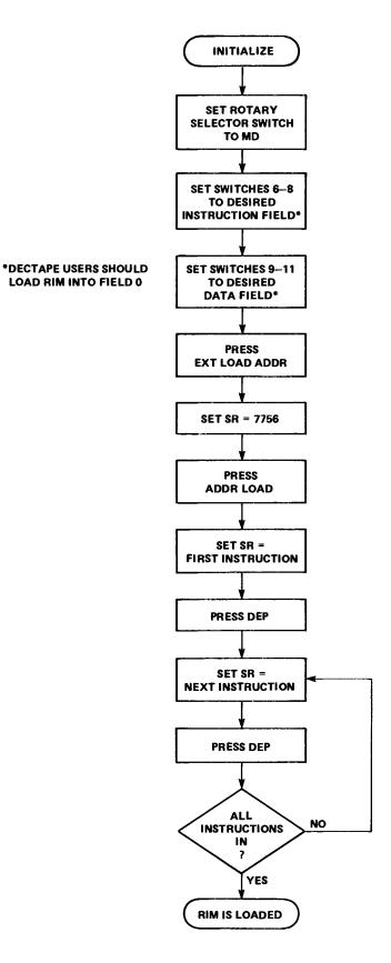
Figure B-1 Loading the RIM Loader
