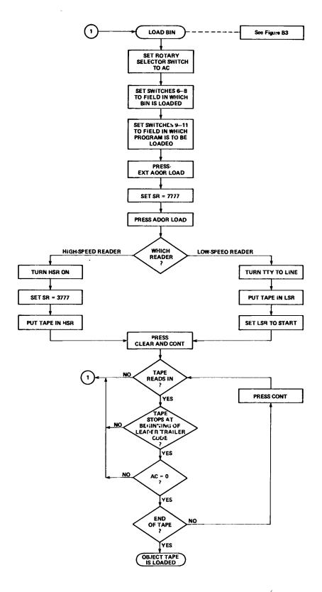
Figure B-4 Loading a Binary Tape Using BIN
