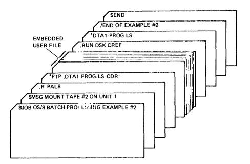
Figure 6-2 Punched Card Input File
