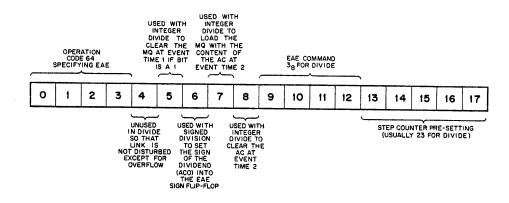
Figure 21 EAE Divide Instruction Bit Assignments
