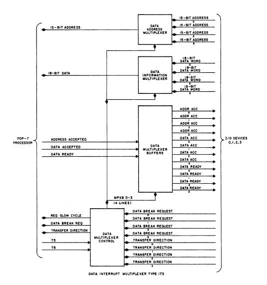
Figure 28 Data Interrupt Multiplexer Type 173
