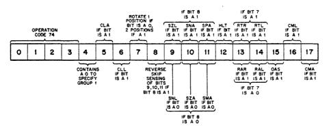
Figure 14 Group 1 Operate Instruction Bit Assignments
