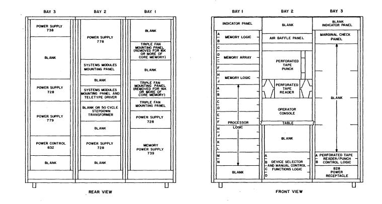
Figure 2 Basic PDP-7 Component Locations
