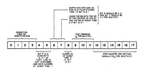
Figure 20 EAE Multiply Instruction Bit Assignments
