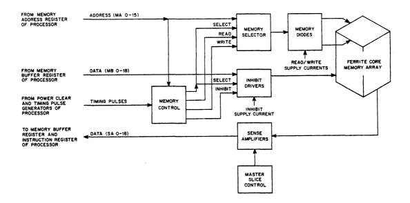
Figure 7 Core Memory Block Diagram
