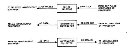
Figure 8 Interface Block Diagram
