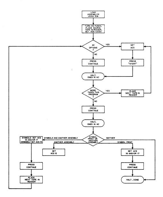
Figure 38 Assembler Flow Diagram
