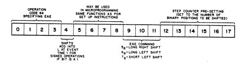
Figure 23 EAE Shift Instruction Bit Assignments
