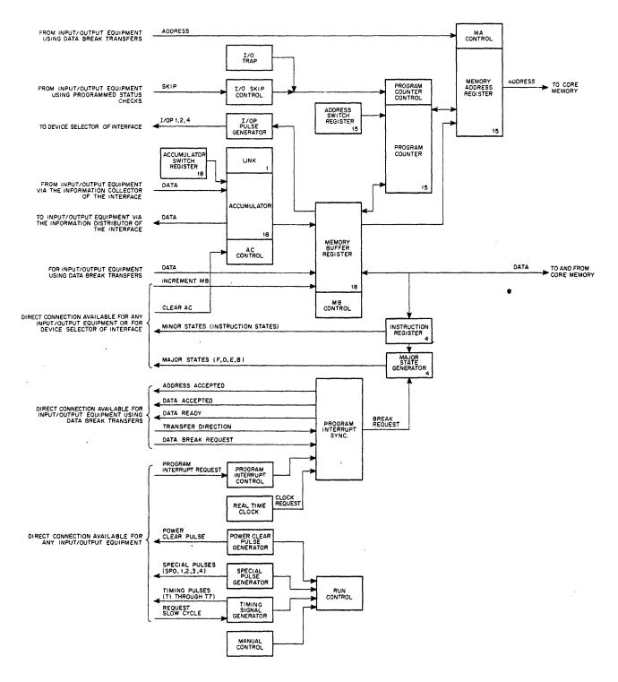
Figure 6 Detailed Block Diagram of the Processor
