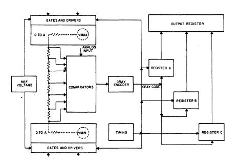
Figure 35 Type 142 A-to-D Converter, Block Diagram
