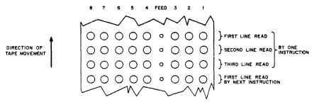
Figure 30 Tape Format and Reader Buffer Register Bit Assignments In Binary Mode
