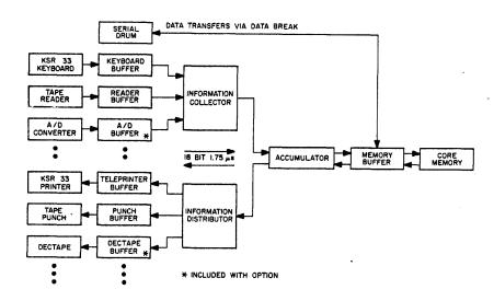
Figure 11 Input/Output Information Flow
