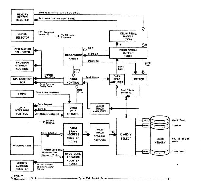
Figure 34 Serial Drum Block Diagram and Interface Connections
