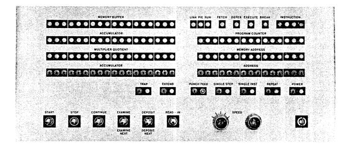
Figure 36 Operator Console
