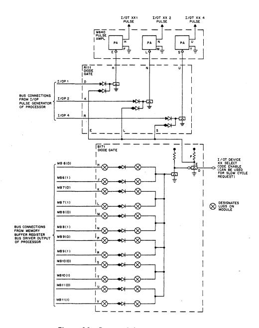
Figure 10 Device Selector Logic Diagram
