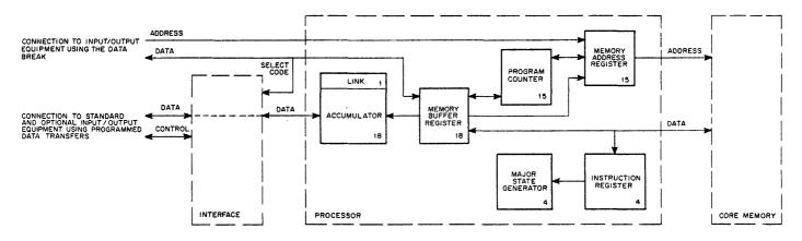
Figure 5 Major Register Block Diagram of the Processor
