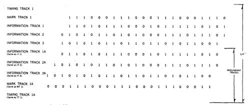
Track Allocation Showing Redundantly Paired Tracks
