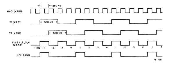
Figure 4-1 Basic I/O Timing
