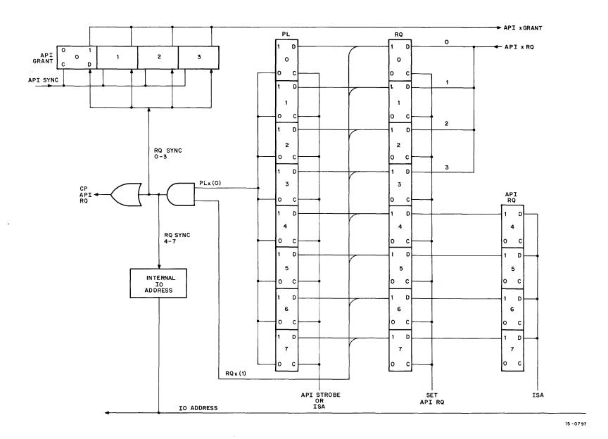
Figure 6-10 API Block Diagram
