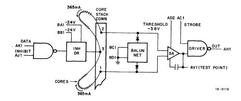
Figure 2-2 Sense Amplifier/Inhibit Driver, Simplified Diagram
