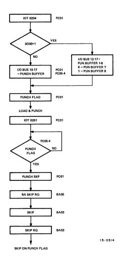
Figure 6–18 High-Speed Punch Operation, Flow Diagram
