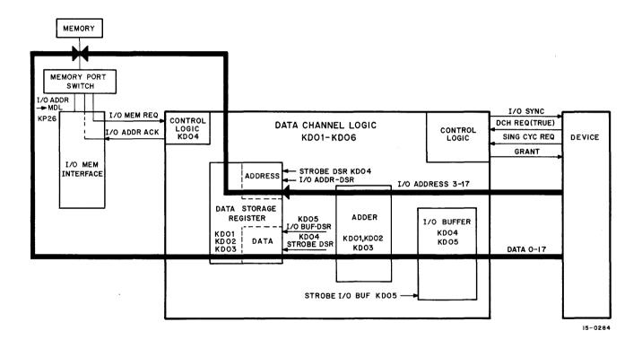
Figure 4-9 Single Cycle Data In Transfer, Block Diagram
