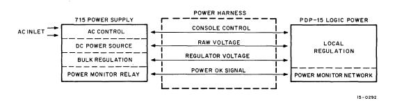
Figure 5-1 Power Distribution Block Diagram
