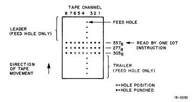
Figure 6–15 Tape Format and Accumulator Bits (Alphanumeric Mode)
