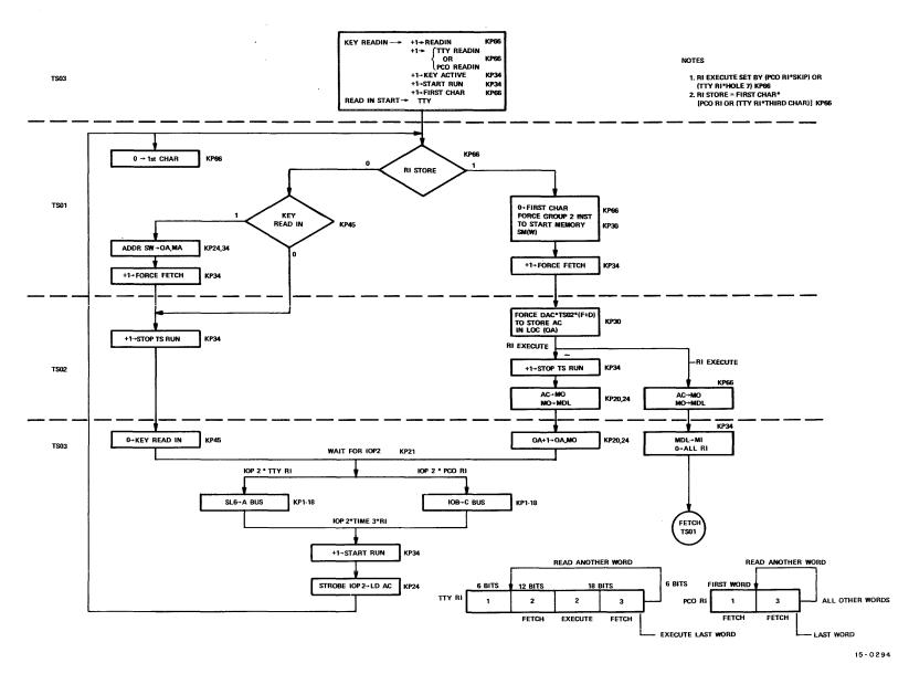
Figure 3-4 Read-In Flow Diagram
