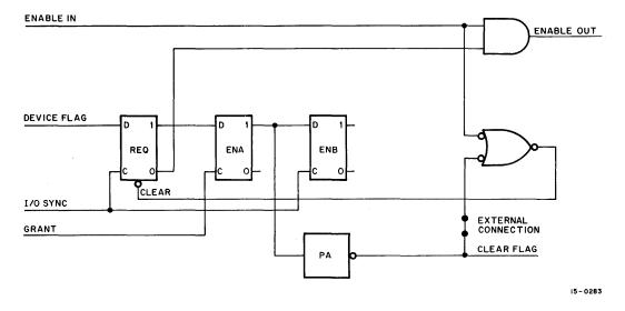
Figure 4-7 Simplified M104 Module Diagram
