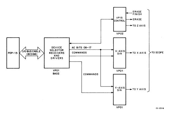
Figure 6-21 VP15 Controller, Simplified Block Diagram
