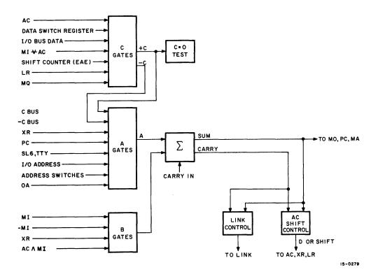
Figure 3-1 CPU Bus Structure
