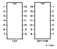
Figure 7-2 Integrated Circuit Pin Location
