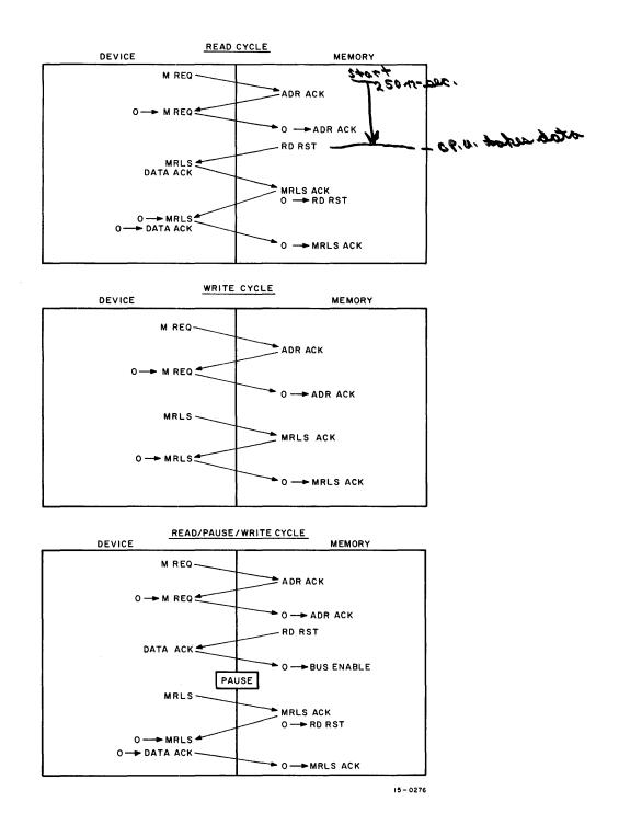
Figure 2-4 Basic Device-Memory Control Signal Flow
