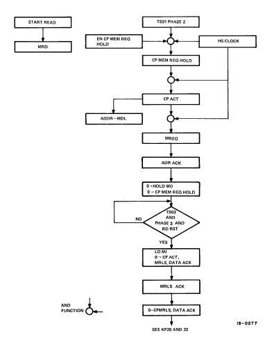
Figure 2-6 Central Processor Read Cycle
