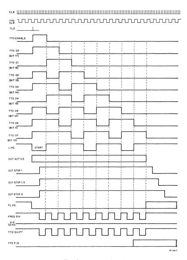
Figure 6-20 Teletype Transmitter (Printer) Timing
