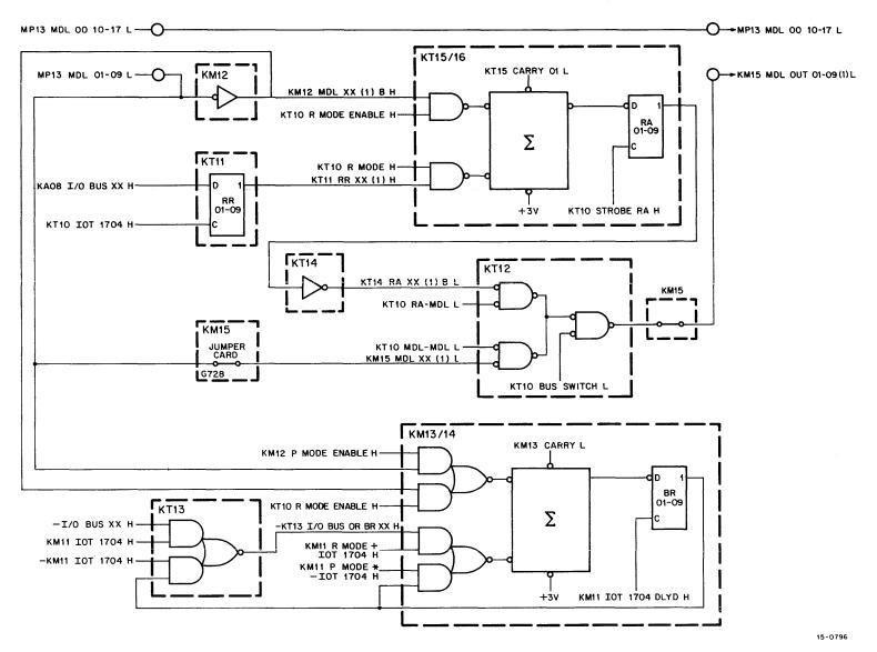
Figure 6-14 Memory Protect and Relocate Interconnection Diagram
