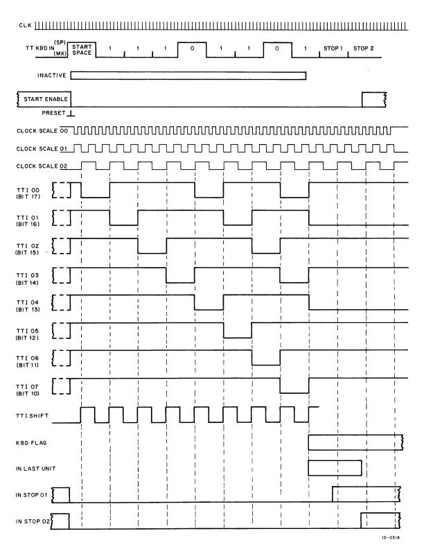
Figure 6-19 Teletype Receiver (Keyboard) Timing
