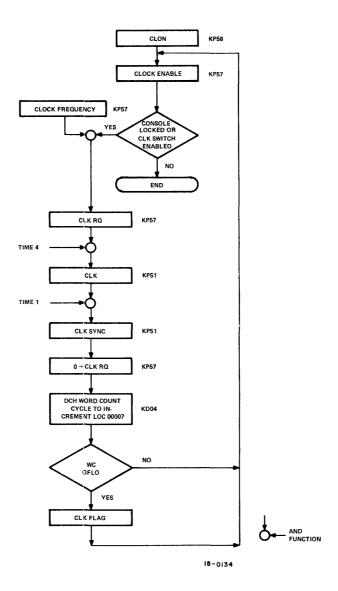
Figure 6-4 Real-Time Clock, General Flow Diagram
