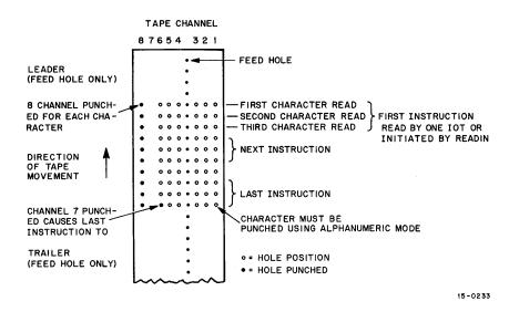
Figure 6–16 HRI Tape Format and Accumulator Bits (Binary Mode)
