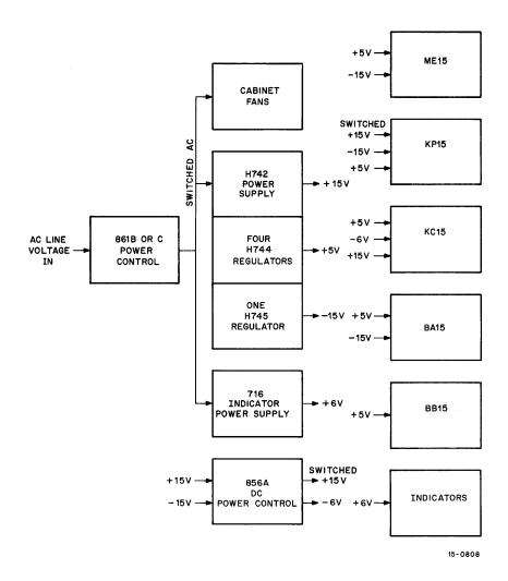
Figure 5-2 PDP-15/C Power Distribution Block Diagram
