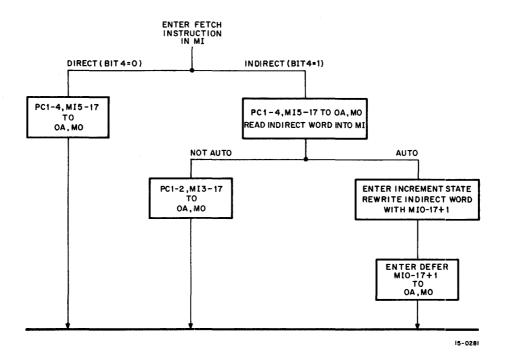
Figure 3-3 Bank (PDP-9) Mode Address Formation
