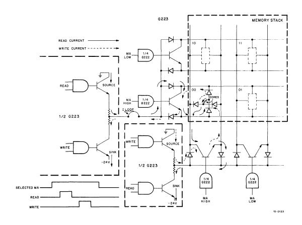
Figure 2-1 Current Path Diagram
