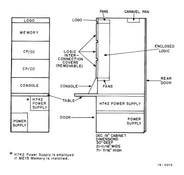
Figure 1-3 PDP-15/10 System Configuration Diagram
