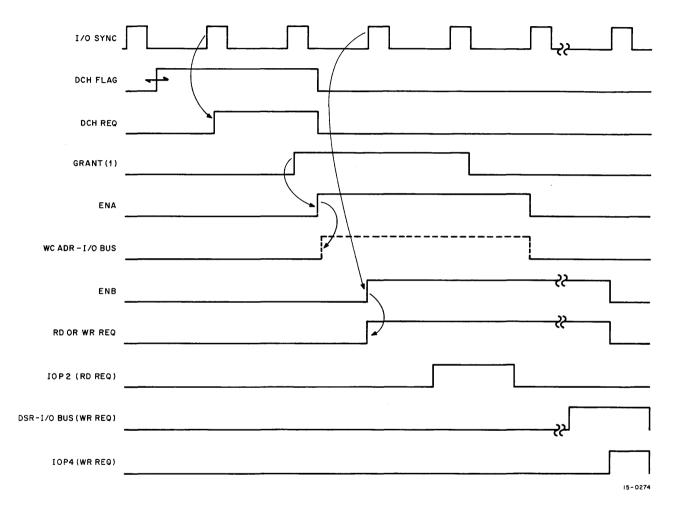
Figure 4–14 Multicycle Timing Diagram
