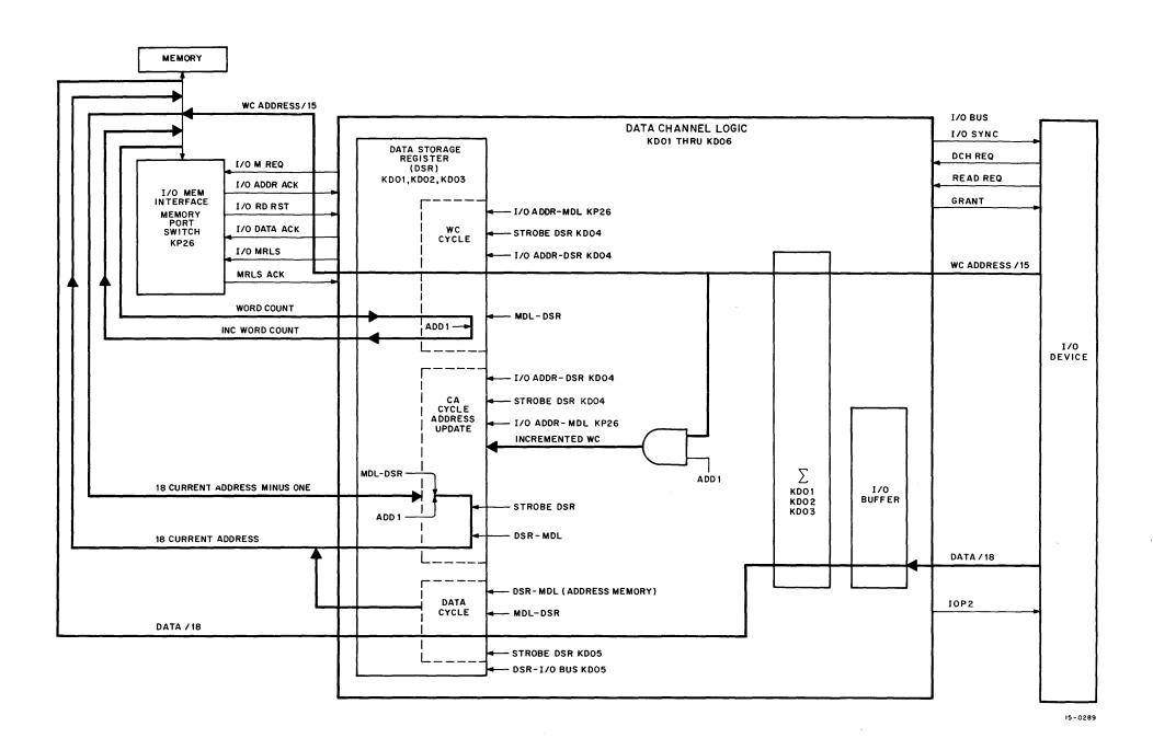
Figure 4-13 Multicycle Data In Transfer Block Diagram
