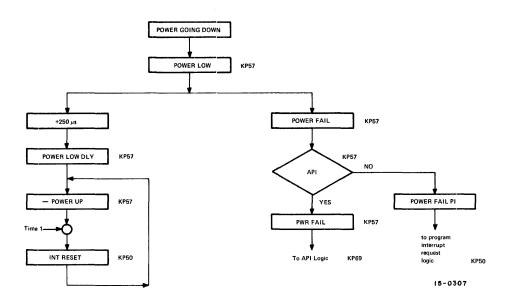
Figure 6-7 Power Fail Sequence With Power Fail Option Enabled, Flow Diagram
