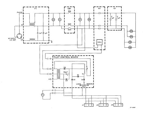
Figure 5-4 861C Power Controller Schematic
