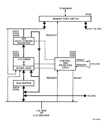
Figure 4-6 Data Channel Block Diagram
