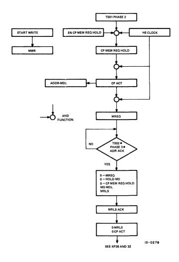
Figure 2-7 Central Processor Write Cycle
