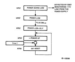
Figure 6-5 Power Fail Sequence With Power Fail Option Disabled, Flow Diagram
