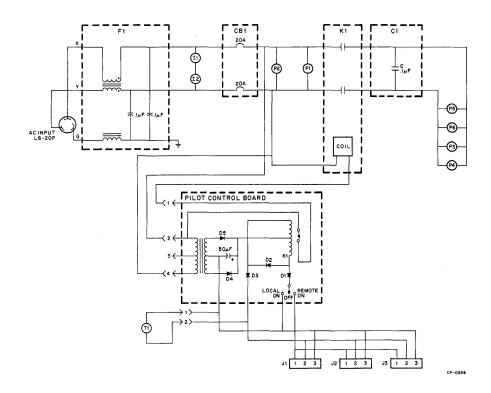
Figure 5-3 861B Power Controller Schematic
