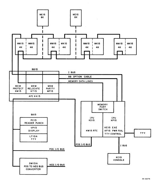
Figure 1-2 PDP-15 System Block Diagram
