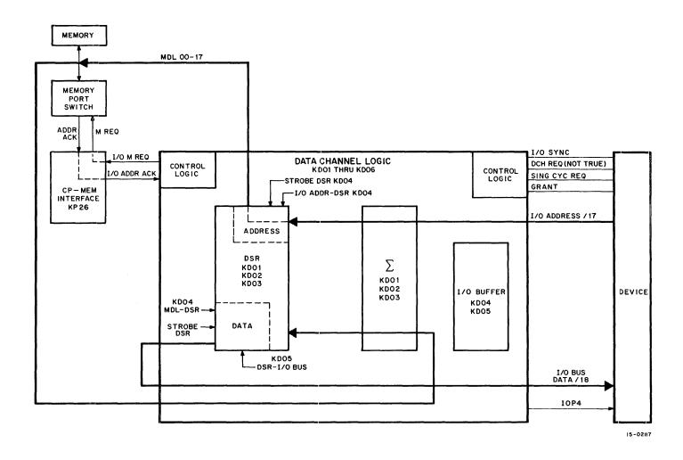
Figure 4-11 Single Cycle Data Out Transfer, Block Diagram
