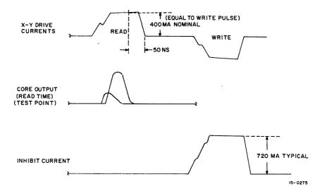
Figure 2-3 Typical Inhibit Current Waveforms
