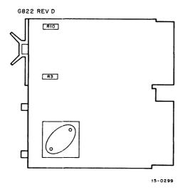
Figure 7-4 G822 Module Adjustment Locations
