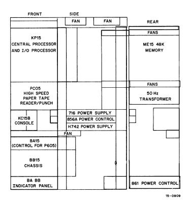
Figure 1-7 PDP-15/C System Configuration Diagram
