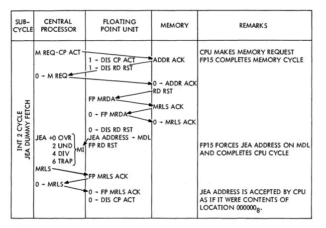
Figure 3-6 INT 2 Cycle Interface Diagram
