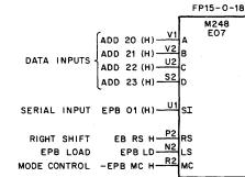
Figure 2-5 M248 Right-Shift Parallel Load Register
