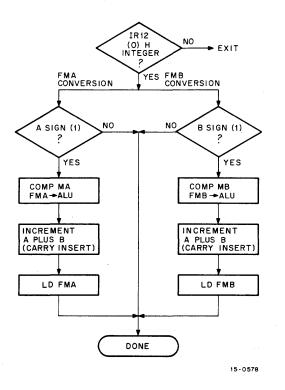
In EXP\*TS02, INCB is generated which puts the contents of the FMB plus one on the ALU bus. This number is strobed back to the FMB during PH03\*TS02. The number now in the FMB is the 2's complement of the number originally contained there and is a negative number in sign and magnitude format.
