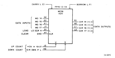
Figure 2-1 M238 Synchronous Up/Down Counter
