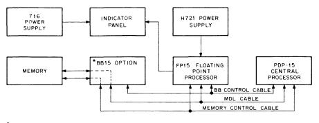
\*If BB option is not installed, cables are directly routed to memory.
