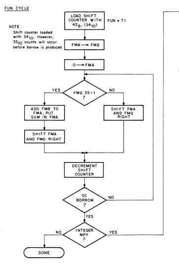
Figure 4-4 Multiply Simplified Flow Diagram
