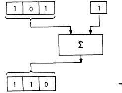
Figure 4-2 Guard Bit and Rounding
