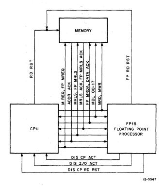
Figure 3-1 Major Signal Interface Diagram
