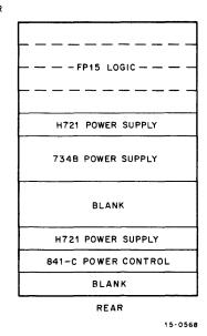
Figure 1-1 Cabinet Housing FP15 Logic
