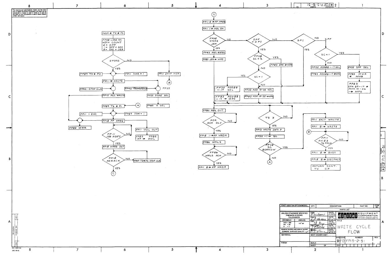
represents the 2's complement of the FMA. During the WRITE cycle, A SIGN is examined. If it is positive, the contents of the FMA are stored in memory; if it is negative, the 2's complement of the negative integer are stored in memory. This 2's complement is contained in the FMB and, consequently, the contents of the FMB are stored in memory.
