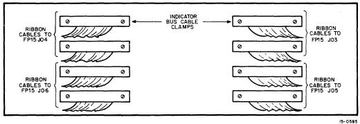
Figure 5-2 FP15 Indicator Bus Connections
