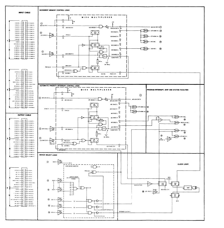
Figure 4-9 Increment Memory Device Logic
