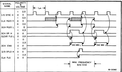
Figure 4-10 Timing Diagram for Increment Memory Devices
