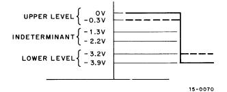
Figure 2-1 Voltage Spectrum of Negative Logic Systems
