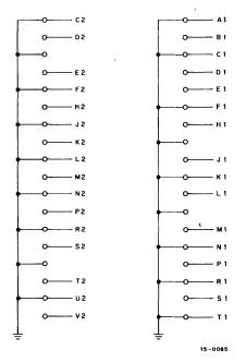
Figure 6-6 M912 PDP-15 I/O Bus Card
