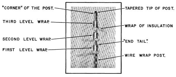
THE CONNECTOR BLOCK AND OTHER POSTS HAVE BEEN ELIMINATED FROM THE PICTURE FOR CLARITY.
