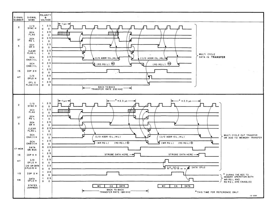
Figure 4-7 Multi-Cycle Data Channel Timing
