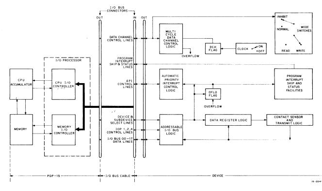
Figure 4-5 Block Diagram for Multicycle Data Channel Device
