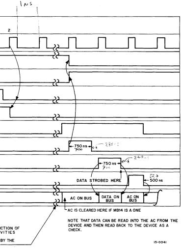
Figure 4-4 Timing Diagram of the CPU Device with API
