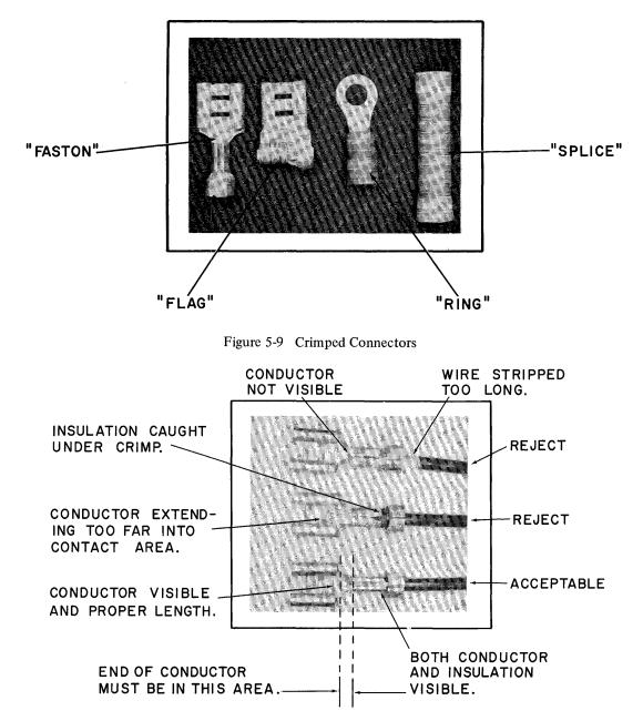
Figure 5-10 Acceptable and Unacceptable Crimped Connections
