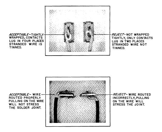
Figure 5-15 Example of Wire Joint Before Soldering
