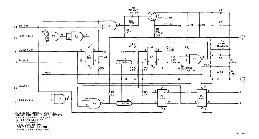
Figure 2-6 M104 Circuit Schematic
