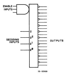
Figure 1-14 Binary to Decimal Decoder
