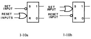
Figure 1-10 R-S Flip-Flop
