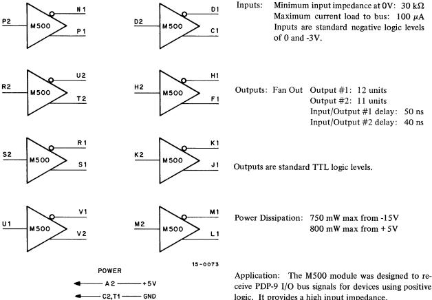
Figure 2-8 M500 Receiver Module
