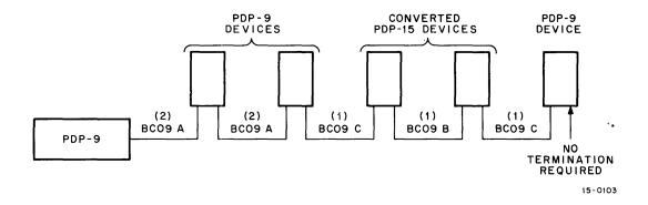
Figure 6-9 Cabling Converted PDP-15 Devices to the PDP-9 I/O Bus
