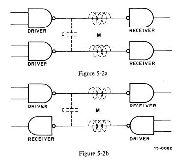
Figure 5-2 Capacitance and Inductive Crosstalk Components
