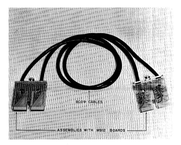
Figure 6-5 BC09B Cable Assembly
