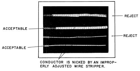
Figure 5-8 Stripping Damage
