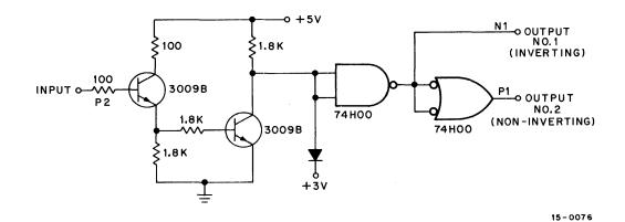
Figure 2-11 M510 Schematic
