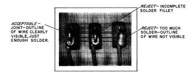
REJECT-INSUFFIENT SOLDER-CAUSED BY USING TOO SMALL A SOLDERING IRON ON A LARGE (#10) WIRE.
