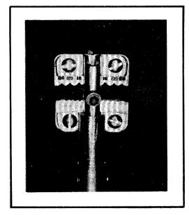
Figure 5-6 Non Adjustable Wire Stripper
