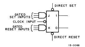
Figure 1-9 J-K Master-Slave Flip-Flop
