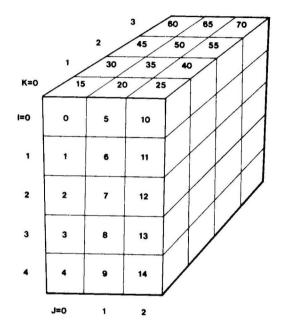
This rectangular solid has dimensions of five rows, three columns, and four planes; thus, IMAX=5, JMAX=3, and KMAX=4. Each plane is numbered exactly as in the 2-dimensional example, except 15 times K (with K = the number of planes back from the first) is added to each subscript in the first plane.
