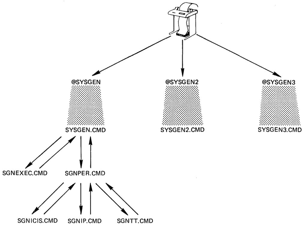
Figure 1-2 SYSGEN Command Files and How They Interrelate
