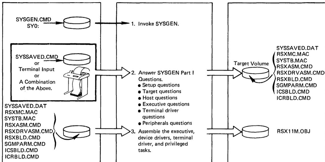
Figure 5-1 Processing Steps in SYSGEN Phase I
