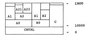
As a single-segment task, TKl required 24200 bytes of storage. The first overlay structure reduced the requirement by 6200 bytes. The second overlay structure further reduced the storage requirement by 2200 bytes.
