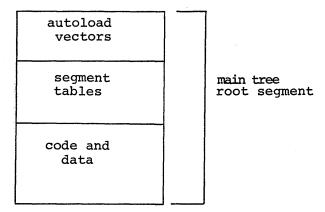
The segment table contains a segment descriptor for every segment in the task. The descriptor contains information about the load address, the length of the segment, and the tree linkages. The segment table is described in detail in Appendix C.
