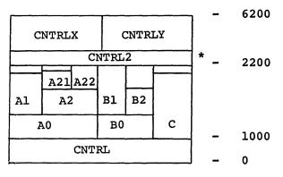
The specification of the co-tree decreases the storage allocation by 4000 bytes. CNTRLX and CNTRLY can still access modules on all the paths of the main tree. The only requirement imposed by the introduction of the co-tree is the logical independence of CNTRLX and CNTRLY.
