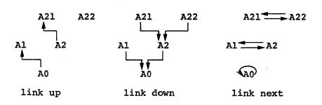
If there is a co-tree, the link next of the segment descriptor for the root points to the segment descriptor for the root segment of the co-tree.
