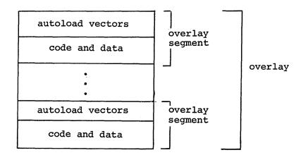
The co-tree overlay region consists of memory allocated for the overlay segments of the co-trees.
