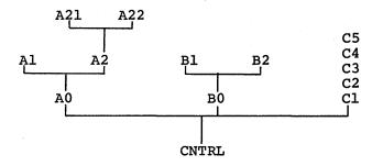
If CNTRL calls A2, then all the modules between the calling module CNTRL and the called module A2 are loaded. In this case modules A0 and A2 are loaded.
