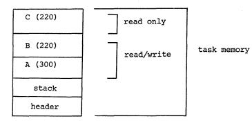
4.1.2.1 Sequential Allocation of P-sections - The SQ (sequential) switch affects only the placement of p-sections in task memory. P-sections with the same name and attributes are collected as described; then uniquely named p-sections are placed in memory in the order of input sequence according to the access-code.
