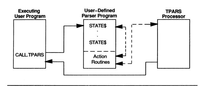
Figure 7–2 Flow of Control When TPARS is Called from an Executing User Program
