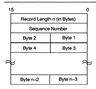
Figure 1–2 Sequenced Variable-Length Record
