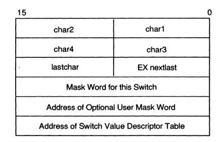
Figure 6–2 Format of Switch Descriptor Table Entry
