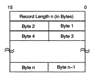
Figure 1–3 Nonsequenced Variable-Length Record
