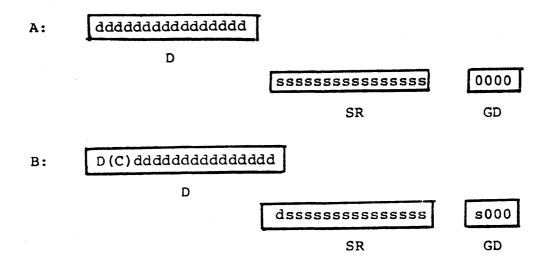
Figure 2-30: Right Shift on 32 Bits of Data
