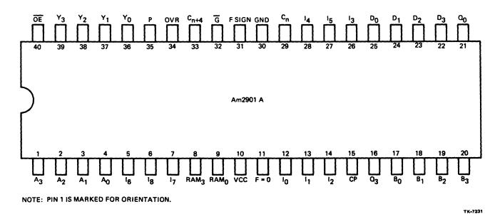
Figure 4-3 AM2901A Pin Connections
