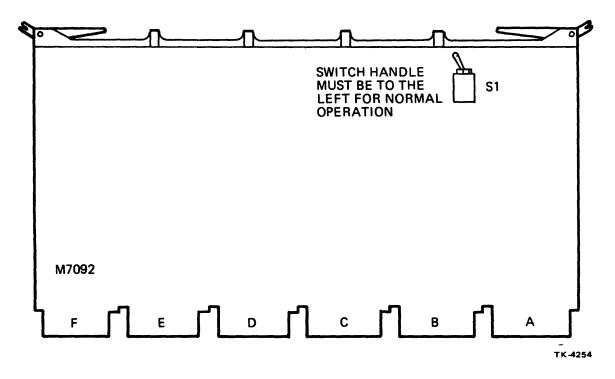
Figure 6-2 KE44-A Data Path/Logic Module, M7092
