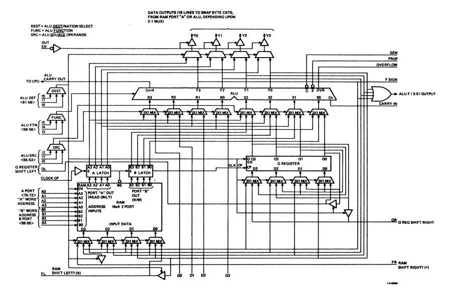
Figure 4-2 2901A Detailed Block Diagram
