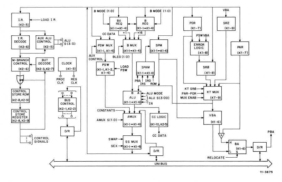
Figure 4-1 KD11-E Block Diagram
