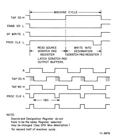
Figure 4-4 Scratchpad Timing
