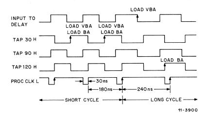
Figure 4-17 Processor Clock Cycle Timing
