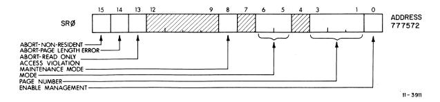
Figure 4-40 Format of Status Register 0 (SR0)
