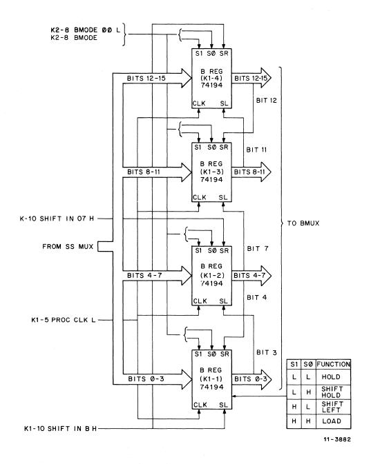
Figure 4-7 BREG Block Diagram
