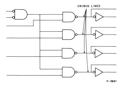
Figure 4-16 Unibus Transceiver
