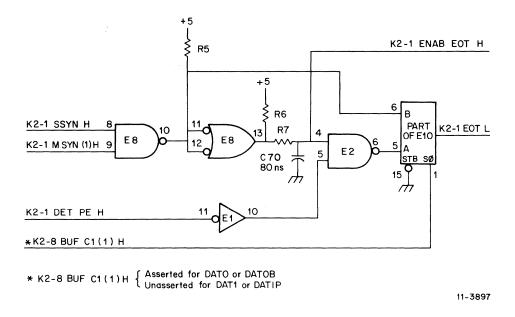
Figure 4-24 End-of-Transfer Logic
