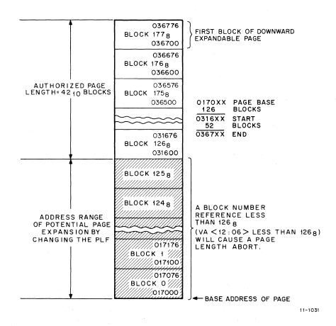
Figure 4-36 Example of a Downward-Expandable Page
