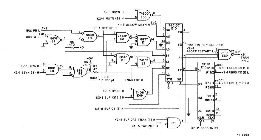
Figure 4-22 Data Transfer Multiplexer
