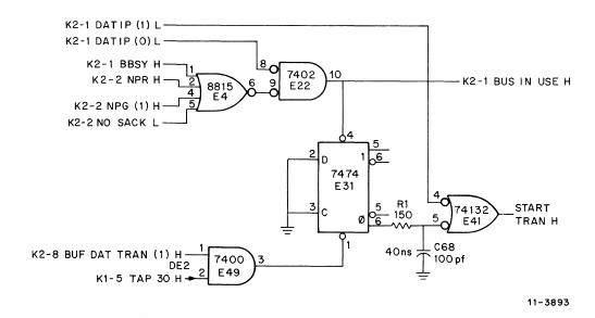
Figure 4-19 Unibus Synchronizer
