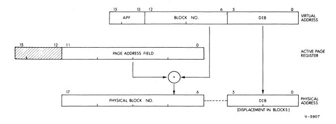
Figure 4-39 Construction of a Physical Address
