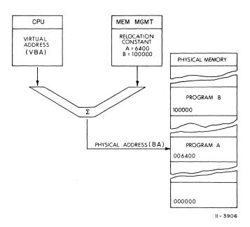
Figure 4-31 Simplified Memory Relocation Example
