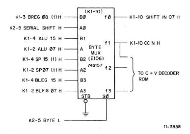
Figure 4-13 Byte Multiplexer
