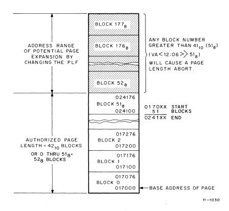
Figure 4-35 Example of an Upward-Expandable Page
