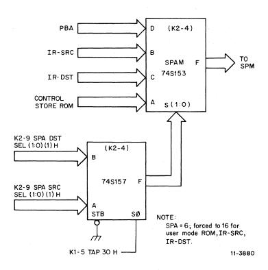
Figure 4-5 Scratchpad Address Multiplexer (SPAM)
