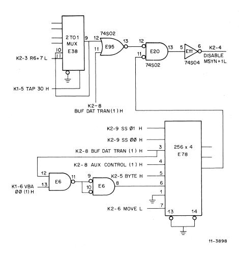
Figure 4-25 Odd Address Detection
