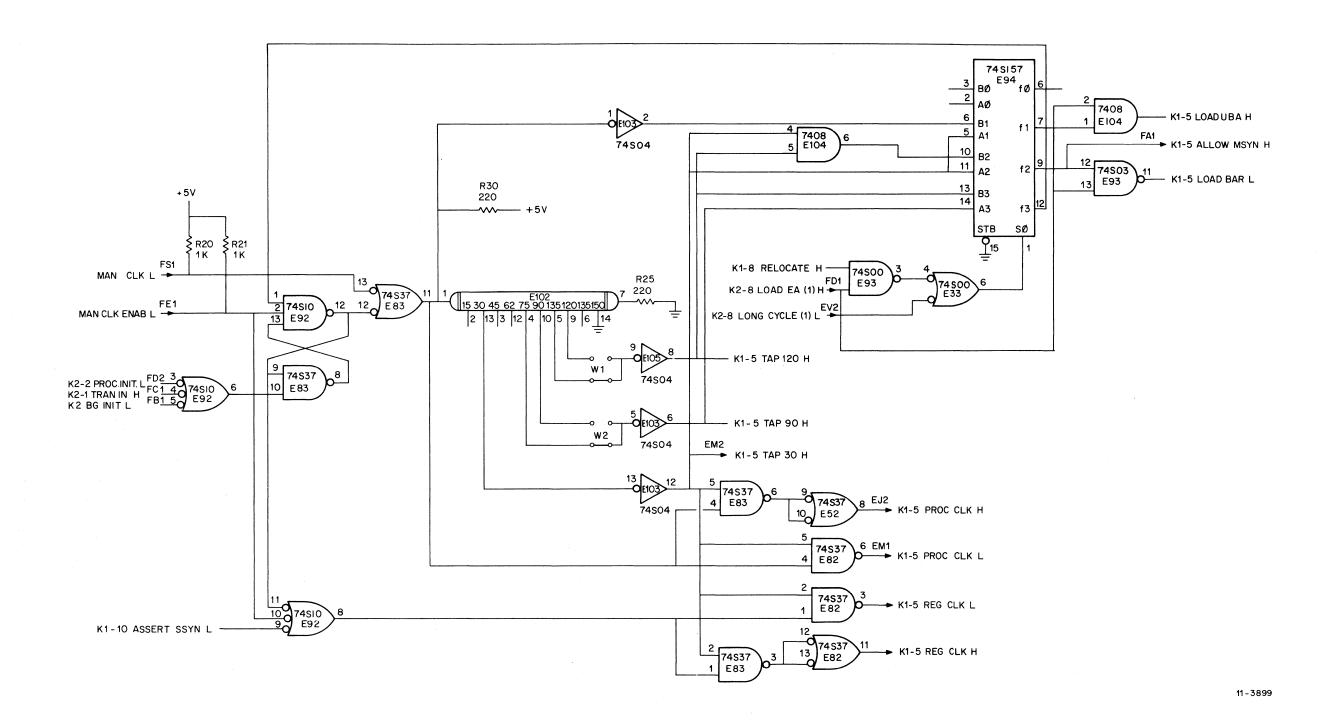
Figure 4-27 Processor Clock Circuit
