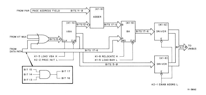
Figure 4-18 Unibus Address Logic Block Diagram
