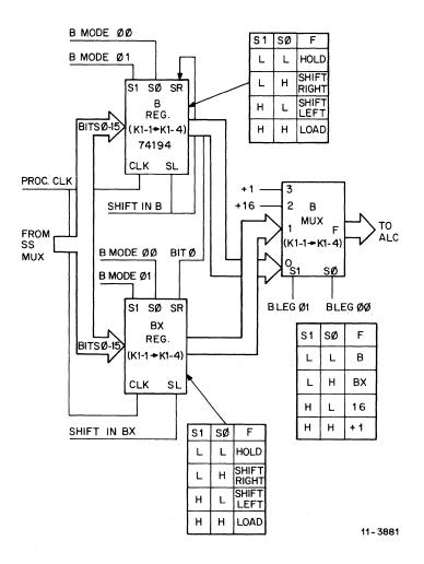
Figure 4-6 B Leg Block Diagram
