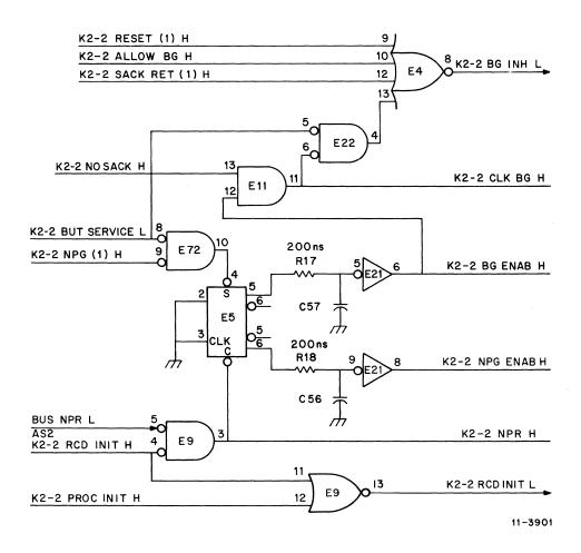
Figure 4-28 Priority Arbitration Synchronizer
