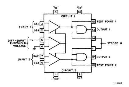
Figure 4-21 Type 7528 Dual Sense Amplifier with Preamplifier Test Points
