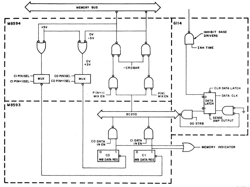
Figure 4-5 Data Path Diagram
