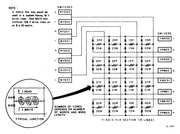
Figure 4-15 Simplified Y Line Selection Stack Diode Matrix
