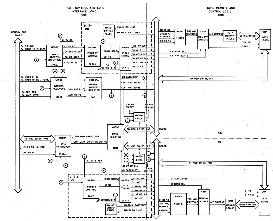
Figure 4-2 MG10 Block Diagram
