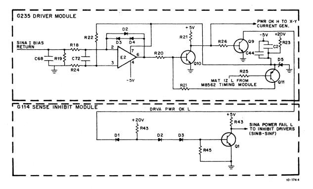
Figure 4-23 DC LO and Bias Current Detection Circuit
