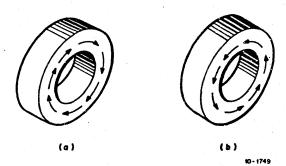
Figure 4-8 Magnetic States of Ferrite Cores
