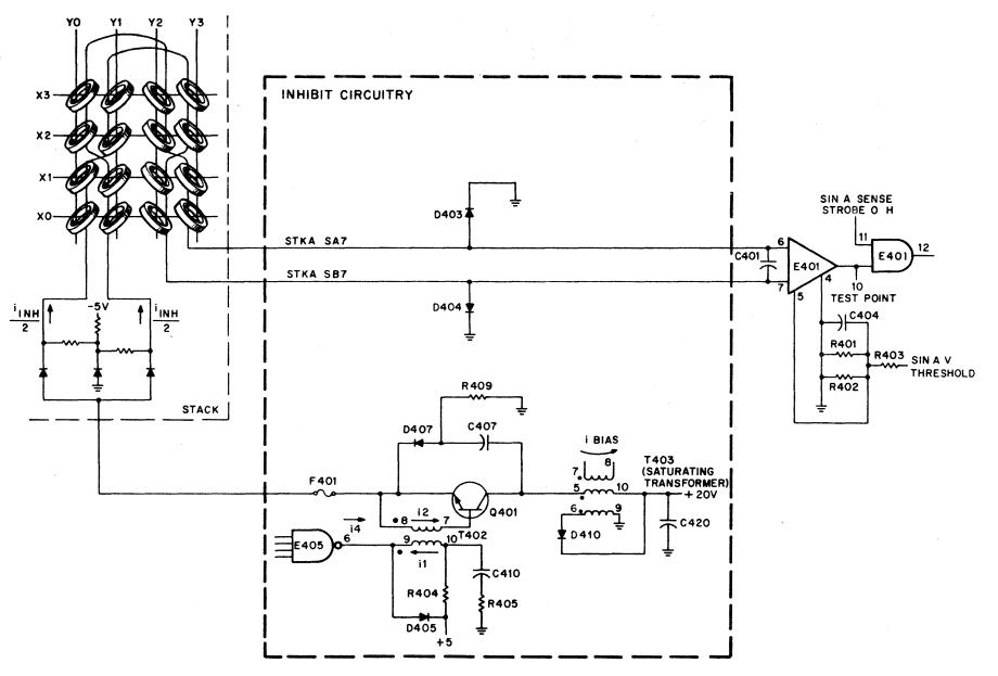
Figure 4-20 Sense Amplifier and Inhibit Driver
