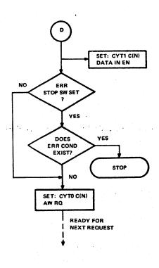
Figure 4-7 Read Restore Timing Flow Diagram
