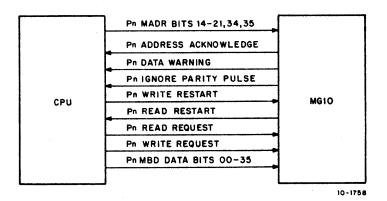
Figure 4-1 Memory Processor Interface
