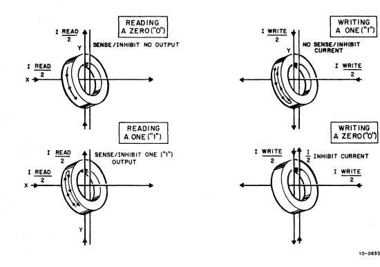
Figure 4-10 3-D, 3-Wire Core States
