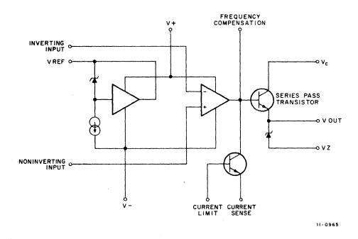
Figure 4-24 Voltage Regulator El, Simplified Diagram
