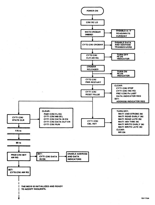
Figure 4-4 MG10 Power-Up Flow Diagram
