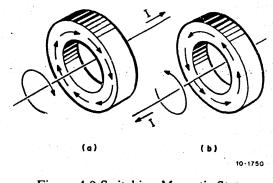
Figure 4-9 Switching Magnetic State of Ferrite Cores
