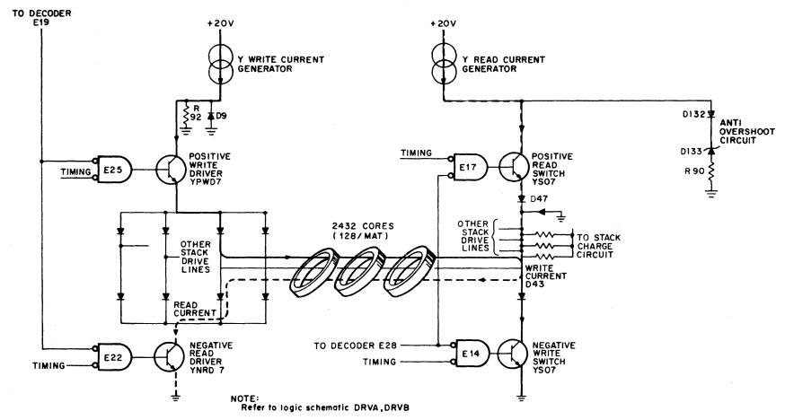
Figure 4-16 Typical Y Line Read Write Switches and Drivers
