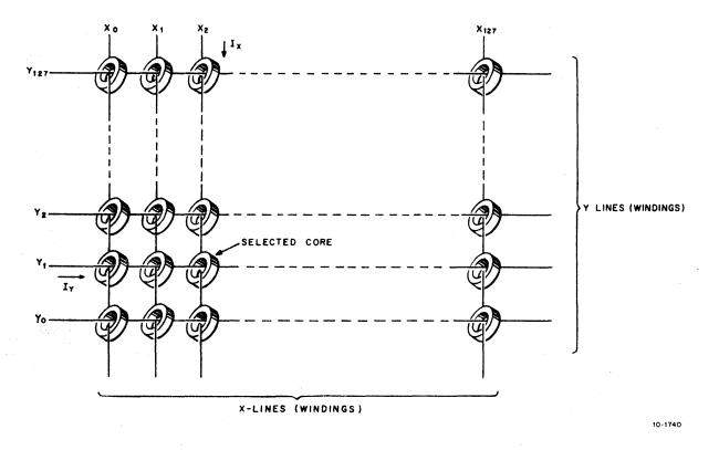
Figure 4-11 Core Configuration in a  $128 \times 128$  Mat
