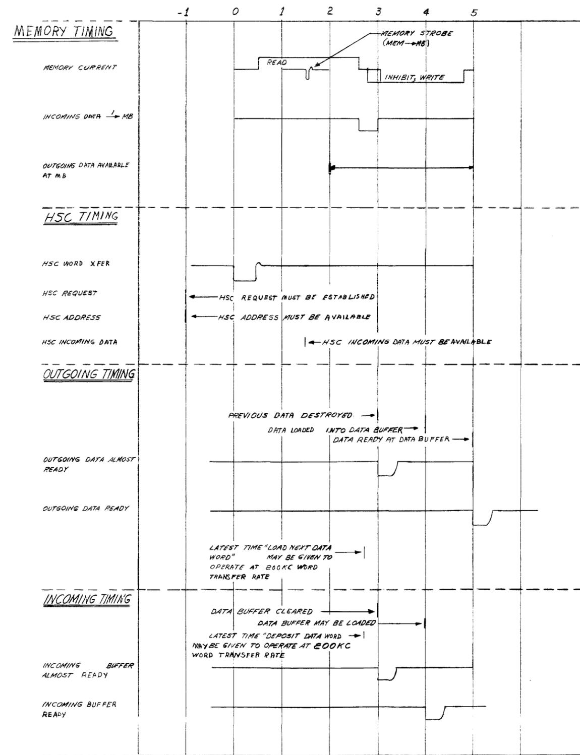
Figure 6-12 Data Channel Type 123, Logical Organization and Timing
