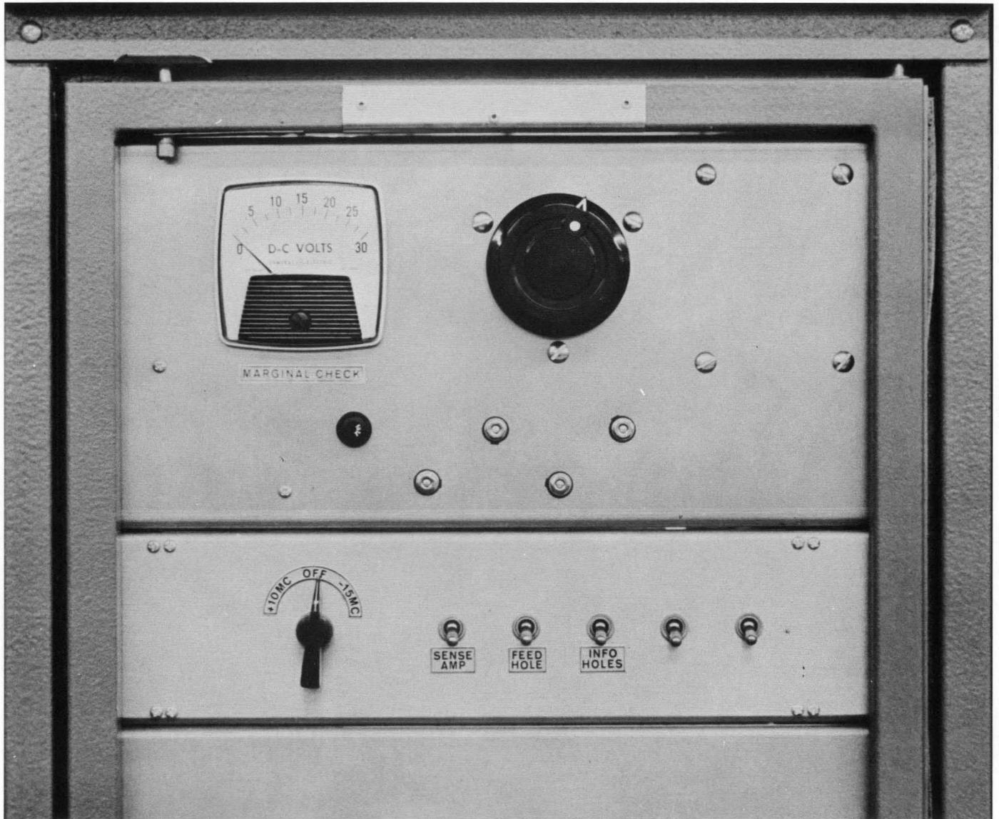
Figure 5-5 Variable Power Supply Type 734 and Marginal Check Switch Panel
