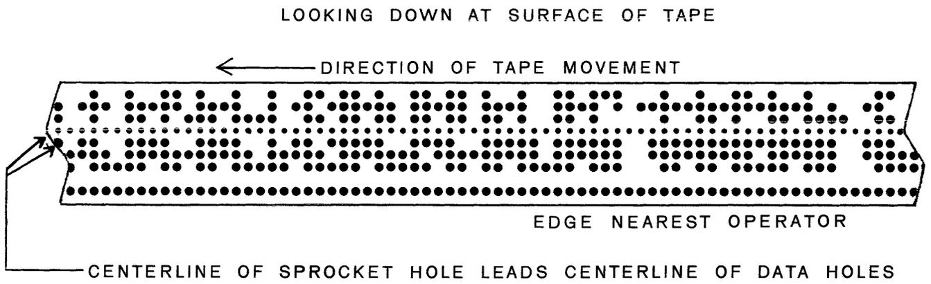
Figure 11-8 Correct Orientation for Loading Paper Tape
