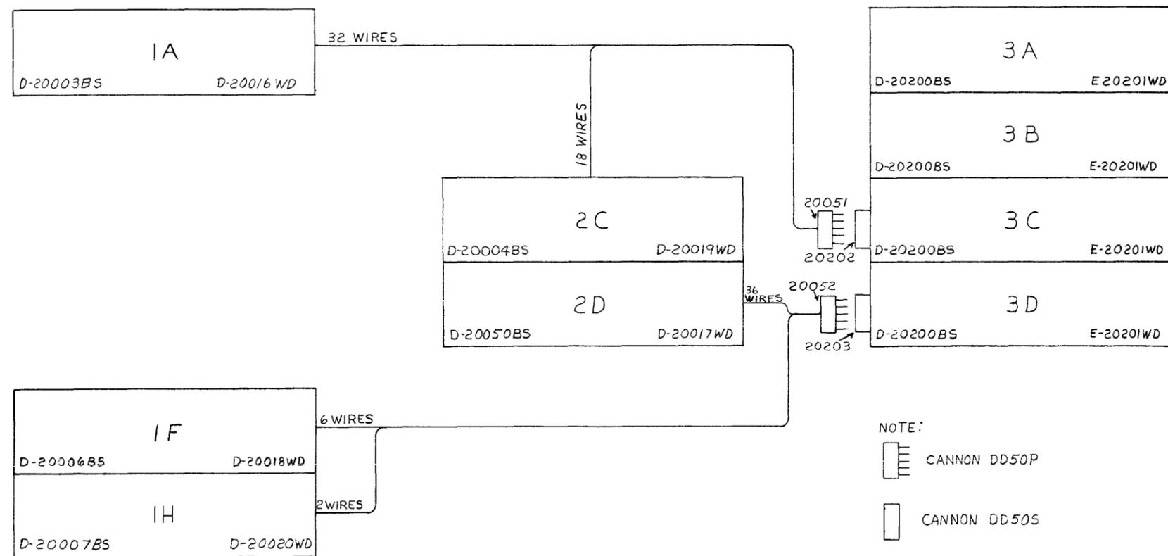
Figure 11-4 Standard Wiring Configuration for One Memory
