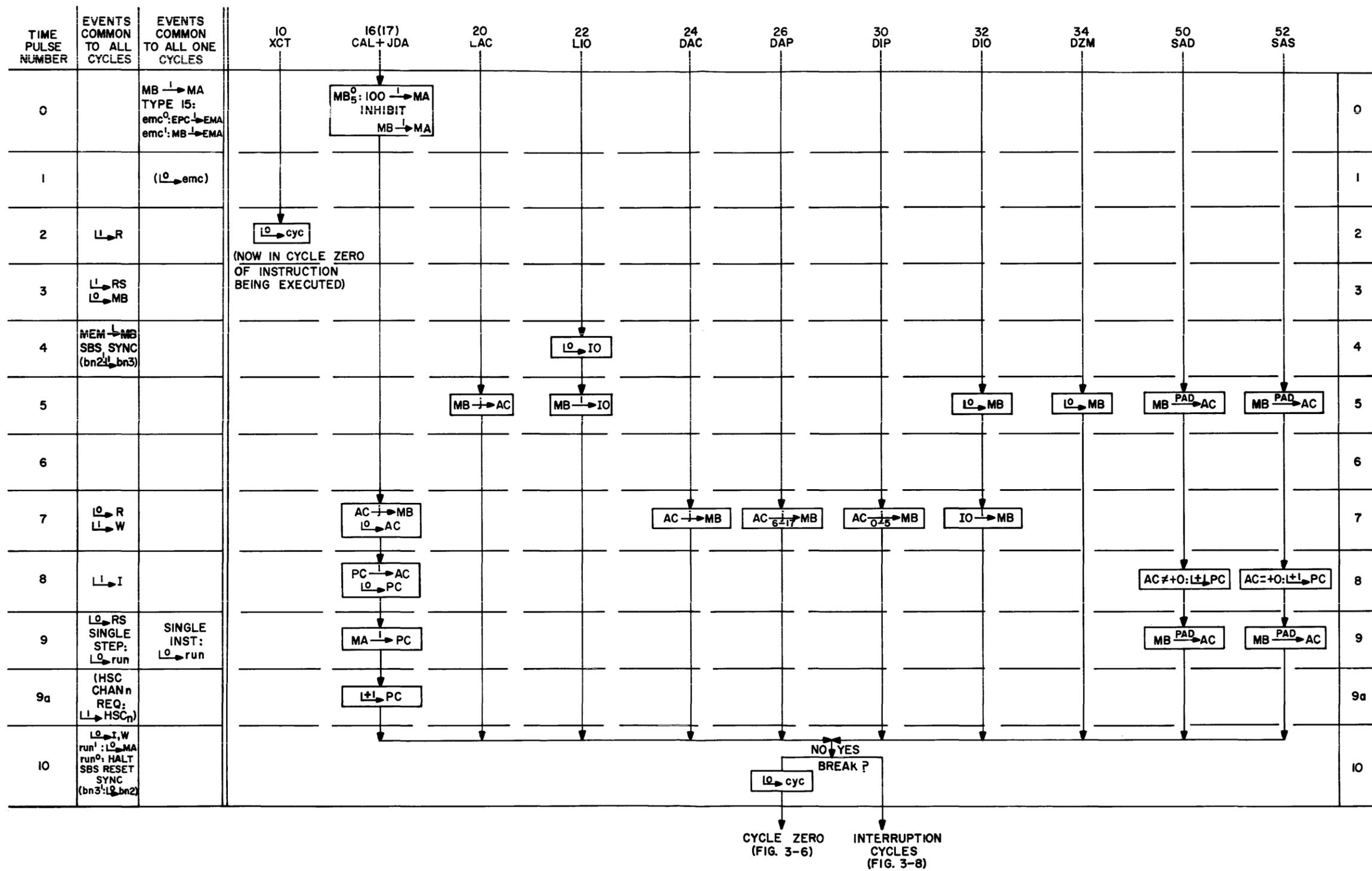
Figure 3-10 Flow Chart: Cycle One, Data Handling and Program Control Instructions
