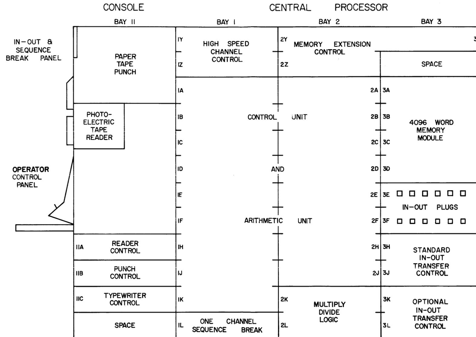
Figure 2-7 Logic Layout, Control Frame
