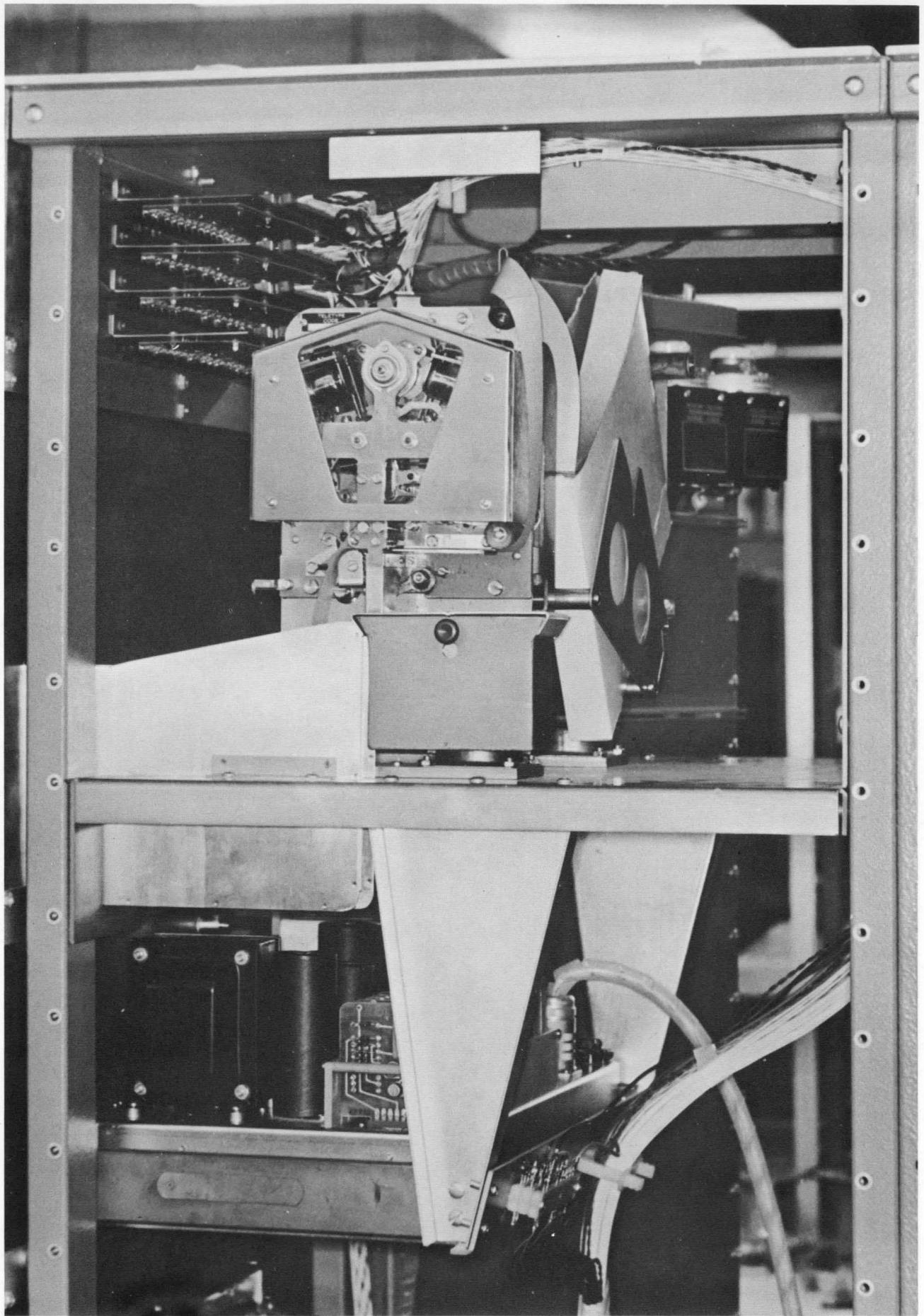
Figure 5-8 Paper Tape Punch, Front View
