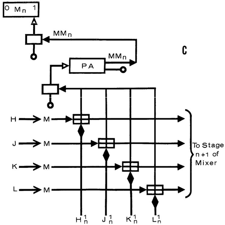
Figure 3-4 Transfer Logic
