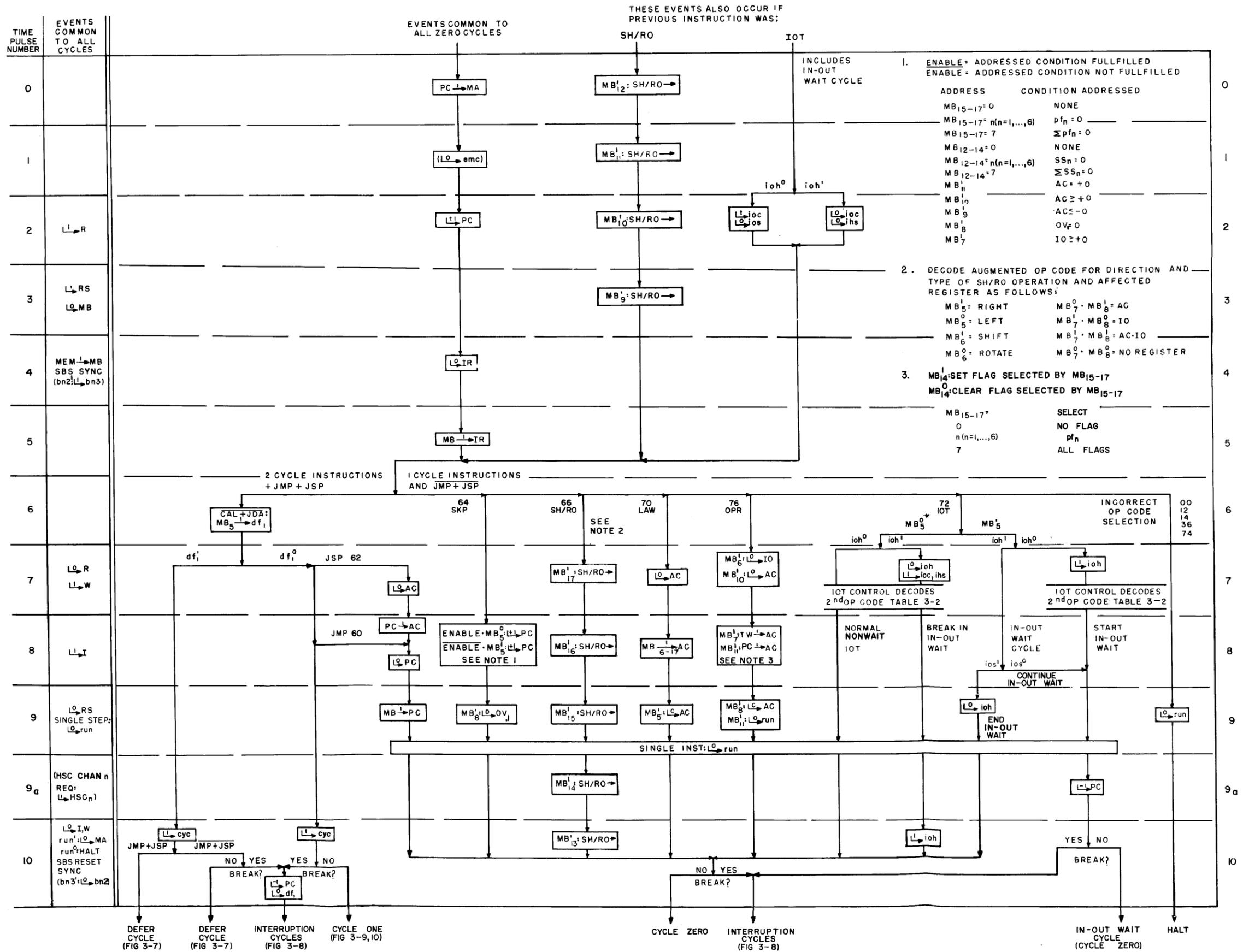
Figure 3-6 Flow Chart, Cycle Zero
