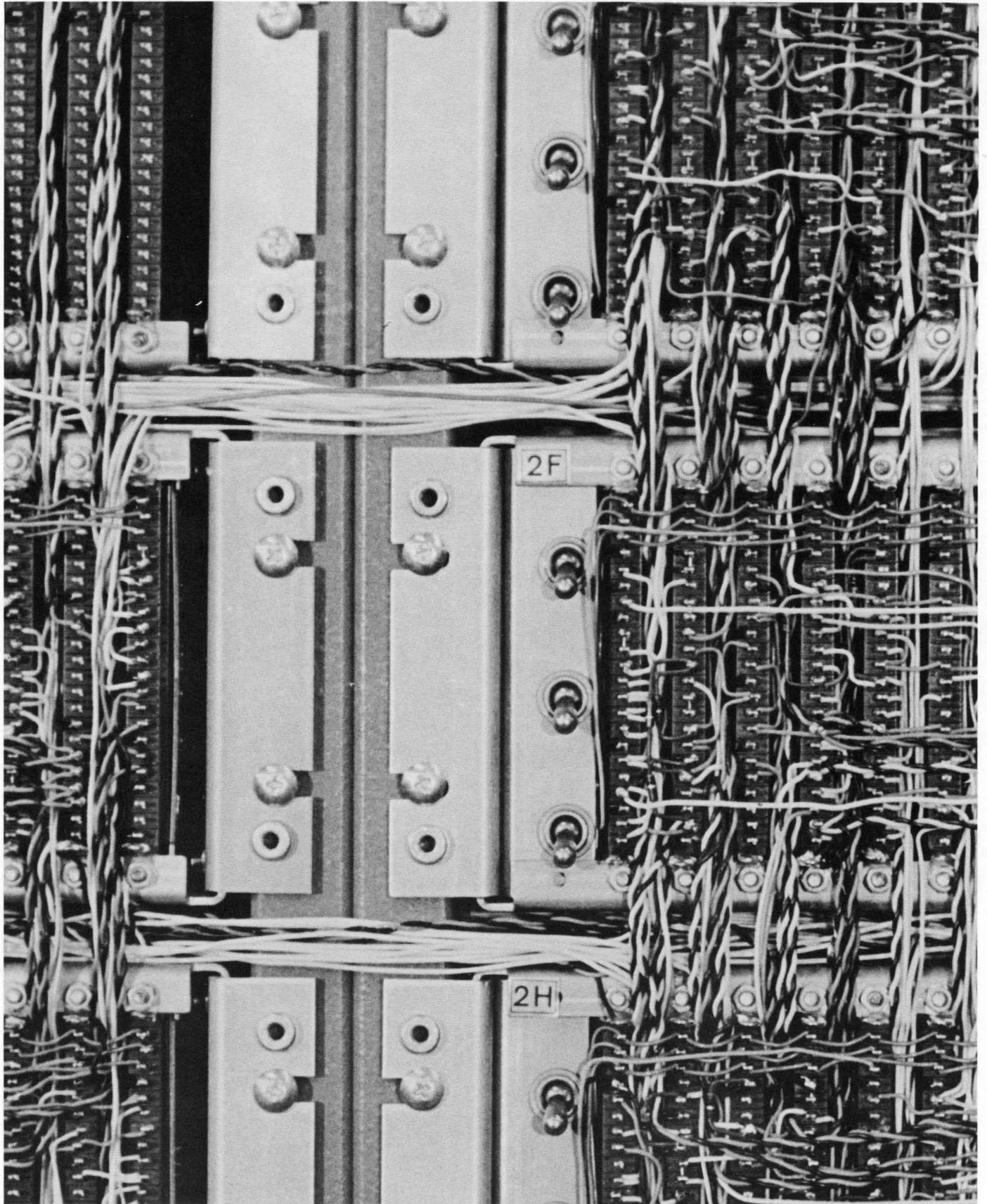
Figure 5-6 Marginal Check Toggle Switches on Mounting Panel
