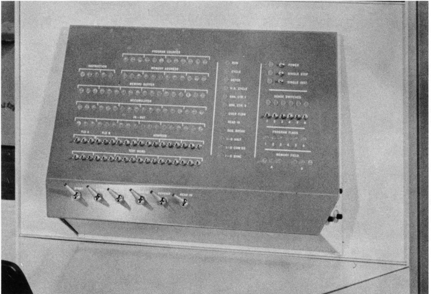
Figure 5-2 Operator Control Panel, Front and Side Views
