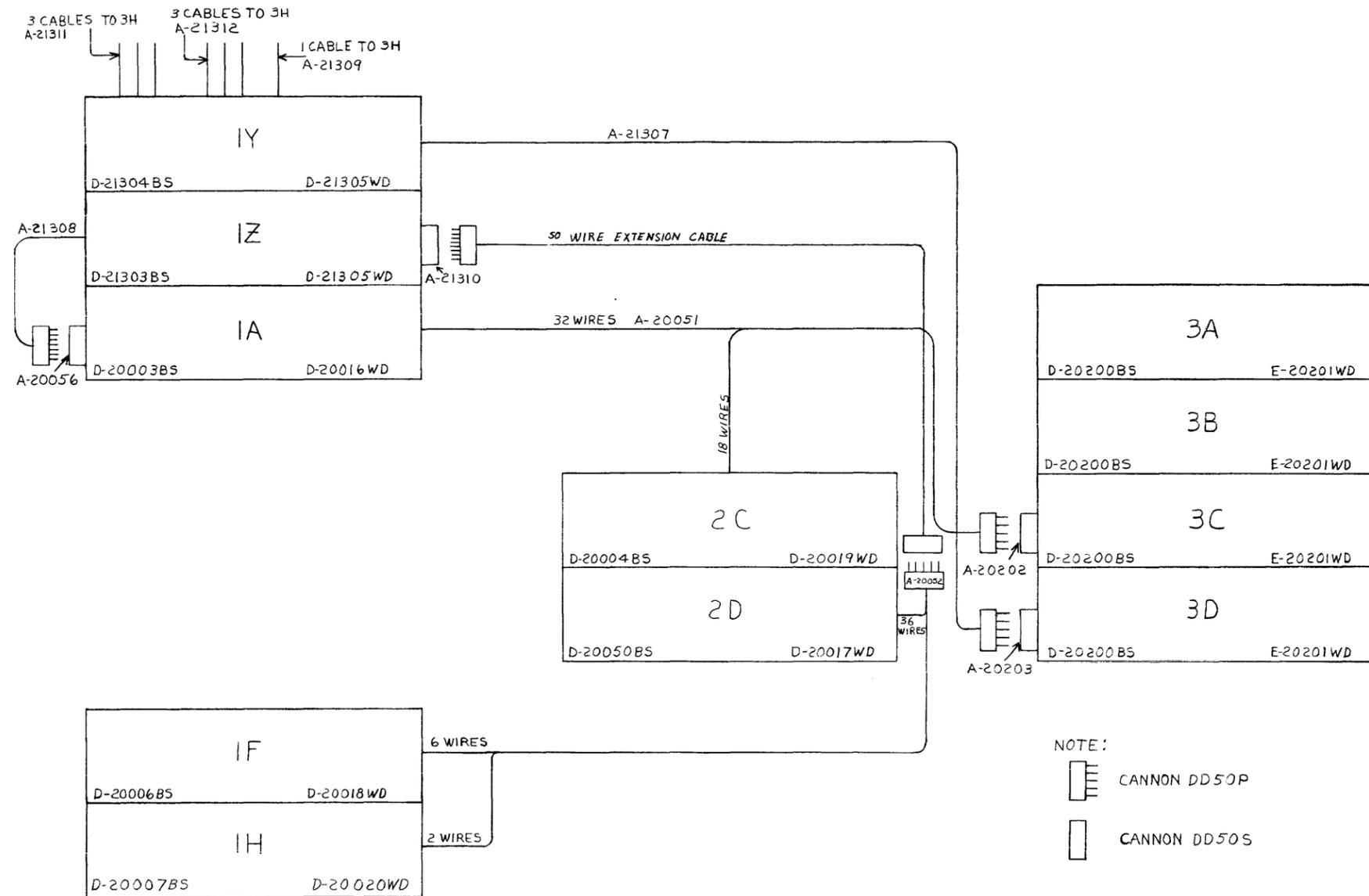
Figure 11-6 Wiring Configuration for High-speed Channel Type 19
