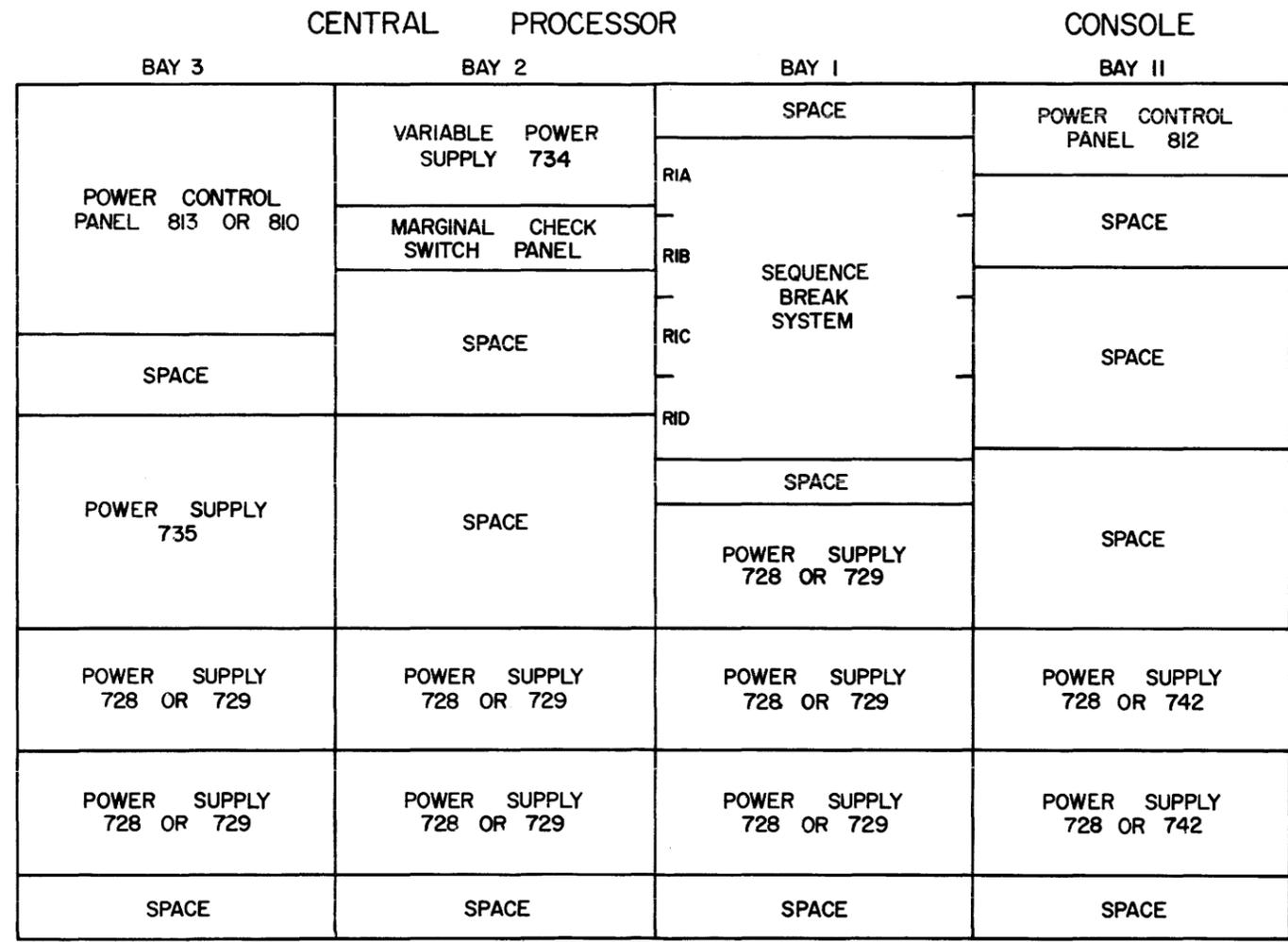
NOTE: IF NO SEQUENCE BREAK SYSTEM REPLACE RIA TO RID WITH BLANK PANELS
