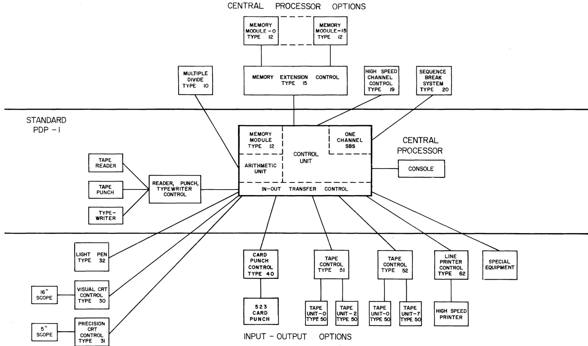
Figure 2-1 PDP-1 System Configuration Diagram
