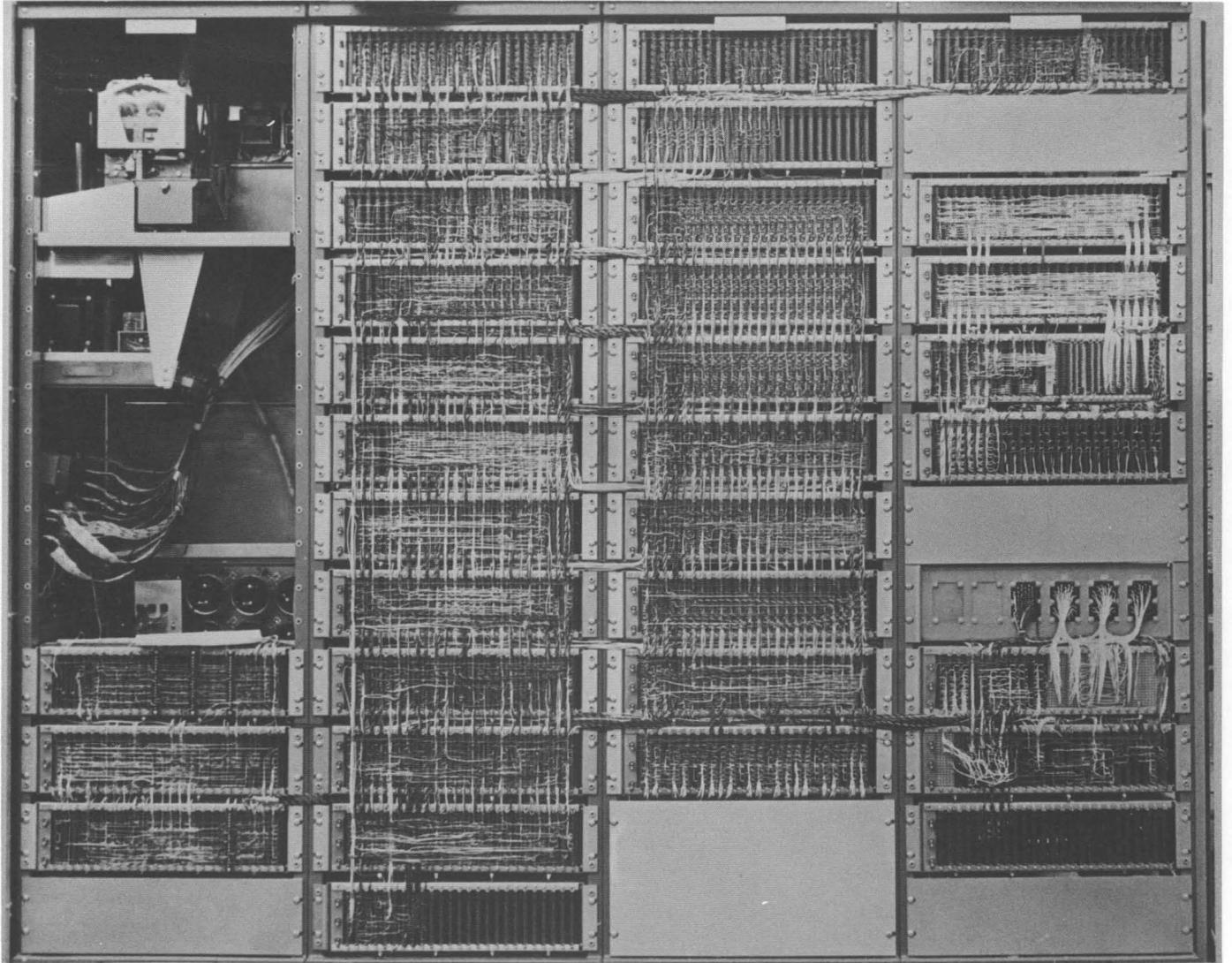
Figure 2-3 Central Frame Logic Panels
