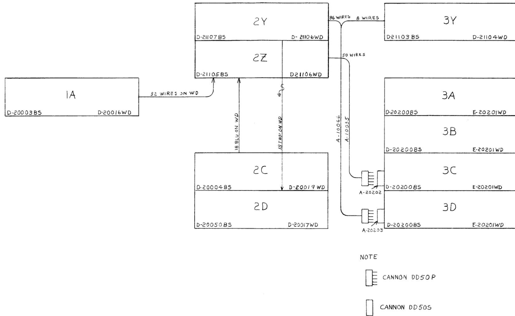
Figure 11-5 Wiring Configuration for Memory Extension Type 15
