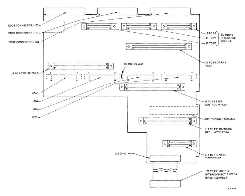
Figure 5-4 Interconnect D1 PCBA; Front View
