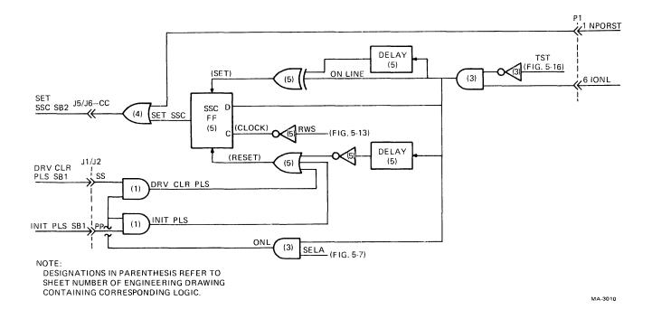
Figure 5-14 Slave Status Change Block Diagram
