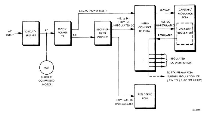
Figure 5-17 Power Supply Simplified Block Diagram
