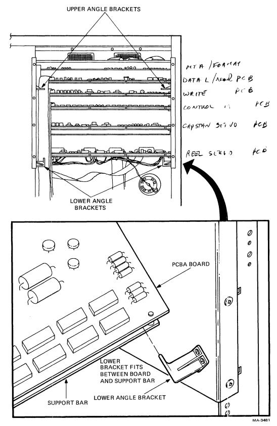
Figure 6-20 PCBA in Extended Position
