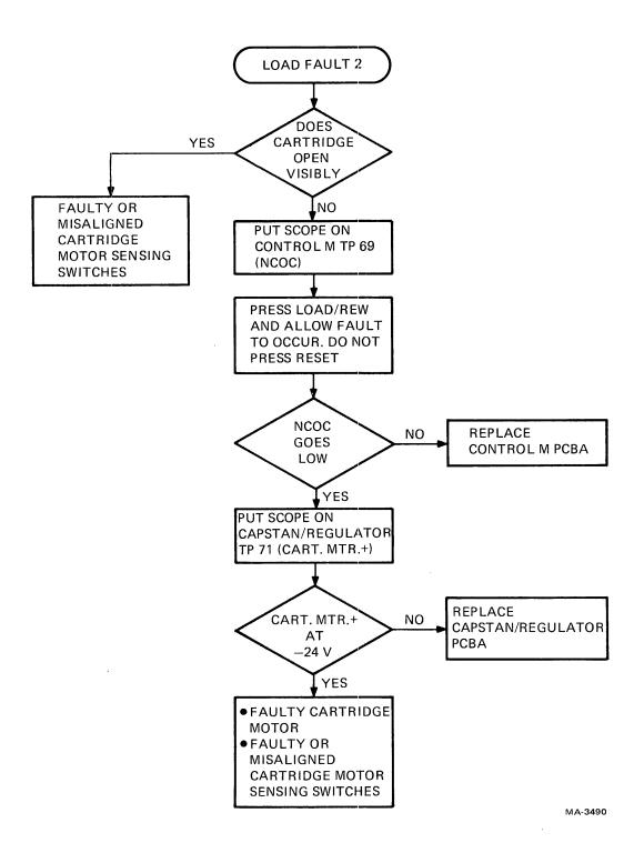
Figure 6-24 Load Fault 2 Flow Diagram
