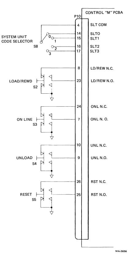
Figure 5-24 Manual Control Switching
