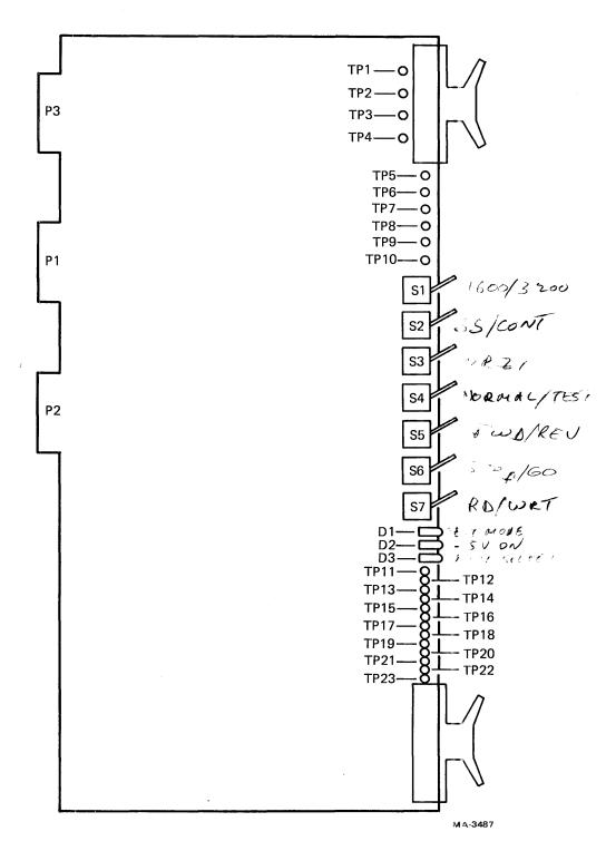
Figure 6-18 M8940 MTA Switches and Test Points
