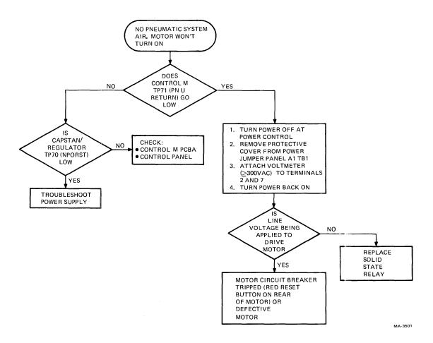
Figure 6-29 Pneumatic Troubleshooting Flow Diagram
