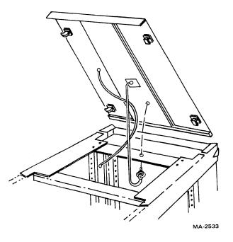
Figure 2-10 Top Cover Fastener
