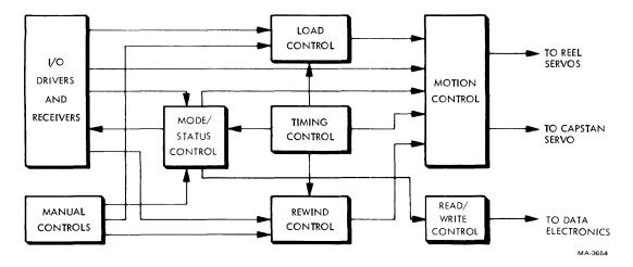
Figure 5-22 Control Logic Block Diagram
