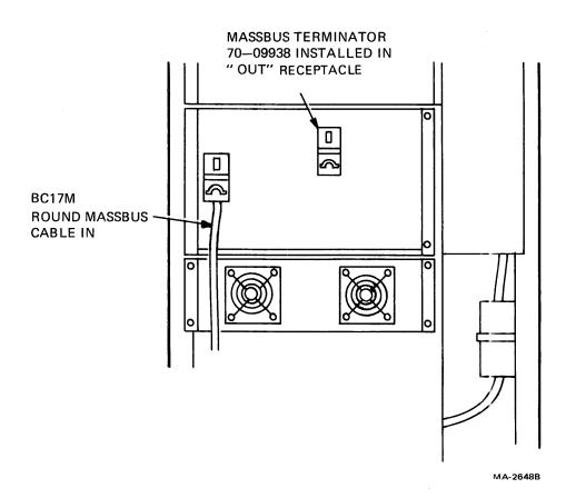
Figure 2-9 Massbus Connection to TU77 Master Transport
