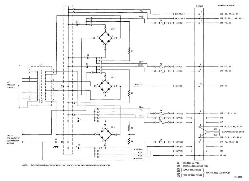
Figure 5-20 Unregulated Power Distribution Circuits
