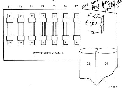
Figure 6-1 Power Supply Fuse Panel
