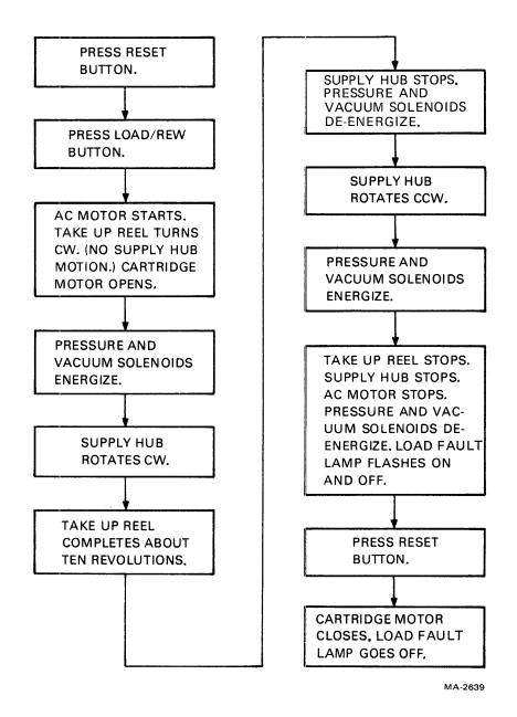
Figure 2-15 Load Sequence Without Tape
