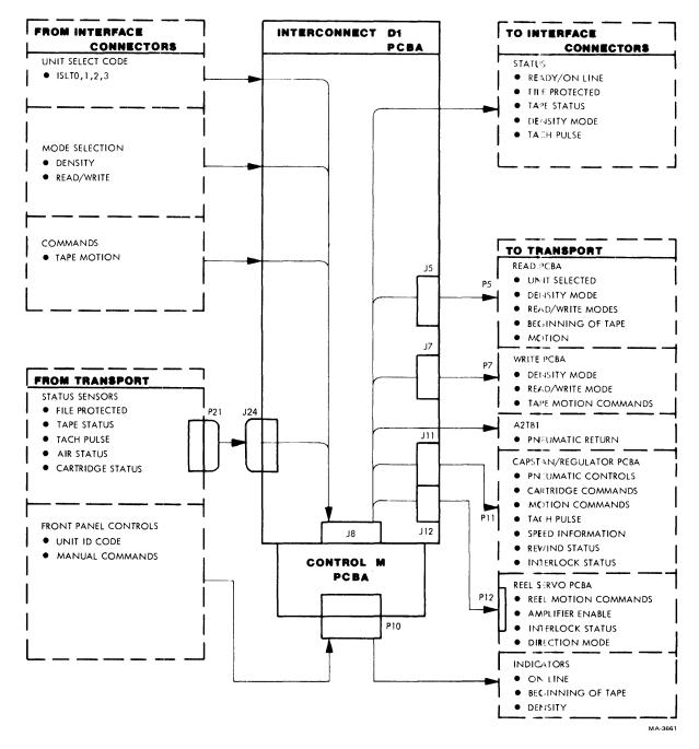
Figure 5-23 Control Signal General Routing
