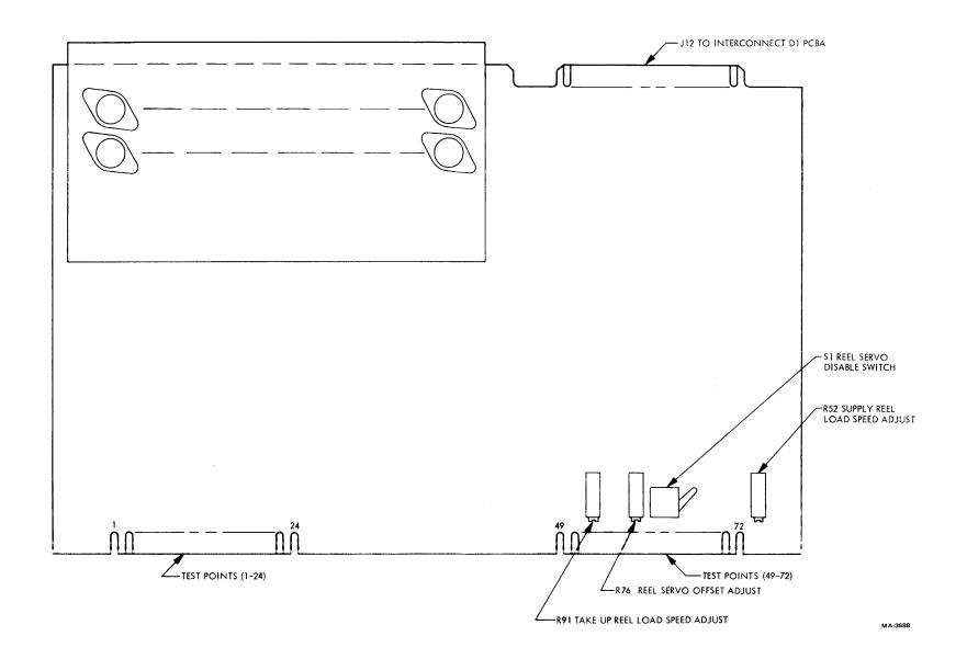
Figure 6-12 Reel Servo PCBA Adjustments and Test Points
