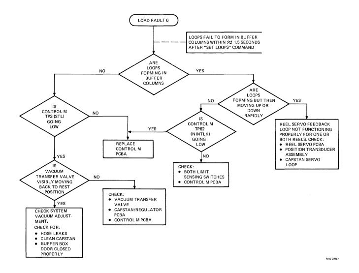
Figure 6-28 Load Fault 6 Flow Diagram
