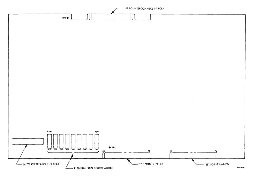
Figure 6-17 Write PCBA Adjustments and Test Points
