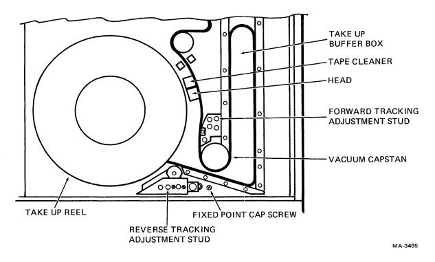
Figure 6-37 Capstan Tape Tracking Adjustment Studs
