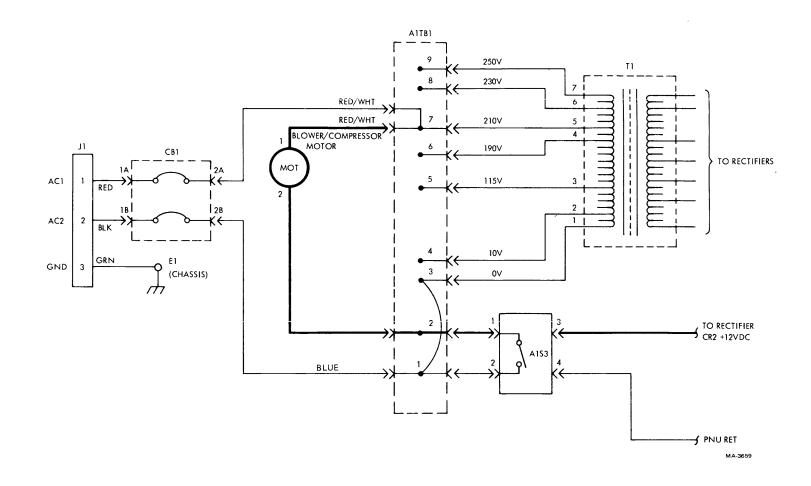
Figure 5-19 Blower/Compressor Motor Power and Control
