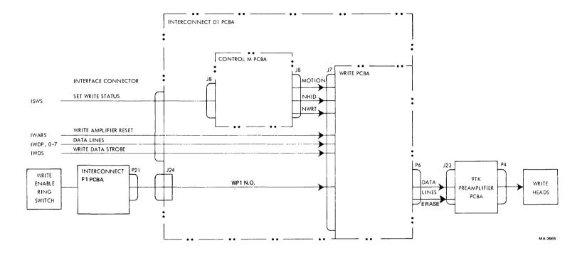
Figure 5-34 Write Function Block Diagram
