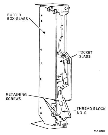
Figure 6-36 Floating Thread Block No. 9
