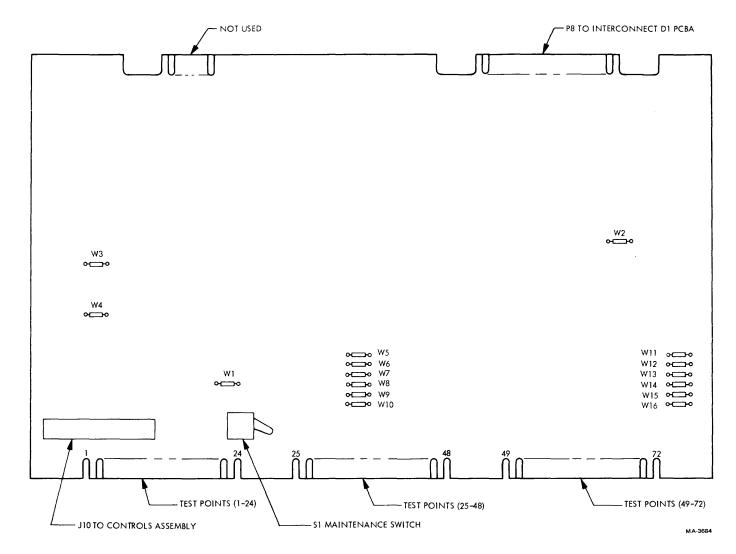
Figure 6-5 Control M PCBA Adjustments and Test Points
