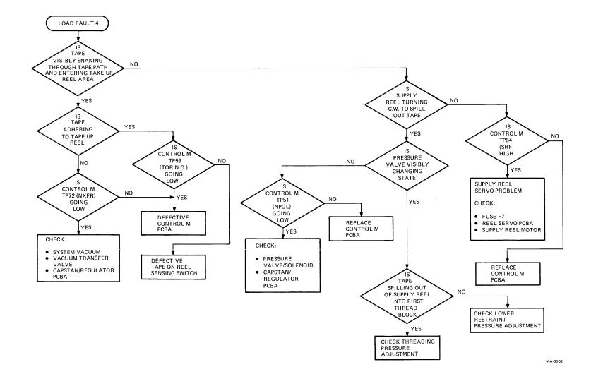
Figure 6-26 Load Fault 4 Flow Diagram
