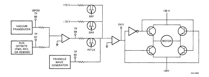
Figure 6-30 Supply Reel Simplified Schematic Diagram
