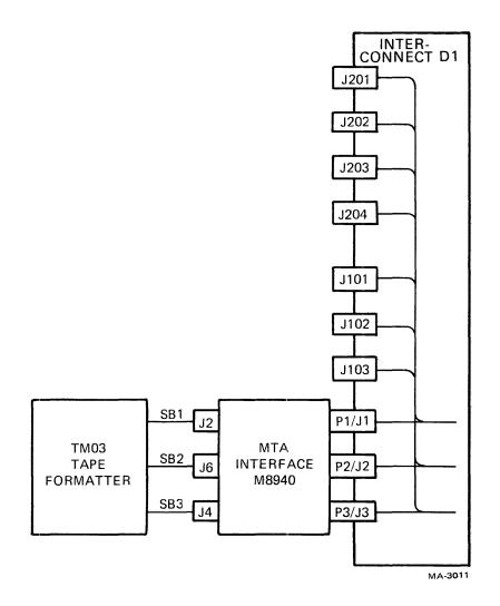
Figure 5-3 TU77 Interface Connections
