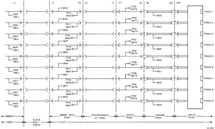
Figure 6-31 Write Data Path Test Points
