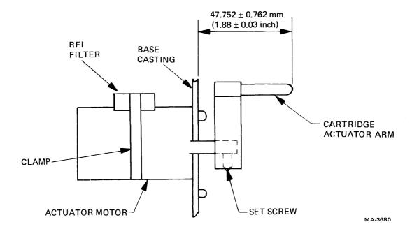
Figure 6-38 Cartridge Actuator Motor
