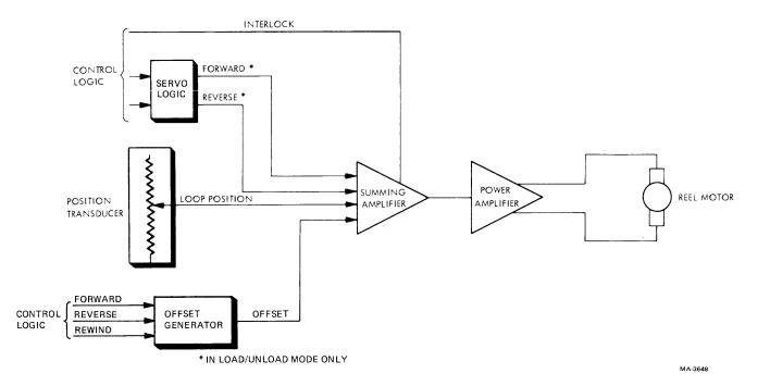
Figure 5-29 Reel Servo Block Diagram
