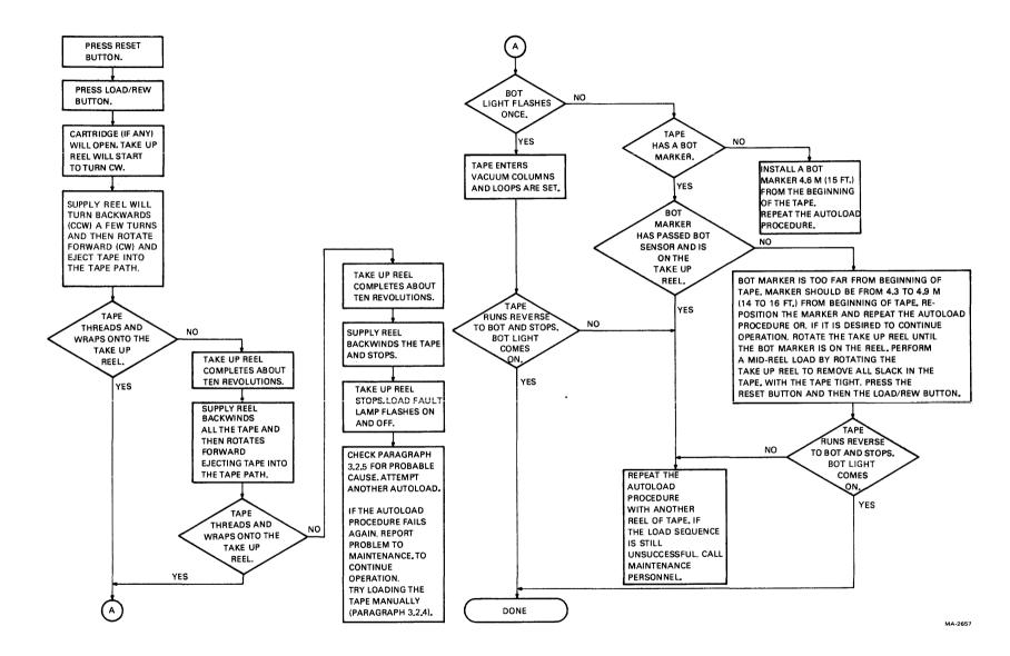
Figure 3-4 Autoload Sequence with Operator Troubleshooting
