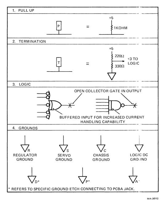
Figure 5-2 Schematic Diagram Symbology
