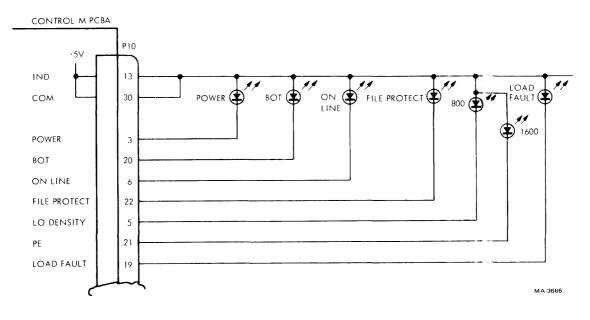
Figure 5-25 Front Panel Indicator Connections
