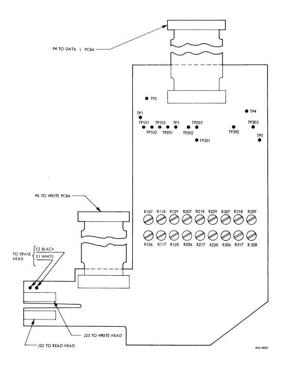
Figure 6-14 9TK Preamplifier PCBA Adjustments and Test Points
