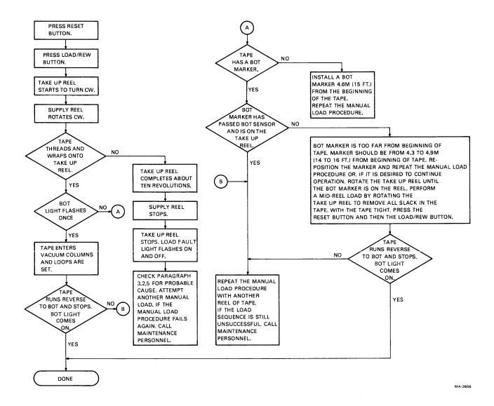
Figure 3-6 Manual Load Sequence with Operator Troubleshooting
