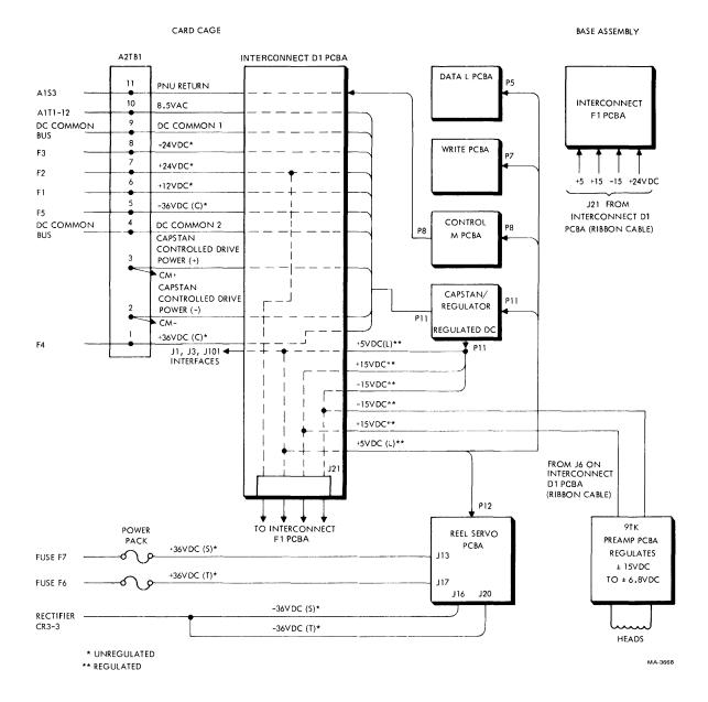
Figure 5-21 DC Power Regulation and Distribution
