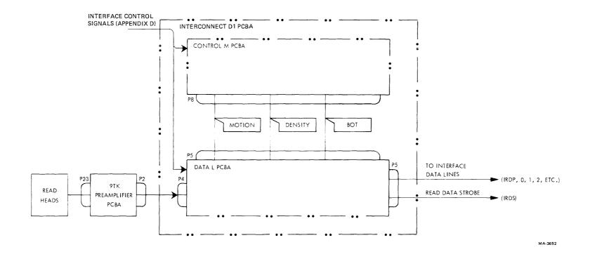
Figure 5-37 Read Function Block Diagram
