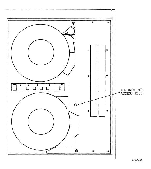
Figure 6-15 Location of NRZI Read Skew Azimuth Adjustment
