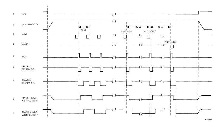
Figure 5-36 NRZI Data Recording Waveforms
