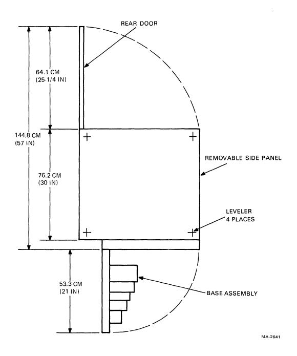
Figure 2-1 Space and Service Clearance, Top View
