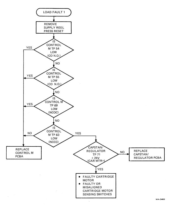
Figure 6-23 Load Fault 1 Flow Diagram
