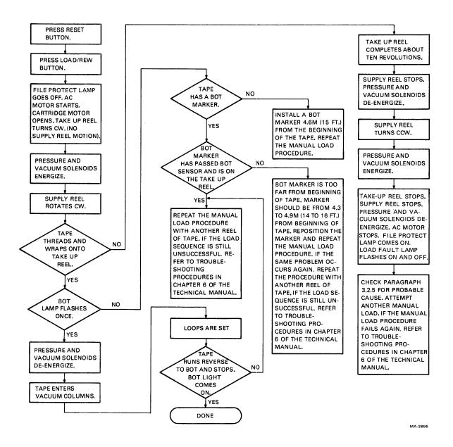
Figure 2-18 Manual Load Sequence
