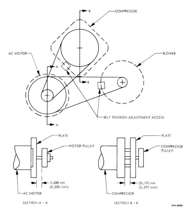
Figure 6-39 Blower and Compressor Pulley Alignment
