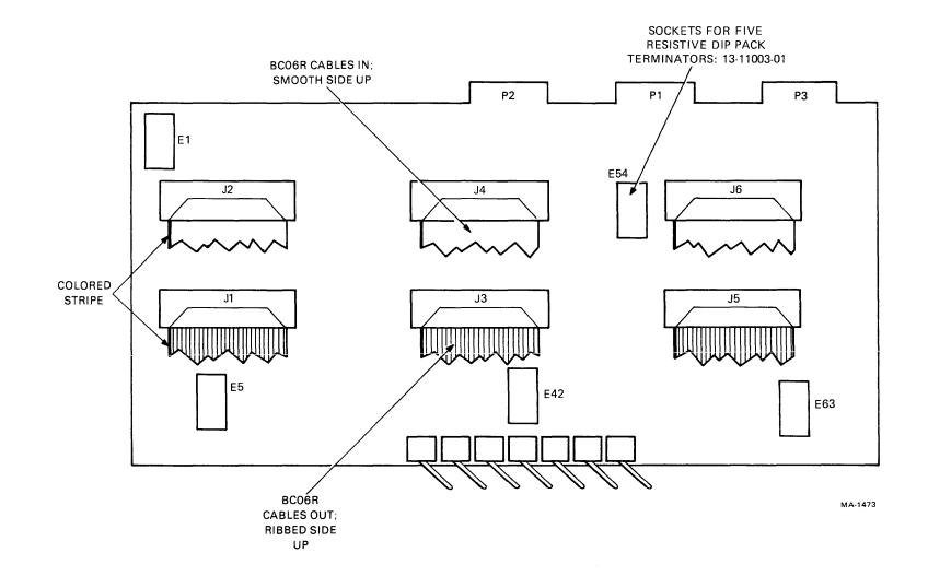
Figure 2-13 Cable Orientation on M8940 MTA Module
