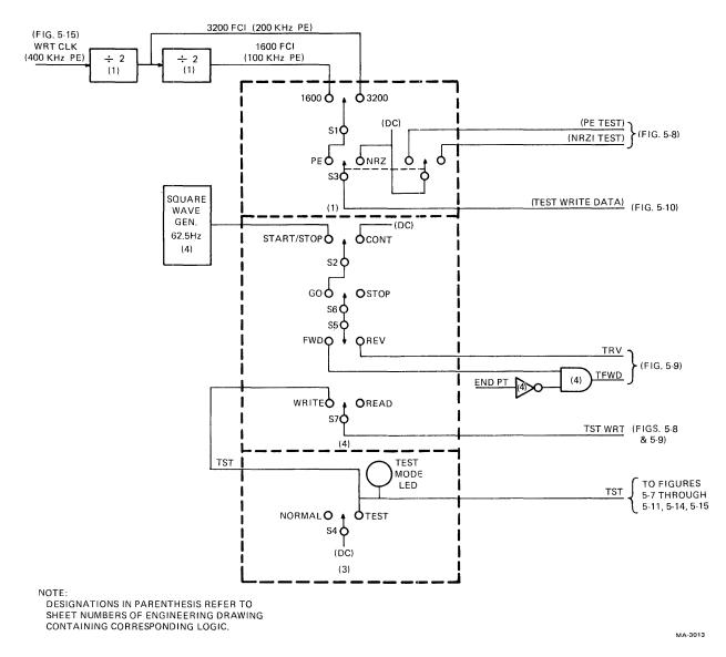
Figure 5-16 Test Logic Block Diagram
