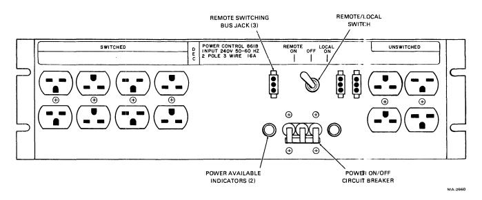
Figure 2-7 861B Power Control Panel
