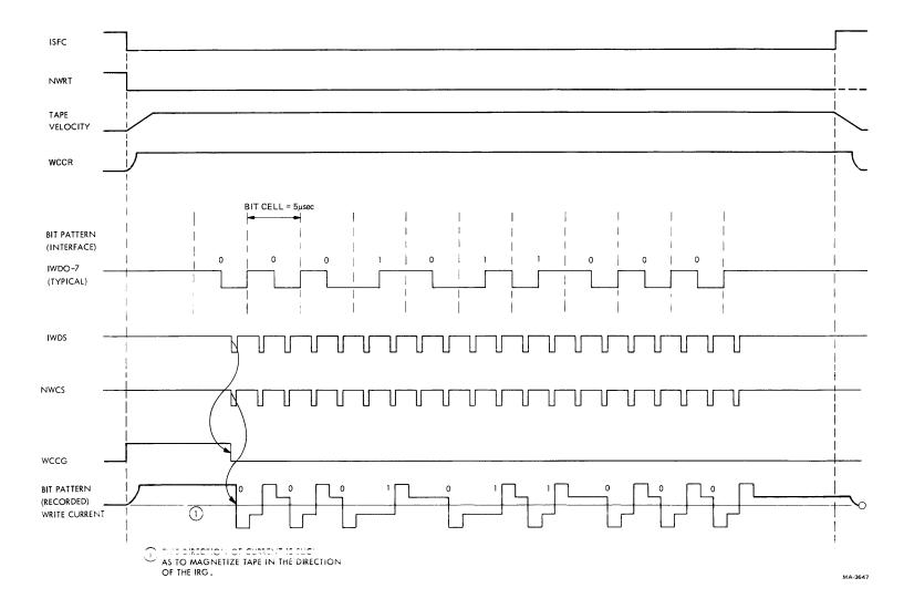
Figure 5-35 PE Data Recording Waveforms
