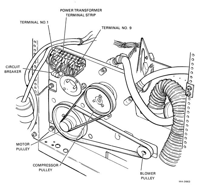
Figure 2-8 Rear of Power Pack with Pulley Cover Removed
