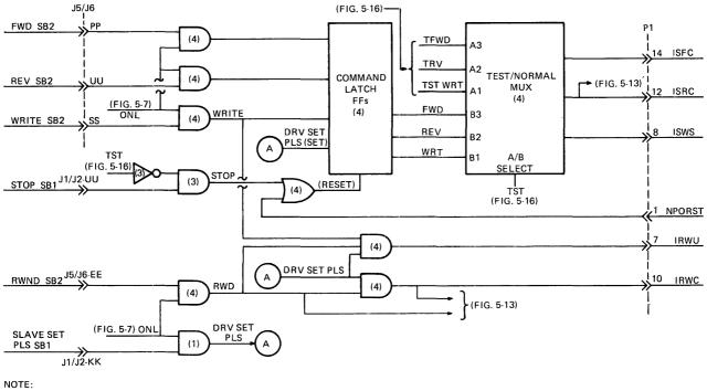
DESIGNATIONS IN PARENTHESIS REFER TO SHEET NUMBER OF ENGINEERING DRAWING CONTAINING CORRESPONDING LOGIC.
