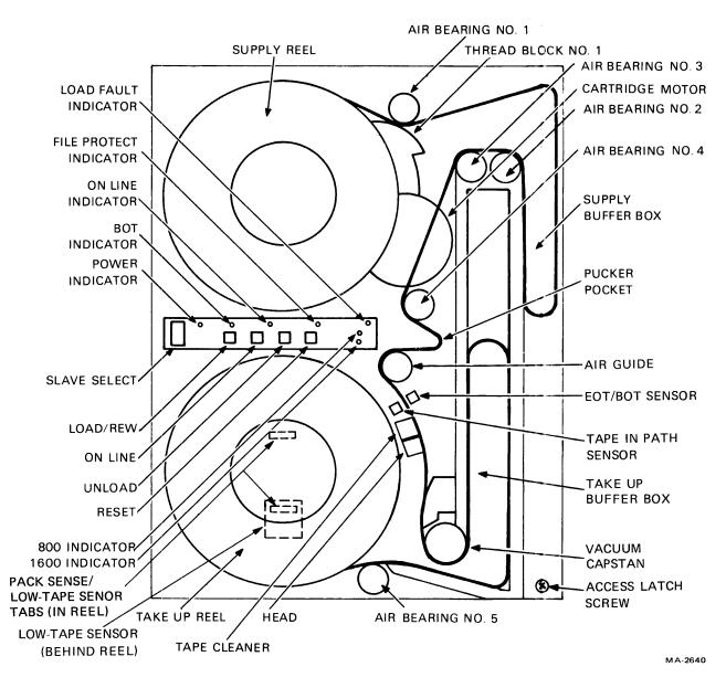
Figure 6-4 Base Assembly, Front Components
