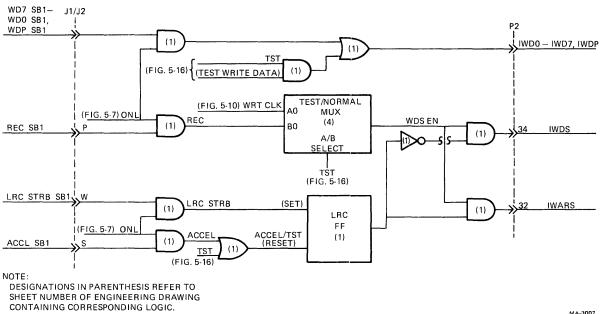
Figure 5-10 Write Block Diagram
