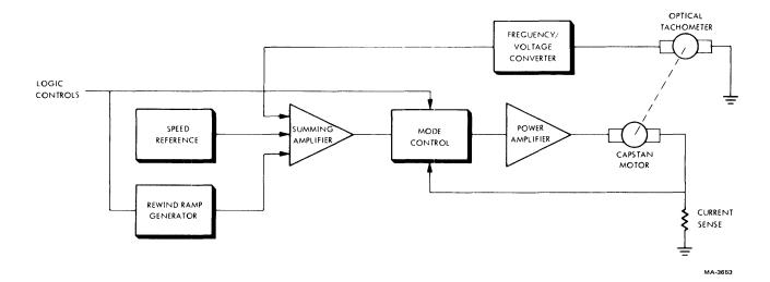
Figure 5-32 Capstan Servo Block Diagram
