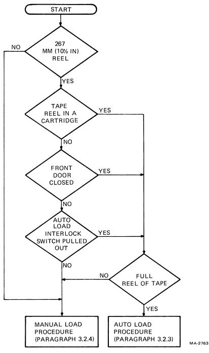
Figure 3-2 Autoload / Manual Load Selection
