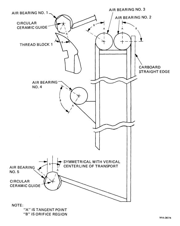
Figure 6-34 Air Bearing and Ceramic Guide Orientation
