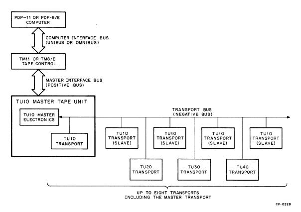
Figure 1-1 TU10 Master Tape System, Maximum Configuration
