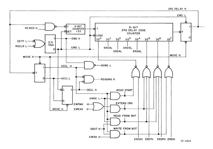
Figure 3-1 Simplified Gap Timing Logic
