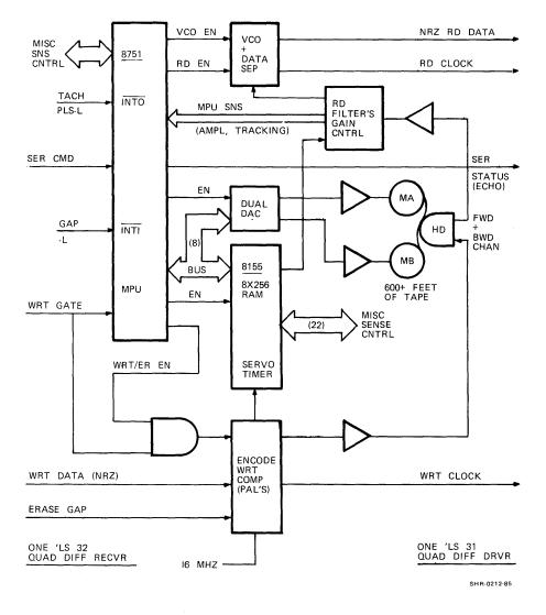
Figure 2-3 Block Diagram: Drive Board
