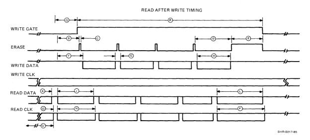
Figure 2-10 Signal Interface Timing (Q-U)
