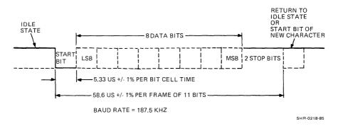
Figure 2-11 Frame Format of Data Coming from Controller
