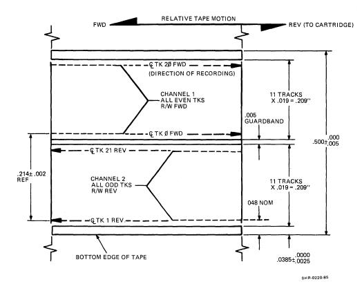
Figure 2-8 Recording Direction
