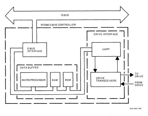
Figure 4-1 TQK50 High Level Block Diagram
