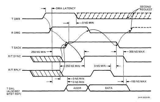
Figure 4-2 Q-bus Timing
