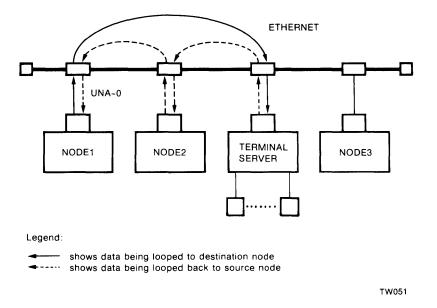
Figure 4–3: Loopback Test with an Assistant Node Giving Receive Assistance
