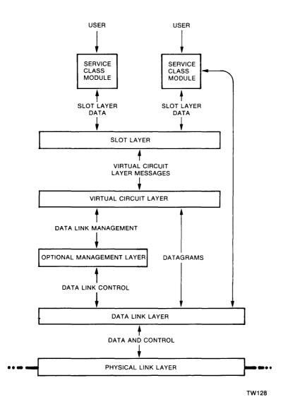
Figure 1–3: Layers in a LAT Network
