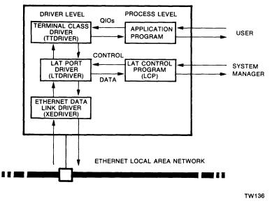
Figure 2–1: LAT Terminal Driver Control on a Service Node (VAX/VMS)
